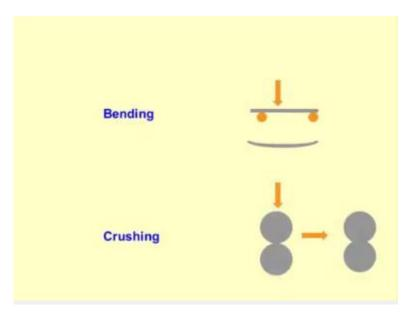
So, this is the deformed form of the plate clear, so one of the ways to deformation of the geomaterials would be the bending, the second one is crushing I hope you understand what the crushing is, two particles are sitting close to each other, and if I apply further stress and the stresses are higher than the crushing strength of the particle what is going to happen, this is what will happen, assimilation of the particles.
