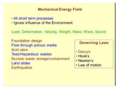
A little bit more discussion on the mechanical energy field, these are all short term processes, ignored the influence of the environment, some of the examples of mechanical energy field systems could be loading, deformation, velocity, weight, mass, waves and sound and where do you use them; in all these instances; foundation design, flow through porous media, acid rains, dissolution has occurred.
