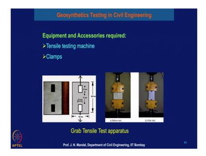
You can here the tensile testing machine and this is the clamp and this is the geotextile material and this geotextile material is before the test and this is the grab tensile test after the test. So, initially this is geotextile and this geotextile is grab with this.
