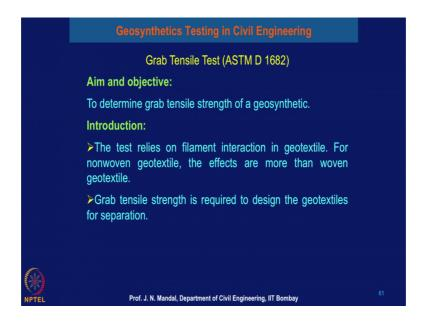
Now, I will discuss the grab tensile test. So, grab tensile test is performed as per ASTM D 1682. The main objective of this test to determine the grab tensile strength of geosynthetics material, an introduction the test rely on filament interaction in geotextile for nonwoven geotextile material the effect are more than the woven geotextile material and grab strength is required to design the geotextile for separation, you know what is the separation.
