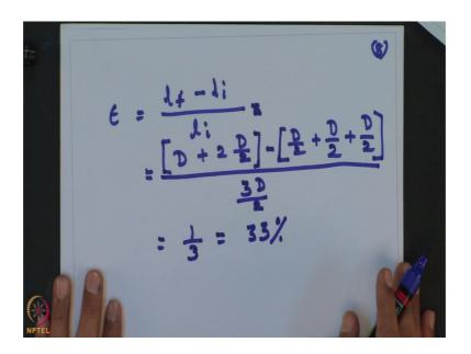
So, final length you know that is that here that is D plus 2 D by 2. So, this is the final length you know D to D by 2. This minus the initial length initial length was you know li is equal to D by 2, D by 2, D by 2. So, you can write initial length is D by 2 plus D by 2 plus D by 2 and this divided by the initial length mean you can write 3 of D by 2.
