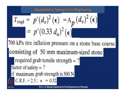
Here you know d v means, 0.33 times d a. So, this into 0.33 d a this whole square into epsilon. So, let us say given tire of 700 kilo Pascal tire inflation pressure, on the stone base crushed and 50 millimeter diameter of the, 50 millimeter diameter of the stone. So, size is 50 millimeter.
