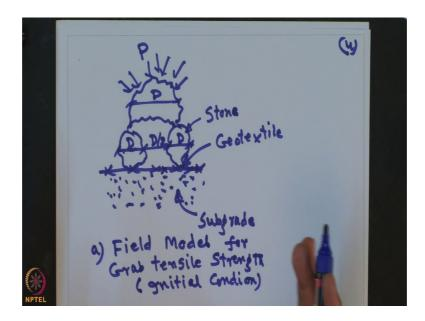
So, this is geotextile material, and these are the sub grade, these are sub grade. And these are the stone these are also a stone and this diameter of the stone let us say this is D by 2 and this distance is D, this distance is D and the top of this there is a another stone material and with diameter let us say D, and this is the pressure is acting on this that is designated at P.
