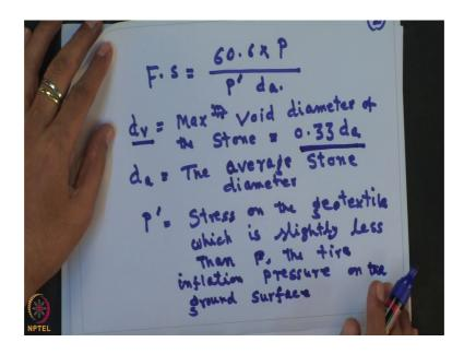
I am giving another example you know that let us say factor of safety is equal to 60.6 into P this divided by, let us say that stone on the geotextile let us say this is P dash into d of a. So, you know that dba has a relationship with the d of a. So, I am telling about what is d v I will explain this one later on that is maximum void diameter of the stone, this will be equal to 0.33 d of a, where d of a is the average stone diameter, average stone diameter.
