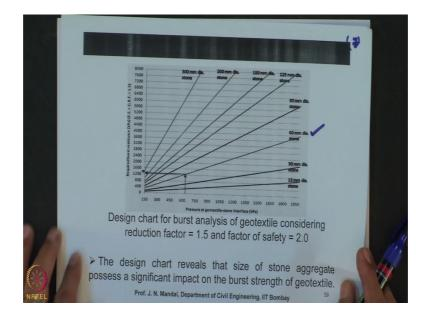
You can see here that pressure geotextile stone aggregate in the problem it is given 650 kilo Pascal this is 650 kilo Pascal, and stone diameter is 60 millimeter we can see considering this as a stone diameter 60 millimeter. So, knowing the pressure on the geotextile 650 stone diameter 60, so you can determine what should be the required burst resistance.
