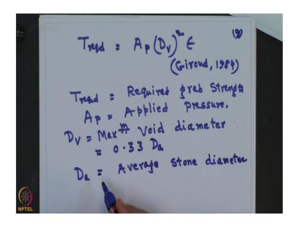
So, this is given by ground in 1984. So, where T require t require is equal to required grab strength required grab strength and A of p, this A p is applied pressure, A p is applied pressure and this is D of v, this D v maximum void diameter. So, this is maximum void diameter maximum void diameter. So, this will be equal to 0.33 times of D of a, where D of a is equal to average stone diameter this is average stone diameter, D a is equal to average stone diameter.
