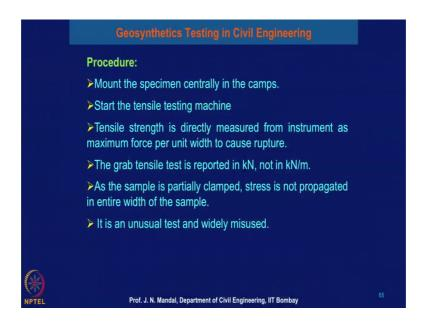
The tensile strength is directly measure from instrument as maximum force per unit width to cause the rapture. So, grab tensile strength is reported at kilo Newton, not as a kilo Newton per meter. I the sample is partially clamp the stress is not propagated in the entire width of the sample. So, it is unusual test and widely misused.
