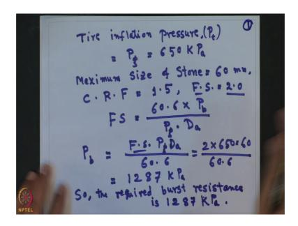
Let us say that tire inflation pressure that is P of t is equal to P of g is equal to 650 kilo Pascal, and maximum size of stone size of stone is equal to 60 millimeter. Then cumulative reduction factor is equal to 1.5 and factor of safety let us say 2.0. So, you know the equation factor of safety is equal to 60.6 into P of b this divided by P of g into D of a.
