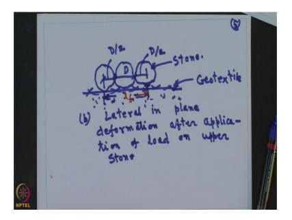
So, so if this is the geotextile material, this is geotextile and you know after applying the load and this is D this person is D by 2 and this person is D by 2. So, this is the stone and this is geotextile material, and this is sub grade. So, when you load applied in the initial stage and then there will be a lateral, lateral in plane deformation lateral in plane deformation after application of load on upper stone upper stone.
