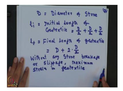
So, initial length, initial length of geotextile is equal to D by 2 plus D by 2 plus D by 2. So, if you can look here that initial length D by 2 and this is D by 2 and this is D by 2 so; that means, 3 D, D by 2. And after applying load that final length of geotextile will be equal to D plus 2 to D by 2. So, if you can see that after that final that when you apply
