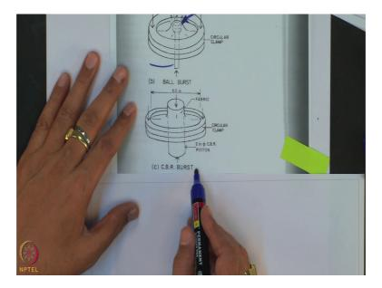
Then another type of geosynthetics material which you call the C.B.R. C.B.R burst. So, this is the same what I mentioned this is the circular clamp and this is the 2 inch diameter C.B.R piston and this piston is applied on the top of the geotextile material geotextile material here would diameter about of this model is 16 and this way also you can determine what should be the burst strength of the geosynthetics material.
