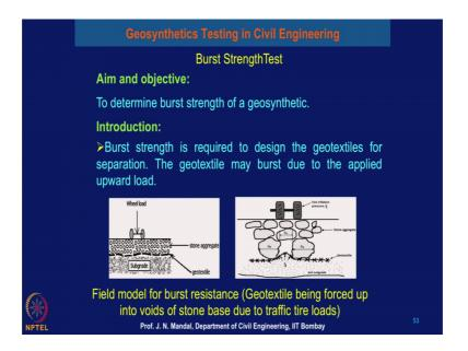
Now, we will perform the burst strength test. So, main objective of this test to determine what will be the burst strength of a geosynthetic material and burst strength is required to design the geosynthetics for separation. The geotextile may burst due to the applied upward load.
