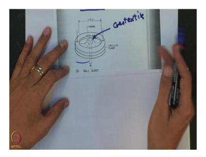
Then second another type of the test that what is called the ball burst. So, this is the kind of circular clamp and this looks like a ball the geotextile or the geomembrane material is clamped and this diameter about 1.75 inch. And, this is the geotextile material, this is geotextile material, this is a circular clamp and then ball burst and you determine what will be the burst strength of the geosynthetics material.
