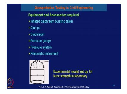
So, now what are the type of the equipment and accessory required for this test? So, you required the inflated diaphragm of the bursting tester, you require clamp and diaphragm, you require pressure gauge pressure system and pneumatic instrumentation. So, this is a kind of experimental model I can just show you.
