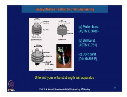
So, here also the that some also the similar type equipment has been shown here, what I shown you also this and this is the C.B.R burst strength, this is the Mullen busrt strength as for ASTM D 3786 that is this one Mullen burst strength and this is the ball burst which is as for ASTM D 751 and this is the C.B.R burst strength which we have developed in our laboratory and C.B.R burst is as for the DIN 54307. So, this is different types of the burst strength test apparatus.
