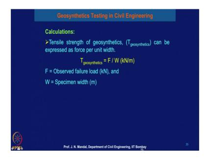
So, you have to calculate the tensile strength of the geosynthetic material and it can be expressed force per unit area that means you know what will be the object failure load and what to do the width of the specimen. So, you can calculate the tensile strength of the geosynthetic material.
