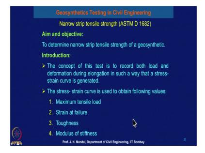
Narrow strip tensile test as for ASTM D 1682. The main aim and objective of this test to determine narrow strip tensile strength of a geosynthetic material. In introduction the concept of this test is to record both load and the deformation during elongation in such a
