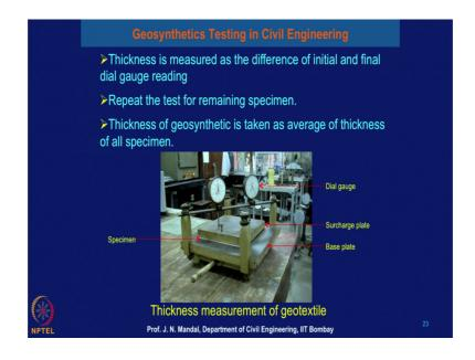
Here, is the equipment what you measure the thickness of the geotextile material. And thickness is measured as a different of initial and final dial gauge reading there here is a dial gauge you can say 2, also the 4 and you take the reading by the dial reading in the initial and the final stage due to application of the load and repeat the test for the remaining specimen. So, thickness of the geosynthetic material is taken as a average of the thickness of all specimen.
