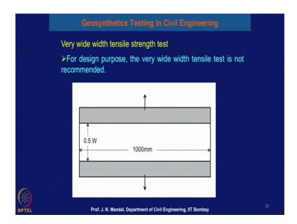
So, next is the very wide width tensile strength. So, here the size of the specimen is 1000 millimeter to 0.5 times of the W. For design purpose the very wide width tensile strength is not recommended, and generally this we do not perform any kind of the test for the wide width tensile test.
