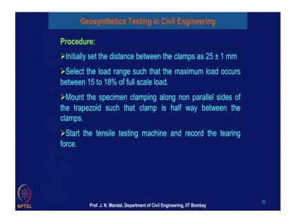
So, procedure initially said the distance between that clamp as 25 plus minus 1 millimeter select the load range such that maximum load occurs between 15 to 80 percent, 18 percent of the full scale load mount the specimen clamping along non parallel side of the trapezoid such that clamp is half way between the clamps. Start the tensile testing machine and record the tearing force.
