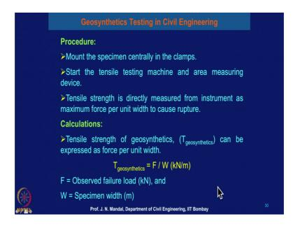
Now, procedure for first mount the specimen centrally in the clamp start the tensile testing machine and area measuring device tensile strength is directly measured from the instrument and maximum force per unit width to cause rapture.
