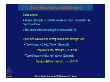
So, how to calculate the tensile strength, cafeteria trapezoidal tensile strength of the geosynthetic material? Tensile strength is directly measured from the instrument as a
