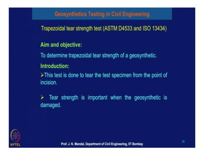
Next you know geosynthetic material may tear. So, we have to perform some kind of the test and which is called the trapezoidal tear test strength. When you dump these any kind of the material or gravel on to the top of the geosynthetic material, geosynthetic material
