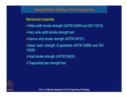
Next is the mechanical properties which is very important in civil engineering and how to perform the different types of the mechanical properties of the geosynthetics material. There are various types of the test are available.
