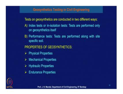
A index test or in-isolation test, test are performed only on geosynthetics itself, and B performance test, test are performed along with the site specific soil. If we can perform the geosynthetics material along with the site specific soil you can obtain some different value with respect to index tests or in isolation test. It is true that if you perform some time some of the test with the site specific soil then you can have much more realistic value.
