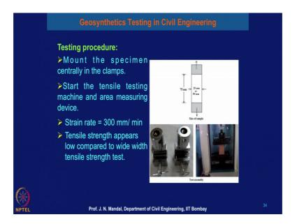
So, tensile strength appear low compared to wide width the tensile test. So, this you can this, this is the clamp and this is a part from the narrow tensile test.
