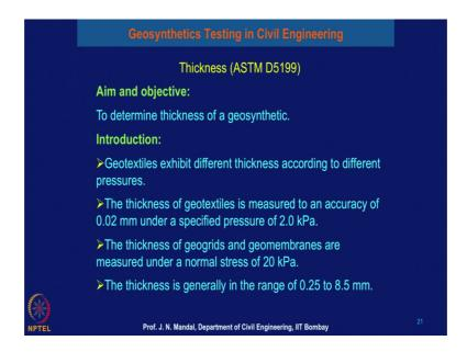
Now, next here to determine what will be the thickness of the geosynthetics material it varies thickness of the geotextile material it may be 0.25 or it may be 3 millimeter, 5 millimeter, 4 millimeter, 4.55 millimeter, 8 millimeter. So, different types of the thickness of the geosynthetic material will be available for particularly for woven and non woven geotextile material and this various application.
