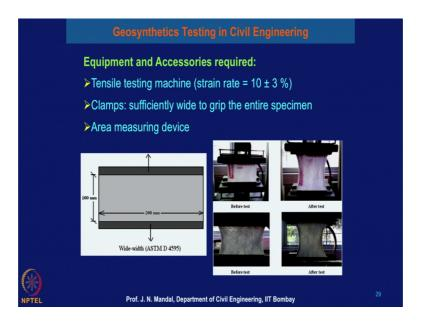
The strain rate for the wide width tensile strain will be 10 plus minus 3 percentage. If it is a ISO specification or international standard organization specification the tensile strain machine rate will be 20 plus minus 3 percentage, so strain rate is very important.
