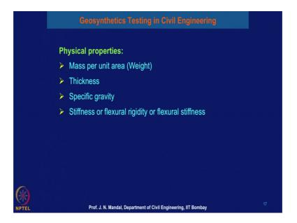
Second what will be the thickness of the geosynthetic material, what is the specific gravity of the geosynthetic material, what will be the stiffness on flexural rigidity or flexural stiffness? So, we will discuss one by one how we can perform the defined physical properties of the geosynthetics material.
