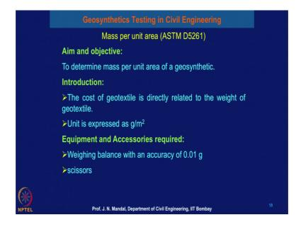
Because mass per unit area vary it may be 100 gram per meter square, 200 gram 300 gram, 400 gram per meter square, 500, 600 gram per meter square. So, if the gram per meter square is more the cost of the geosynthetic material also will be the more, but we have to select one gram per meter square geosynthetic material is required for the specific application and how you can perform the test.
