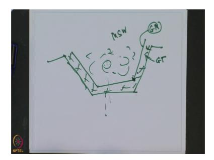
So, if you want to construct a land field like this conventional system you know, but alternative system you place the different types of the geotextile material which will act
