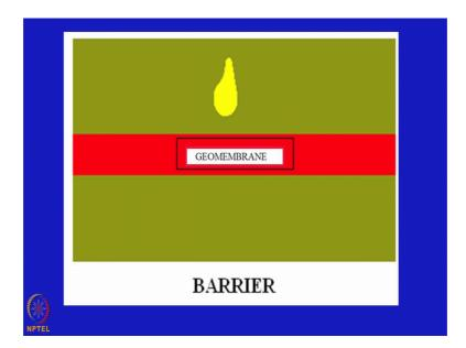
And this is geomembrane you know for the land field you can use as a barrier, that is impermeable material and it cannot be contaminated the water cannot be passes through and it can control. For example, the land fields if you want to construct a land field, so there are different types of the land field.
