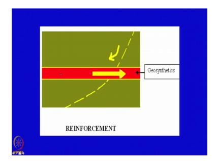
For example, this is a slope this slope can fail like this then you can place the geosynthetic material between the (Refer Time: 12:19) foundation to increase the factor of safety. So, here geosynthetic material act as a reinforcement. So, the beauty of this geosynthetics material for a particular application is not only act as a separation filtration or drainage, but also act as a reinforcement for an example that for the road construction.
