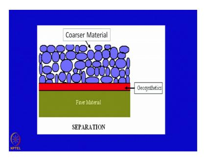
Now, I will just briefly explain what do you mean by the separation. You can see here that the rate one is the geosynthetics material. It may be woven, non woven geotextile, it may be geogrid material and top one is the coarser material and bottom one is the finer material.
