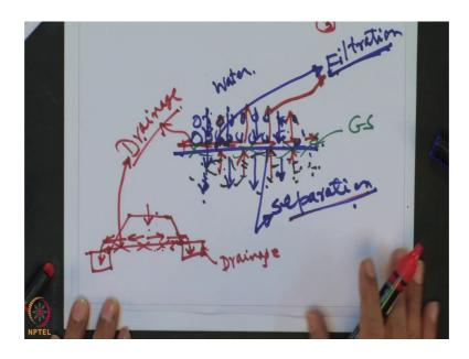
So, if this is the geosynthetics material. So, let us say this is the geosynthetics material and this is the courser material, and this is the finer material, this is the finer material. So,
