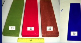
Flexural strength test specimen (Density of the geofoam material from left to right are 15, 20, 22 and 30 kg/m 3 )
