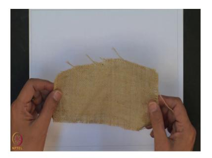
You can also develop this woven natural geotextile material. This is woven jute geotextile material. Here, you can see this filament are perpendicular to the each other. So, it is woven jute geotextile material. So, it has also the tensile strength in the machine direction and also cross machine direction and corresponding to the elongation. What? We will study.
