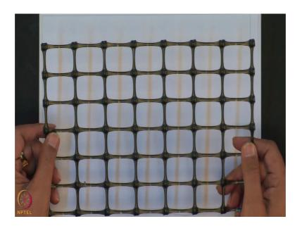
This is biaxial geogrid material this is biaxial geogrid material. So, this also can be used for the railway. It has also the tensile strength in the machine and cross machine direction and corresponding to the elongation. There are some other materials also used for the construction of the reinforce soil retaining wall.
