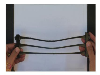
And this act as a reinforcement and you have to determine what will be the tensile strength in the machine and cross machine direction and corresponding to the elongation. And this kind of the geogrid material can be used for the for the construction of the reinforced soil retaining wall or the reinforce soil slope and also you can use for the geogrid material for the road construction and this is the uniaxial geogrid material.
