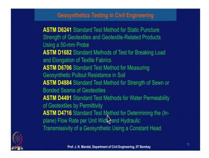
ASTM D6241 Standard Test Method for Static Puncture Strength of Geotextile related product using a 50 millimeter probe; ASTM D1682 Standard Test Method of Test Breaking Load and Elongation of the Textile Fabric. ASTM D6706, Standard Test Method for Measuring Geosynthetics Pullout Resistance in Soil.
