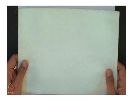
So, this filament is very random. So, you have to perform what will be the tensile strength in the machine direction as well as in the cross machine direction and what will be the elongation for both machine as well as cross machine direction. You can also perform the test in the diagonal direction. So, this is the non woven geotextile material which filament are very random.
