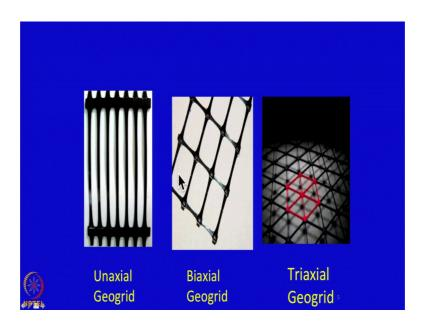
So, this geogrid material is used, this is Uniaxial Geogrid; this I showed you that Biaxial Geogrid. There are another also new material has come which we called that Triaxial Geogrid material and this Triaxial Geogrid material also is made from the bamboo and also polyester material.
