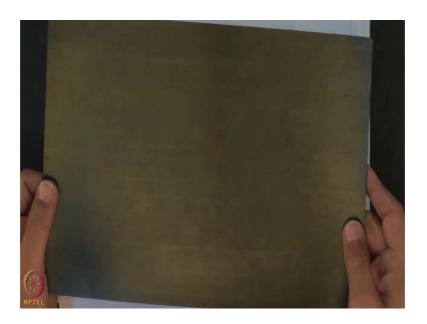
This is smooth geomembrane material. So, if we want to use in a slope of land flow and then, you sometimes require there will be the mobilization of the friction between the slope soil layer and the geomembrane and that is the why that there are some geomembrane material also develop.
