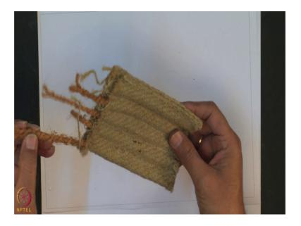
The outside is a woven and non woven jute material and quiet coconut fibre; this act as a probe of water. So, this is the jacket and this is the core material. You can use also this kind of also as a geocomposite material. This, another material which you call the Geocell.
