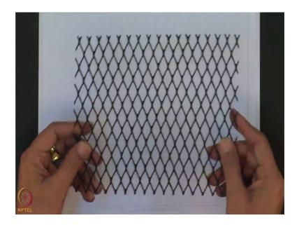
This Geonet material is used for the drainage and the filtration you can use for the Lanchow. What there is a problem with the drainage and the filtration, you can use this kind of the Geonet material.
