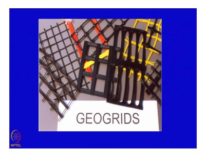
So, most of the cases that this material can use as a filtration and the (Refer Time: 14:55) material and as well as reinforcement. Next this is the geogrid material. So, these material have a uniaxial geogrid and also the biaxial geogrid uniaxial geogrid and also biaxial geogrid. This is the uniaxial geogrid ok.
