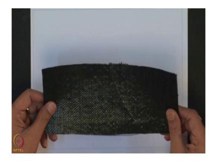
So, it is called the woven geotextile material.
