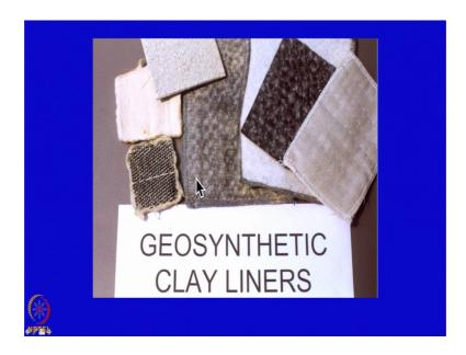
And this geosynthetic clay liner is made of geotextile, bentonite, and the geotextile. It is like a sandwich form. So, when the water will come in contact with the bentonite and it is expand and it act as a impermeable material.
