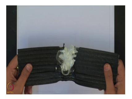
And this is what you call the friction tie. So, this kind of the material also can be used for the construction of the reinforce soil wall and it is called the friction tie. We can use some material for the reflection cracking.
