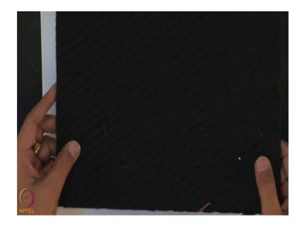
This is non woven and the Geonet material and the non woven. So, this is the geocomposite material. You can have also this is also you can say geocomposite material.
