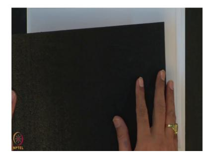
The one side of the geomembrane is very rough which can be face towards the slope of the soil because, there will be a development of the friction between the rough of the geomembrane side to the soil and the other side is a smooth.
