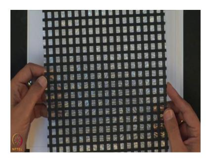
So, this the kind of the material which you can use for the reflection cracking material. It had been used also in the airfield pavement for the reflection cracking and it has strength also 100 kilo Newton per meter or 50 kilo Newton per meter. So, this is all glass polymer material.
