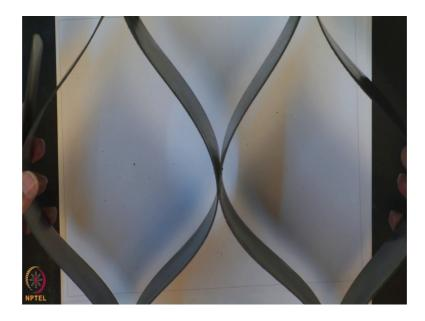
So, this Geocell or the geocell you can be claps; it can be expanded and it can be filled up with the different types of the filling material, gravel sand and place it and compact it. You can construct the road, you can use for the slope, you can use for the erosion control with a potential application of geocell material in Civil Engineering.
