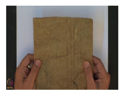
So, this is the natural non woven geotextile and this geotextile material is made from jute fibre. So, natural material also used for the as a geotextile material. So, this is the non woven natural jute geotextile material.
