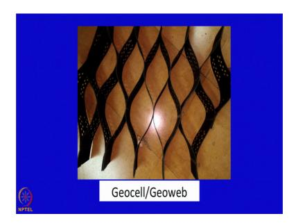
So, this the Geocell, this is the hexagonal, hexagonal; 3 dimensional hexagonal structure.
