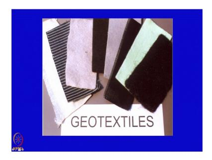
There are 2 types of the geosynthetics material; one is the woven geotextile material, another is non woven geotextile material. So, when you say it is the woven geotextile material, you can see here this geotextile material, this filament are perpendicular to each other and showing one of the woven geotextile material, this the woven geotextile material and these are the filament are perpendicular to each other.
