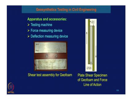
So, for this kind of the test you recall that apparatus; what kind of apparatus you want to use and how you will perform the shear between the two geofoam material? So, here I will show you that apparatus that is required testing machine and this is force measuring device and deflection measuring device.
