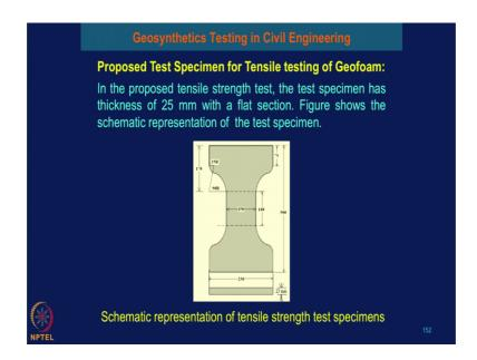
Now, we will show you that Proposed Tensile Specimen Test measurement of the tensile strength of the geofoam material and this proposed tensile strength of the geofoam material is developed by IIT Bombay and it is much more simplified than the earlier ASTM tensile strength of the EPS geofoam material. In this proposed tensile strength test, the test specimen has a thickness of about 25 millimeter with a plat section.
