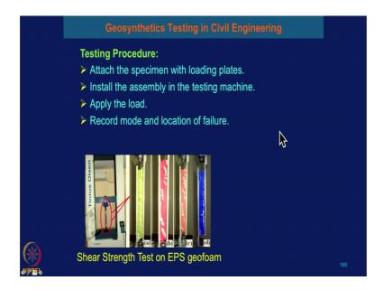
So, from this testing method, how you are attaching the sample and what will be the testing procedure that I wanted to show you. Here you can see that attach the specimen ok. This is the specimen attached with the loading, loading plate and here is the attached with the loading plate and install the assembly in the testing machine and then you can apply the load and record the mode and the location of the failure.
