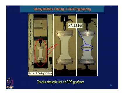
So, if you can perform the test, you can see here this is the sample and you are using the universal testing machine to perform the tensile strength of the EPS geofoam under
