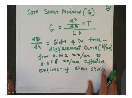
So, you can determine Core Shear Modulus which is designated as G. So, G you can write is del of P divided by del of u into t this divided by L into b. Where, del P by sorry del of P by del of u is equal to the slope of the force displacement curve. So, this is the slope of the force, force displacement curve; that is Newton per millimeter.
