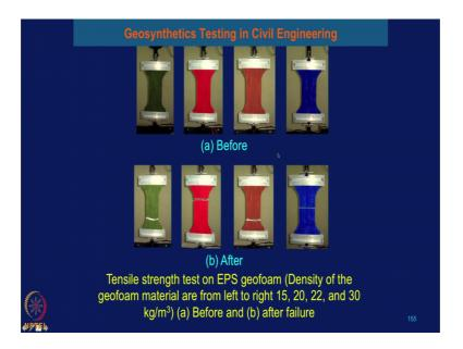
So, here tensile test strength test of EPS geofoam and as I say with density 15, 20, 22 and the 30 kg per meter cube. This is before the test. This four before the test and you can see after the test. In some sample is not at the edge some sample at the top and sometimes is at the bottom and some sample at the centre of the EPS geofoam material. So, it is preferable that sample should fail at the middle of the sample.
