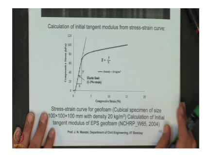
So, here I am showing this is the stress compressive stress verses compressive strain curve of a geofoam. This is the cubical specimen size is 100 millimeter into 100 millimeter of density of 20 kg per meter cube. So, here to calculate what will be the initial tangent modulus of the EPS geofoam. So, here the, this is the stress strain curve is shown and you draw a tangent here, you draw a tangent here.
