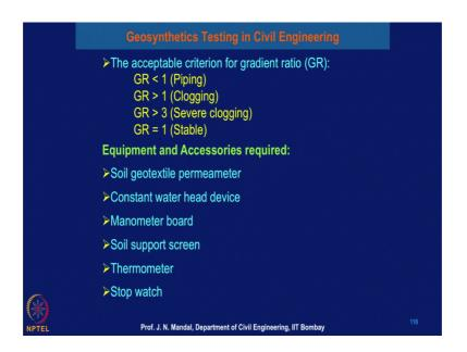
This is the acceptable criteria for gradient ratio. If gradient ratio greater than 1, you can see it is clogging. If the gradient ratio greater than 3, you can say it is a severe clogging. If the gradient ratio is 1, then you can stay stable. To perform the test you require now what will be the equipment and the accessory. So, you require Soil geotextile permeameter, Constant water head device, Manometer board, Soil supports screen, Thermometer and Stop watch.
