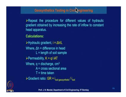
For different value of hydraulic gradient, obtained by increasing the rate of inflow to a constant head apparatus; for example that you have to calculate this gradient ratio.
