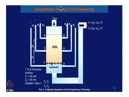
And here, you can see that these all are port and this is the soil sample geosynthe synthetic material is here and this is 1, 1 2 3 4 5 and 6. So, these are pizometer number. So, you can determine what will be the P of 1 here, here. Then, this is P 3 and this is for P 5; this is for P 6; this is for P 4 and this is for this is for P 2 ok. And this distance from here to here Z 1, which is 25 millimeter and from here to here Z 2 is about 50 millimeter.
