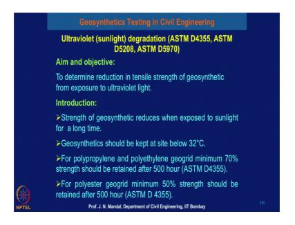
Now, strength of geo synthetics material may reduce when the expose in the sunlight for long time. So, you cannot keep the geo synthetics material for longer time in the sunlight because geo synthetics material may degrade. So, what percentage of degradation it would be?
