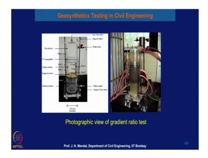
And this is the equipment already is developed in our laboratory here. This is photographic view of the gradient ratio. This is this is the gradient ratio and geosynthetics material is placed somewhere here and the soil and at a different different parts, I will show you in detail about the photometric gradient ratio of the soil sample.
