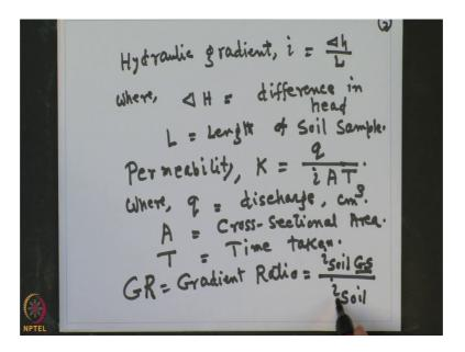
So, here I am showing you some calculation. So, hydraulic gradient, gradient that is i is equal to delta h by; where, delta of h is equal to difference in head and L is the length of the soil sample; L is the length of soil sample ok. And permeability; Permeability, K is equal to q divided by i into A into T; where, q is equal to discharge; q is equal to
