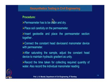
Now, what is the procedure to perform the test? So, permeameter has to be clean and dry. Place the soil carefully on the permeameter. Insert the geotextile and place the permeameter section together. Connect the constant head device and manometer device with permeameter.
