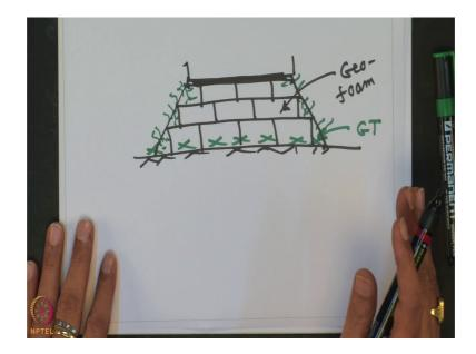
So, it was like these suppose if this is the ground surface ok. You can place the 1 layer of the geotextile material here. This is geotextile material GT and you can construct the embalmment on the very soft soil; you do not need any kind of the compaction. So, this is a block. So, this is this is the geofoam block. This is the geofoam block.
