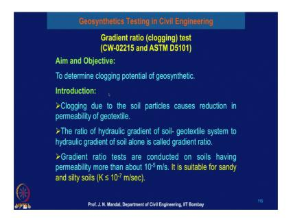
So, now I will talk about the gradient ratio. So, here the objective is to determine the clogging potential of geosynthetics. In introduction clogging due to the soil particle cause reduction in the permeability of the geosynthetics material. The ratio of hydraulic
