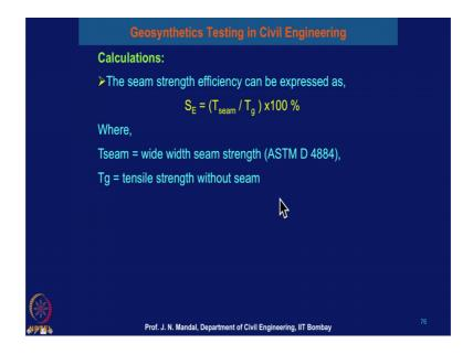
So, how to calculate the seam strength? So, seam strength can be calculated and seam strength efficiency can be expressed as S E is equal T seam divided by T g into 100 where T seam is the wide width seam strength as for ASTM D 4884.
