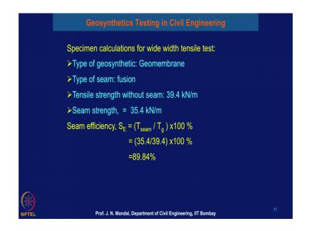
Now, specimen calculation for the wide width tensile strength let us test type of the material it may be geosynthetics or the geomembrane material. And type of the second sewn seam is may be the fusion, or tensile strength without seam is 39.4 kilo Newton per meter and which seam strength is 35.4 kilo Newton per meter.
