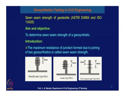
The main objective of this test: to determine the sewn seam strength of the geosynthetics material. So, maximum resistance of the junction formed due to the joining of two geosynthetics is called the sewn seam strength. We can see here different types of the difference types of the joining system and this is the butterfly seam type that is SSd-2.
