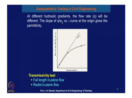
In case of the permittivity, it is a filtration and in case of the trasmittivity it is a drainage; that means, when the water flow along the plane of the geosynthetics material.
