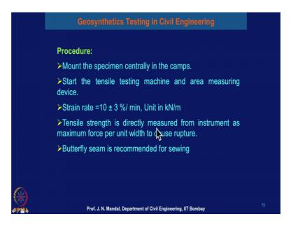
So, procedure mount the specimen centrally in the camp start the tensile testing machine and the area measuring device. And, as I said the strain rate is 10 plus minus 3 percentage per minute and the unit of the seam strength is in terms of the kilo Newton per meter. So, tensile strength is directly measured from the instrument, as maximum force per unit with to cause the rapture. It also told that butterfly seam is recommended for the same.
