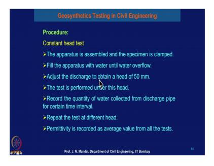
And, this is the this is the different hydraulic gradient of flow rate that is q will be the different types the slope of q by A of g versus delta of h curve, at the origin which will give you that what will be the permittivity of the geosynthetics material?
