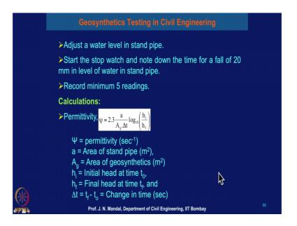
So, adjust a water level in the stand pipe and then we can start the stopwatch and note the time for a fall of about 20 millimeter in the level of the water in the stand pipe. So, we record the minimum 5 reading.
