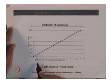
This x axis with its height from the center of the bulb was the hydrometer reading that is in centimeter and this is the hydrometer reading, so that 1.02, 1.02, 1.02, 1.015, 1.01 like this is the hydrometer reading so this is the calibration of the hydrometer so knowing the that what will be the height of the center from the bulb to the hydrometer reading so you can calculate that what will be the hydrometer reading.
