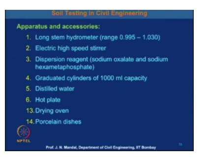
And the accessories you require long stem hydrometer that range about 0.995 – 1.030, you required electric high speed stirrer this dispersion reagent horizontal sodium oxalate and sodium hexametaphosphate, then graduated cylinder of 1000ml capacity with have sodium and they required the distilled water, hot plate, drying oven and the porcelain dishes. So these are the accessories required for performing the test.
