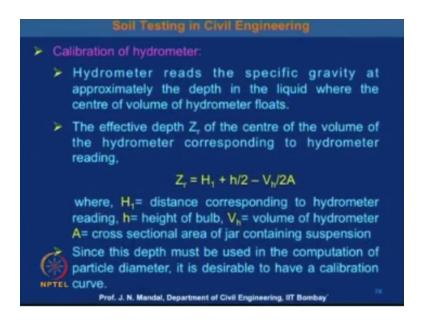
This is important to calibrate the hydrometer and how you can calibrates the hydrometer, so hydrometer reads the specific gravity at approximately the depth in the liquid where the center of the volume of the hydrometer floats. The effective depth which we discussed that is  $Z_r$  of the center of the volume of the hydrometer corresponding to the hydrometer reading that means we can express that.
