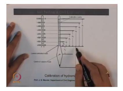
This is H and this is  $H_g$  so this is the lowest calibration mark here and this is center of the volume of the bulb and this is small is the height and this is calibration height for any reading  $D_1$  you can measure 25 then 1.0025 like this 20 so you can calibrating this mark like this also. also you can use this calibration of hydrometer.
