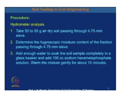
So procedure for the hydrometer analysis first of all we have to take above 50 to 55g of air dry soil passing through 4.75mm sieve. Then determine the hygroscopic moisture content of the fraction passing through 4.75mm sieve you know that how to determine the hygroscopic moisture content. And then add enough water to soak the soil sample completely in a glass beaker and add 100 cc sodium hexametaphosphate solution so warm the mixer gently for about 10 minutes. Now transfer the mixture.
