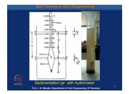
So this is the sedimentation jar with the hydrometer, so here I can tell you this from here to here.
