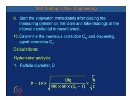
Immediately after placing the measuring the cylinder on the table and take the reading at the interval mentioned in the record sheet. And then determine the meniscus correction which I explain earlier how to calculate the meniscus correction that is Cm and then also we have to determine what will be the dispersing agent correction that is Cd. Now we have to calculate that what should be the particle size diameter.
