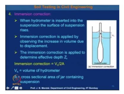
So you can see the, this is the distilled water here and this is the hydrometer and this is the immersion correction and how we go for the immersion correction this, what we what to discuss. So immersion correction is applied by observing the increase in volume due to the displacement. The immersion correction is applied to determine the effective depth and that effective depth is
