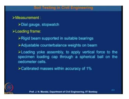
And correspondingly you measure what should be the dial gauge. For a specific time you take the dial gauge reading the loading frame rigid beam supported in suitable bearing, adjustable counterbalance weight on beam loading yoke assembly to apply vertical force to the specimen loading cap through a spherical ball on the eodometer cell. Calibrated masses within accuracy of 1% I will show you that equipment what we can use for the, what to perform the consolidation test.
