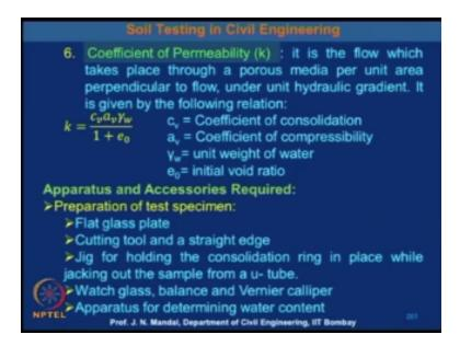
Now other term is the coefficient of permeability and that is denoted by K, and coefficient of permeability also you can determine from the consolidation test his is the indirect method to determine the coefficient of permeability. So coefficient of permeability is the flow which take place through a porous, media or unit area perpendicular to the flow under the unit hydraulic gradient.
