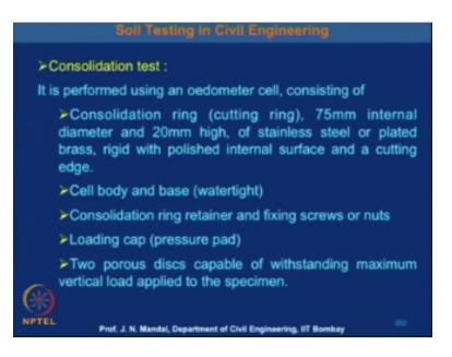
There 75mm internal diameter and 20mm high, of stainless steel or plated brass, rigid with the polish internal surface and the cutting edge. Cell body and base that is watertight and consolidation ring retainer and fix screw or nuts loading cap in pressure pad and two porous this is capable of withstanding the maximum vertical load applied to the soil specimen. Now how to measure the dial gauge and the stop watch we use the stopwatch take the reading time reading.
