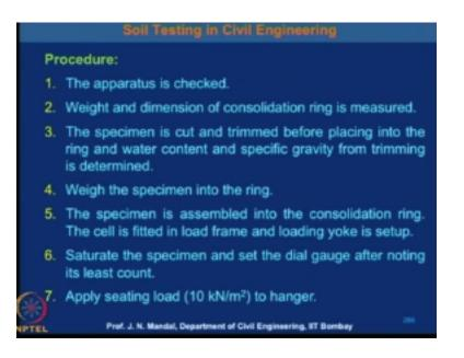
So here some procedure the apparatus is first checked, weight and dimension of the consolidation ring is measured the specimen is cut and trimmed before placing in to the ring I showed you the what is the ring and water content and specific gravity from the trimming is determine so we have to calculate what will be the water content and the specific gravity of the soil sample.
