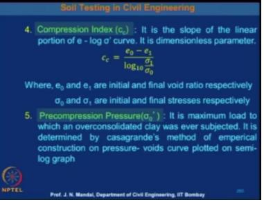
And then the  $C_c$  is express as  $e_0 - e_i / \log of$  based in  $\sigma_1 / \sigma_0$ . So this compression index you can determine form the linear portion of the log e and  $\sigma'$  called all log of p cart from this you can determine this compression index this is also another very important parameter. Then another term which you call the pre compression pressure.
