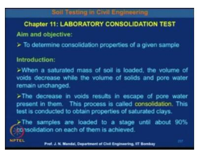
The volume of the void decreases while the volume of the solids and pore water remain unchanged. The decrease in the voids result in escape of pore water present in them the process is called consolidation. This test is conducted to obtain the properties of the saturated clay, the sample are loaded to a stage unit about 90% consolidation on each of them is achieved. Now some of the to understand this consolidation.
