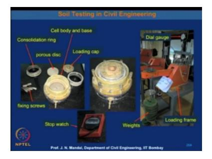
So here is shown that this is the consolidation the ring okay and this is the porous disc and this is the loading cap and this is the cell body and the base. So here is a fixing screw here is a stopwatch you have to take the reading of the dial gauge at a particular time and this is basically consolidated meter equipment, here this is here. And then we have to apply the loading term and here load is applied that weight different weight you have to apply 1, 2, 3, 4 kg load we are applying.
