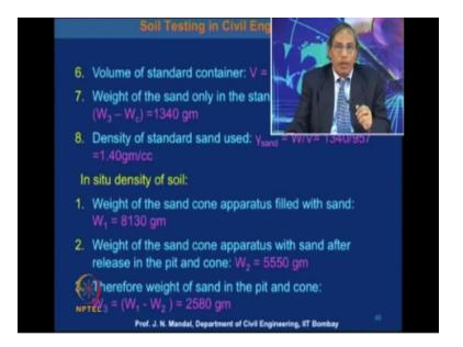
Now you know that what will be the volume of the standard container and that is very standard. Then volume = 957 cc. now weight of the sand only in the standard container W=(W3-Wc) = 1340 gm. Then density of the standard sand used  $\psi_{sand}$  = W/V that is W=1340 this divided by that volume is 957 so the density of the standard sand comes 1.40 gm/cc.
