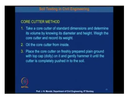
So take a core cutter of standard dimensions and determine its volume by knowing its diameter and height. And weight the core cutter and record is weight. Secondly oil the core cutter from inside and hardly place the core cutter on freshly prepared plain ground with top cap dolly on it and gently harmer it until the cutter is completely pushed in to the soil. Thank you.
