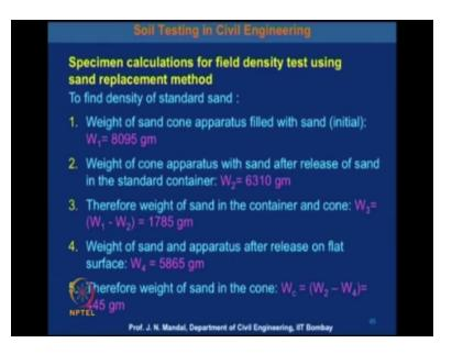
Now specimen calculation for field density test using sand replacement method. So you have to find density of standard sand. First of all it take weight of the sand cone apparatus field with sand initially. Let us see that weight is equal to  $W_1$ =8095 gm. Then weight of the cone apparatus with sand after release of sand in the standard container. Let us see weight is  $W_2$ =6310 gm.
