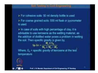
As the addition of distilled water what is the problem in waiting the soil. Then specific gravity is given by equation, specific gravity is equal to  $W_s \ge G_k/W_4 + W_s - W_3$ . Here Gk the specific
