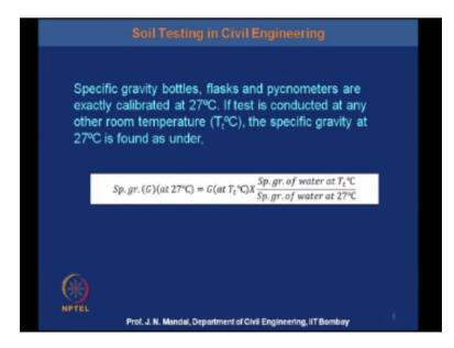
The specific gravity bottle, flask and pynometer are exactly calibrated at 20°C. If the test is conducted at any other room temperature say  $T_1^\circ$  the specific gravity at 20°C also found with this specific gravity G at temperature of 20°C=G(at  $T_1^\circ$ C) x specific gravity of the water at T1°C/specific gravity of the water at 20°C. So some calculation on specific gravity test.
