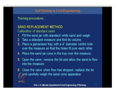
So what are the testing procedural so first of all the sand replacement method he required calibration of the standard sand, fill the sand jar with standard white sand and weigh and I show you that what is the white standard sand so you fill up into the jar and take the weight of the white standard sand and take a standard measure and you can find its volume then, place a galvanized tray with a 4" diameter center hole over the measure so that the hole fit over each other.
