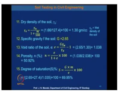
Dry density of the soil,  $\psi$ d also we can determine the moisture density of soil that mean  $\psi$ d =  $\psi_m/1=m/100$  that means that moisture density is (1.66/127.4)100 and that is 1.30 gm/cc. So  $\psi$ m is the weight density of the soil. Then specific gravity of the soil we have determine that is G = 2.65. Then form these data dry density and the moisture content and the specific gravity you can calculate what should be the void ratio of the soil.
