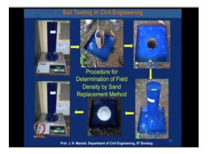
So here you can see the apparatus how you can fill up with sand into this hole and then you can collect it and then it determine that field density of the sand by sand replacement method.
