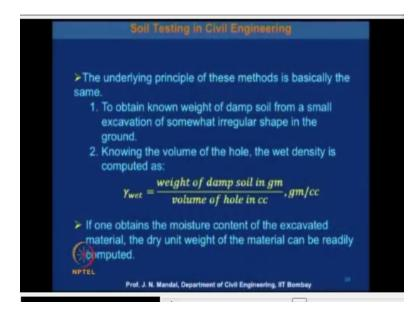
First to obtain known weight of damp soil from a small excavation of somewhat irregular shape in the ground and then knowing the volume of the hole, the wet density is computed as that  $\lambda_{wet}$ will be equal to ratio of the weight of damp soul in gm and the volume of the hole in cc that you can determine what will be the weight  $\lambda_{wet}$  in units is gm/cc. If one obtain the moisture content of the excavated material.
