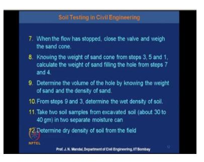
So when the flow has stopped, close the valve and weigh the sand cone. Knowing the weight of sand cone from steps 3, 4 and 1, calculate the weight of sand filling the hole from steps 7 and 4. Determine the volume of the hole by knowing the weight of the sand and density of the sand. So he know that what the volume of the hole he know what the weight of the sand so he can determine the density of the sand. From step 9 and 3, determine the wet density of soil.
