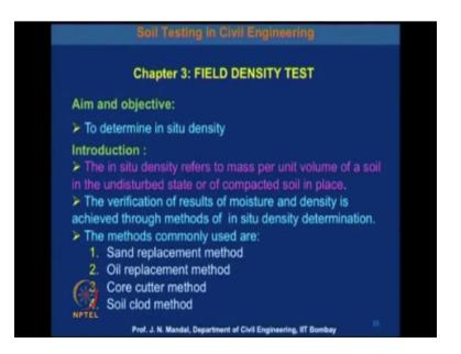
Aim and objective: To determine in situ density. These are very important that how you can determine in situ density f the soil. Now the in situ density refer to mass per unit volume of a soil in the undisturbed state or of compacted soil in place these very important that one should they collect the undisturbed soil sample not the disturb soil. And then the verification of results of moisture and density is achieved through methods of in situ density determination.
