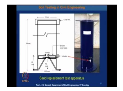
Now here you can see the sand replacement test apparatus and this is the cone these dimensional area is 200mm and this is 8.5 mm and the core cutter it can be replace and it can fill up with the sand and you can measure what should be the volume.
