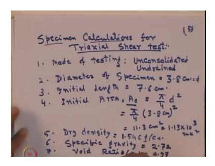
So this is the specimen calculation for tri-axial shear test. So first that mode of testing, mode of testing that is unconsolidated undrained test. Now you know the diameter of the specimen is equal to 3.8cm and next initial length of the sample is 7.6cm. Next initial area that is  $A0 = \pi/4$  into let us say  $d^2$  if d is the diameter of the specimen if this is D. So you can write  $\pi/4$  3.8 this is cm, this is square you can have  $11.3cm^2$  or  $1.13x10^3$  this is  $mm^2$ .
