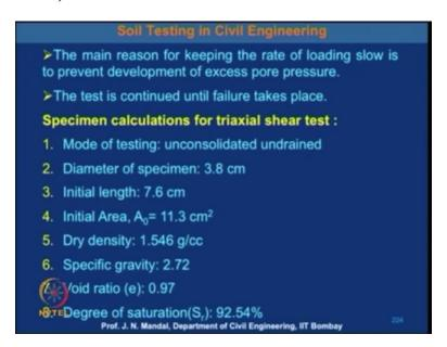
Now the main reason for keeping the rate of loading slow is to prevent the development of excess pore water pressures. And this test is continued until failure take place, I just see some specimen calculation or tri-axial shear test.
