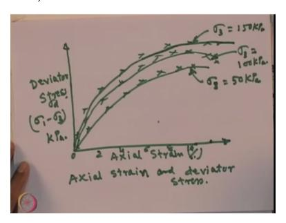
Suppose if you draw a line like this the axial strain, this is axial strain okay that is in percentage and this is the deviator stress and that is  $\sigma 1 - \sigma 3$  we say  $\sigma - \sigma 3$  or you can say  $\sigma 4$  and that is in kilo Pascal. So this under defined axial strain this value may be 2, 4, 6, 8, 10 like this 12. So from the table you know what will be the axial strain which is known to you the axial strain value and now what will be the deviator stress.
