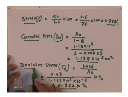
So strain can be in terms of the percentage that is  $\Delta L/L0x100$ , so what is  $\Delta L$ , because your deformation is 0.6. So 0.6 deformation this divided by I say the length of the sample as I told you earlier that is 7.6cm or here it will be the 76m. So this is the initial length of the sample this into 100 so you can have this value it 0.789%.
