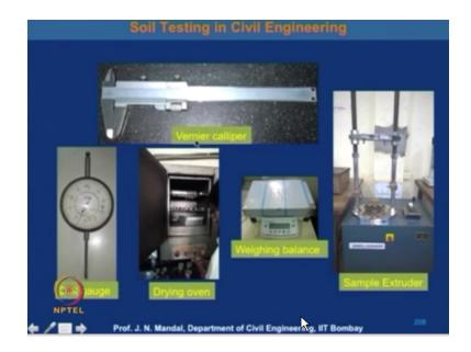
This one is the venire capillary this one and this is the dial gauge here target which you can measure then this is the drying oven in which keep the sample or dry and this is the waiting balance you can wait the soil specimen and this is the sample exclusion any sample is to be excluded from the mould for the testing and here also unconfined compression test.
