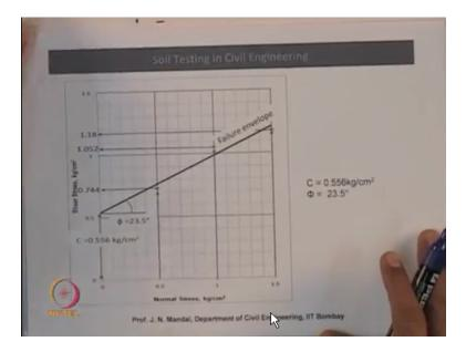
And then there is 1.18 now we can plot the good graph in between the normal stress and the shear stress for the determination of the parameter so and the showing that what should be the normal stress and what should be the shear stress value so here you can see the figure this is a normal stress and this is the shear stress so we know that when the normal stress is normal stress is 0.5 when the normal stress is 0.5 then shear stress is 0.74 for that means when the normal stress is 0.5 here.
