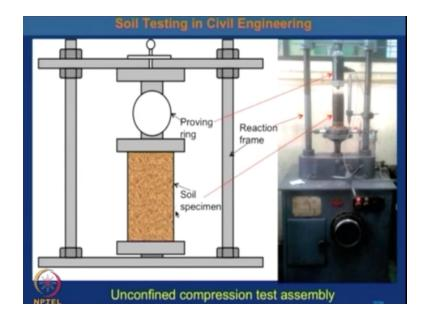
This is the test assembly and here is the soil you can see soil specimen here is a proving ring and this is the reaction frame so this is the soil sample this unconfined compression test and you can see this is the this soil sample is here and you can apply the load at a particular speed and then you measure what will be the unconfined compression strain of the soil.
