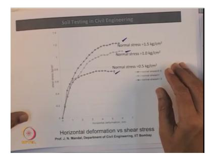
So under the different normal stress so you can plot the curve in between the shear stress and the horizontal deformation so this is the under normal stress of 0.5 kg/cm<sup>2</sup> this is for 1 kg/cm<sup>2</sup> and this is for 1.5kg/cm<sup>2</sup> so here including the normal stress and shear strain value also a column is increasing now there are different types of the test and if it is a if it is a unconfined compression test.
