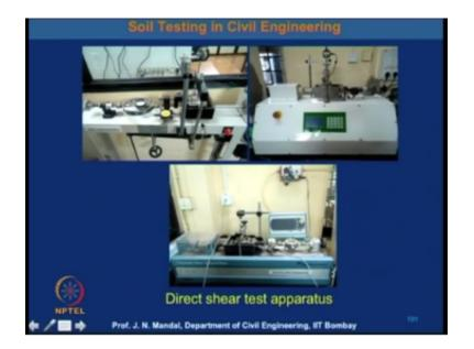
This is the shear direction box takes apparatuses what is separately explain you this is all direct shear box test okay any way the shear strength parameter of the soil is determine using this shear box test.
