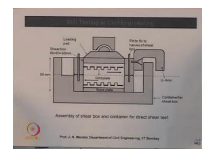
Now I can show you this is the assembly of the shear box and the container for direct shear test this is the lower plate this is base plate and these are the upper part and this is the loading pad and this is the shear box so size is about 16 to 60 and the 50 mm and here is a pin to fix the hope of the shear box and this is 50 cm this is 60/ 60 there is a base plate there is a grid plate and this is the u arm and this is the container for the shear box.
