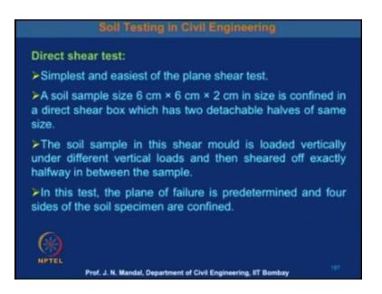
Direct shear test these are simplest and easiest of the plane shear test a soil sample of Size 6cm x 6 cm x 2 cm in size is confined in a direct shear box which have 2 detachable halves of same size. The soil sample in this shear mould is loaded vertically under different vertical loads and then shear of exactly half way in-between the sample in this stage the plane of value is predefined and 4 side of the soil specimen are confined.
