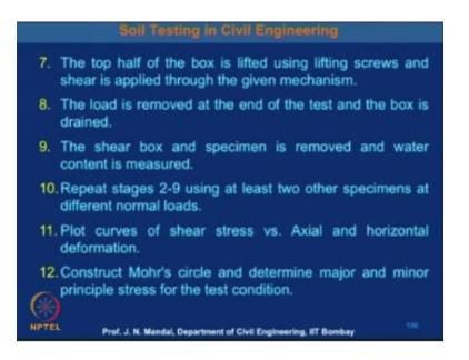
So with this kind of the test you can determined that what should be the shear stress what should be the axial and the horizontal deformation then you determine what will be the major and the minor principles stage under this condition, so this will be very this parameters shear strength parameter will be very useful in geo technical engineering thanks.
