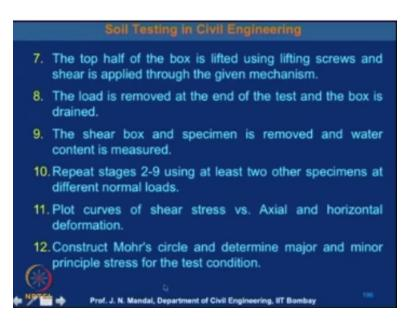
And water contain is measure repeat the stage 2 - 9 using at least two other specimen at the different normal loads then plot curves or shear stage verses axial and the horizontal deformation the construct Mohr's circle and determine the major and the minor principle stress.
