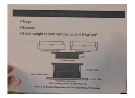
This is the static molding device what direct shear test and this is the MS plate this is remolded soil specimen and this is gelding color this is the direct shear cutter and here is the pressure block this is 6 cm and this is 2cm and this is 9 cm, and this gelding color that is about 6 cm and this is direct shear cutter and this about 6 cm so these are the static molding device for direct shear test.
