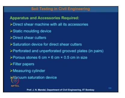
So what are the apparatus and the accessories required for the direct shear test I will now explain that what are the accessory requirement 1 is the direct shear machine with all it is accessory in is the static molding device shear cutter in saturation devices of direct shear cutter populated and unpopulated grouped plate in shears where as stone that is 6cm x 6 cm x 0.5 cm in size filter paper measuring cylinder and vacuum saturation device.
