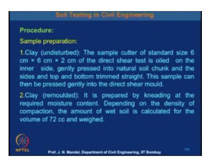
Now how did the procedure call sample preparation that is clear we understand the sample cutter of standard size of 6cm x 6cm into 2 cm of direct shear test is oiled on the inner side gently pressed into natural soil chunk and the sides and top and bottom is timed straight and this sample can then be pressed gently into the direct shear mould if it is a clay remoulded it is prepared by kneading at the required moisture content depending on the density of compaction.
