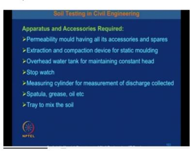
Permeability mould having all its assessory and spare. Extraction and compaction device or static moulding. Overhead water tank for maintaining the constant head, stop watch, measuring the cylinder for measurement of discharge collected. Spatula, grease oil etc. Tray to mix the soil.
