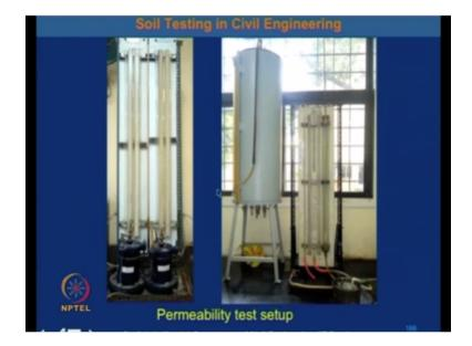
This is the permeability test setup and this is constant head permeability test, this one is the constant heat permeability test and this one is the variable plate permeability test. So we can perform the two kind of the test one is the constant heat permeability and another is the variable heat permeability. This is for the constant heat permeability test and this is for the variable heat permeability test. So you can use both the apparatus for the determination of the permeability of the soil.
