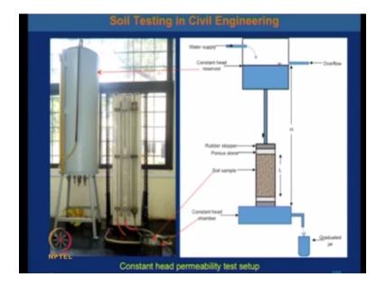
So it pass through the, this is constant heat and let us say this height is about 20.8cm and water which pass through the soil sample and then you collect it here in this jar at a particular time. And then from the jar you will be knowing how much quantity of water you are collecting at a particular time, so let us say that quantity of water collected in this jar is about 36CC for a time let us say in 30 second.
