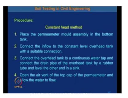
Now let us talk about what will be the procedure for the constant heat method. First of all place the permeameter mould assembly in the bottom tank and then collect the inflow to the constant level over a tank with a suitable connection. Now connect the overhead tank to a continuous water tap and collect the drain pipe of the overhead tank by a rubber tube and level the other end in a sink. Open the air vent of the top cap of the permeameter and allow the water to flow.
