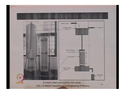
So that this is the soil sample is here and this is the constant head chamber, and this is the soil sample its length is L, and this is the porous tool the top, bottom and this one is the rubber stopper. And this water is supplying at reservoir and that is constant heat water is supplying at a constant heat and then water is overflow from here. So this height from here to here is H, and length of the sample is the L.
