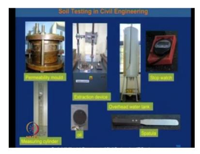
This is the defined types of the assessory required for the permeability test. So this is the permeability mould and this is the extraction device from where the permeability sample are to be extracted using this equipment. And this is the overhead water tank, this is the tank this is the water is inside so this is the overhead water tank and this is the stop watch we have to measure at a particular time the flow of water through the soil.
