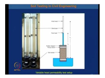
Now this is the variable head permeability test okay. So here the swing that this is the soil sample for variable head permeability and this is the porous stone here, porous stone and this is the rubber stopper.
