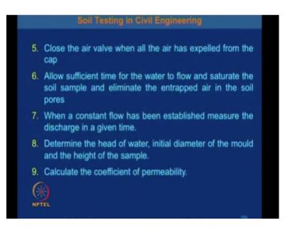
Next close the air valve when all the air has expelled from the cap. Allow sufficient time for the water to flow and saturate the soil sample and eliminate the entrapped air in the soil pores. When a constant flow has been established whether the discharge in a given time. Then determine the head of water, then initial diameter of the mould, and the height of the sample. And then you can calculate that what would be the coefficient of permeability of the soil.
