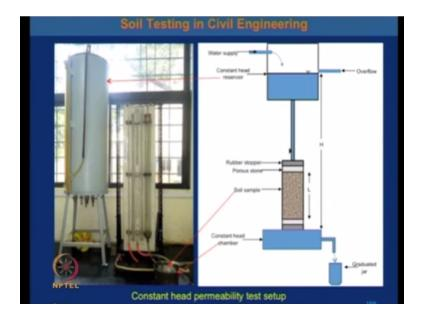
So this is the equipment for the constant head permeability test apparatus you can see here head water rate this is the sample so here I can.
