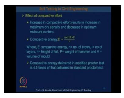
Increase in compactive effort results in increase in maximum dry density and decrease in optimum moisture content. Now this compactive energy we can write. (Refer Slide Time: 00:43)
