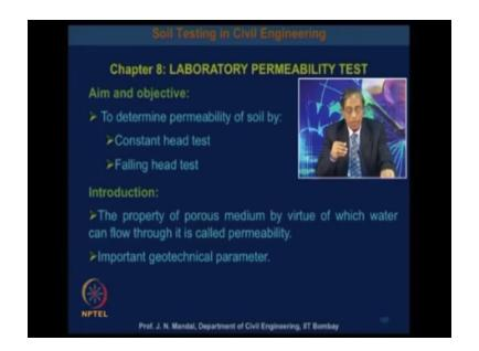
This permeability test is important in soil mechanics and how to perform the permeability of any soil, so the main objective of this permeability test is to determine the permeability of soil and there are methods, one is called the constant head method and this constant head method is particularly for the constant soil and other is called the falling head method and falling head method is particularly for the final gain soil.
