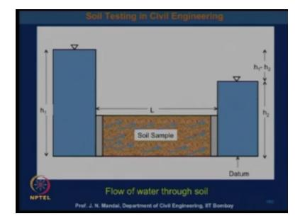
Let us say that this is the soil sample of length is L, and this is h1 here head water is here is h1 and this is water head here is h2 so water can pass from this upper and through the soil sample to this, this is the datum. So there is a difference here is h1 - h2 so if a soil sample of length is l and the sample also has a cross sectional area support a I am just representation here that is the sample length.
