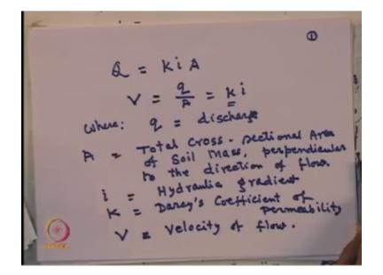
Write that Q = KiA again V = q/A that is ki, now here this small q is the discharge and A is total cross sectional area of soil mass and perpendicular to the direction of flow. And this i is hydraulic gradient and k is Darcy's coefficient of permeability and v is the velocity of flow. So we use that Darcy's law.
