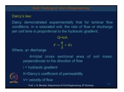
So this important this equation that v = q / a = ki you know what is i, hydraulic gradient and this is the k that is Darcy's coefficient of permeability and this is velocity of flow v.
