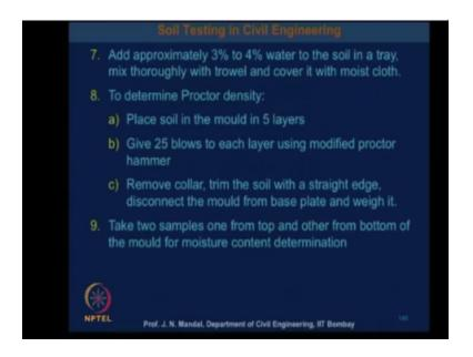
Now add approximately 3% to 4% of water to the soil in a tray and mix thoroughly with the travel and cover it with the moist cloth. Next to determine the proper density place, the soil in the mould in five layer and give 25 blow to each layer using the modified proctor hammer, remove collar, trim the soil with a straight edge disconnected the mould from the base plate and then weight it. Take two sample one from the top and other from the bottom of the mould for moisture content determination.
