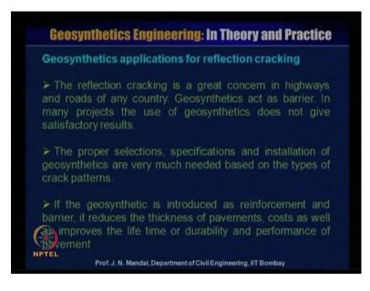
This geosynthetics application for reflection cracking. So, reflection cracking is a great concern in highway and road of any country. Geosynthetics, act as barrier in many project, the use of geosynthetics does not give satisfactory result, because the proper selection specification and installation of geosynthetics are very much needed, based on the type of crack pattern.
