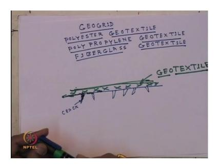
So, it is required to resurfacing the existing pavement due to excessive crack, so this is the crack. So, you provide the bituminous overlay in general ranging in the thickness of 25 to 100 millimetre in the traditional method and crack in the original pavement then reflect up through the new overlay. So, again there is a possibility for the formation of crack on the surface of the road.
