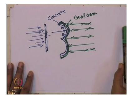
Now, if you simply can place this, if you can simply place a concrete like this and this all the wave, then it will attract this facing of element, which is made of the concrete, because this is a rigid. And there is a possibility for breaking this kind of the concrete because however the force applied on this concrete, it is direct applying on the concrete and this is a rigid, so most of the time it fail.
