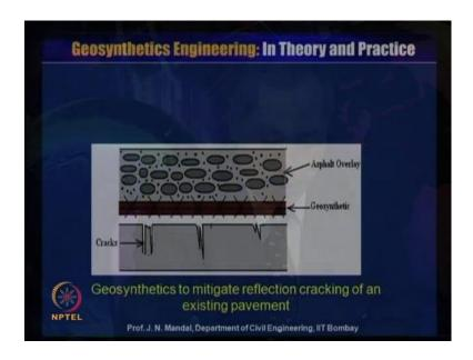
Now, reflection crack prevents an in pavement overlay look at here that if this is the pavement and there is a possibility of different cracking pattern of the road surface.
