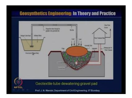
You can see here, for example, this is the Powai Lake sedimentary soil, so this is the dredged cutter head and this is all sedimentary slurry and they you can pump it out and
