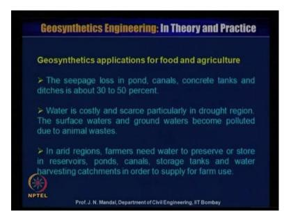
Now, geosynthetics application for food and agriculture, you know that, see page loss in pond tunnel concrete tank, the ditches is about 30 to 50 percentage. Water is costly and scarce particularly in the drought region. The surface water and ground water become
