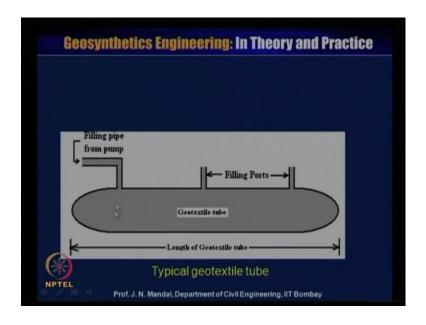
You can see, this is a geotextile tube and that you have to fill all kind of the draining material and fill it to the pipe from pumping and filled up. This is nothing, but a tube and then it can be filled up this is a filling part. So, this is the length of the geotextile tube and fill up and then you can apply the load and then water can be coming out from the geotextile tube. I will later also explain more about this.
