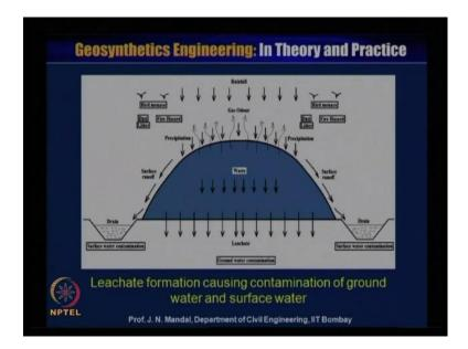
So, this figure you can see that leachate formation caused, during the contamination of ground water and surface water. You can see this is all kind of the waste material and this top if you do not provide any kind of the geosynthetics material, that will be surface
