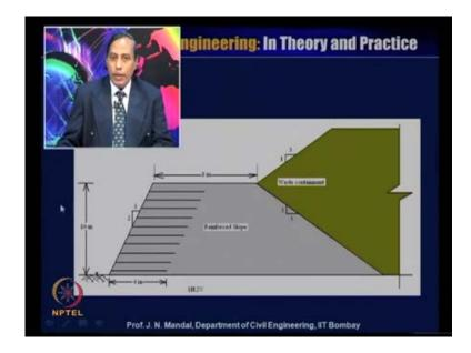
So, you can provide if the multilayer of the reinforcement and also, you can reduce the slope vertical to horizontal is 2 is to 1. So, you can minimize and this also we can see this is the 1 vertical to 3 horizontal, this is 1 vertical to 3 horizontal.
