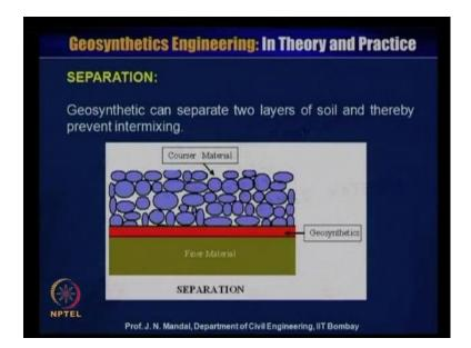
Now, if you place a one layer of the geosynthetics material in between the finer material or courser material.
