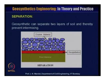
And also geosynthetics material also give a very good tensile strength. So, it can prevent the intermixing between the courser and the finer material. Next is the filtration, is the function.
