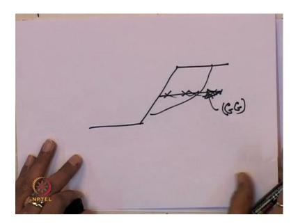
So, this slope without reinforcement may fail. But if you can place one layer of the geogrid material you can say that G G. So, it can be resisted because it has a tensile strength or it act as a good reinforcement.
