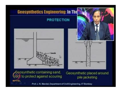
You can have the protection, the geosynthetics containing sand rock to protect against the scouring. Sometimes you can see in the railway bridge where there is a possibility for scouring in this zone and it is eroded and there is a possibility for instability of this structure. So, you can fill up with the good quality of sand or aggregate in a bag and then you can place here in this zone. So, you can save, so you can protect this sphere.
