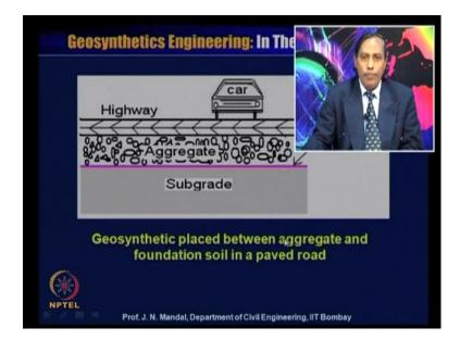
You can acts also geotextile placed between the aggregate and the foundation soil in a paved road. So, you can see that here geosynthetics material act also as a separation.
