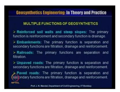
The same material one is acting as a reinforcement as well as it act as a drainage function. When you construct the embankment, the primary function is separation. It separate the finer material to the courser material and secondary function are the filtration, drainage and the reinforcement.
