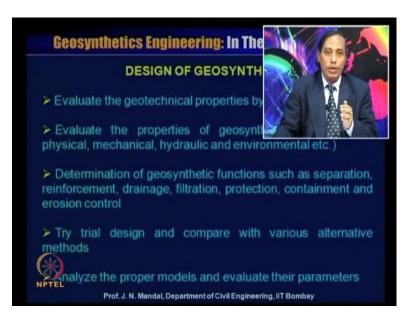
So, many design of the geosynthetics material. It is necessary to evaluate the geotextile property by soil exploration thoroughly. Then evaluate the properties of the geosynthetics material. There are physical property, mechanical property, hydraulic property, environmental property. Then determination of the geosynthetics function such as separation, reinforcement, drainage, filtration, protection, containment and erosion control.
