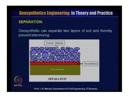
Now, what is separation? So, geosynthetics can separate the two layer of soil and thereby prevent the intermixing. Let us say that separation.
