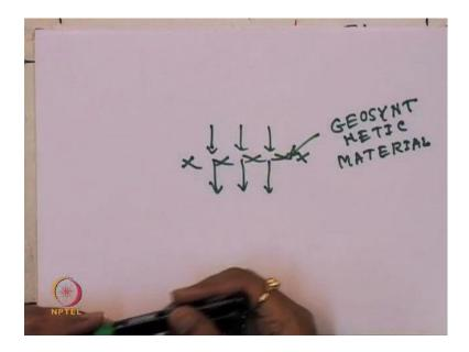
So, in case of the filtration function I am just showing you that if this is the geosynthetics material then liquid can pass across the plane of this geosynthetic material. This is geosynthetics material. So, you remember that when the water or liquid pass across the plane of this geosynthetics material, it called the filtration. And it call also the permittivity.
