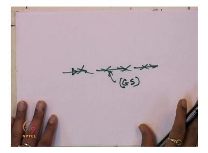
So, if this is the geosynthetics material which is designated at G of S and liquid should pass along the plane of the geosynthetics material which you call the drainage, and within the plane of the geosynthetic material, so at adequate liquid flow within the plane of the geotextile material.
