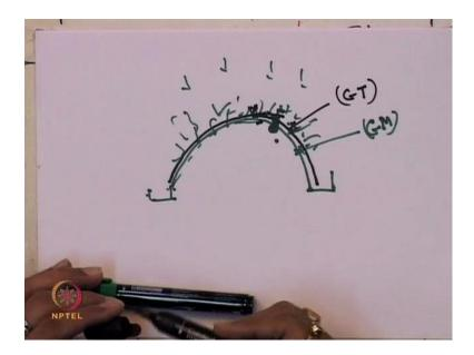
So, if you wanted to construct a tunnel like this. This is the drainage and you can see there are rock or there may be a triangular kind of the rock, which can if this is the geomembrane material. It is a geomembrane material, then this concept of the rock can penetrated into the geomembrane and there is a possibility for damage and leakage and when the rain, the rain water can pass through this geomembrane material.
