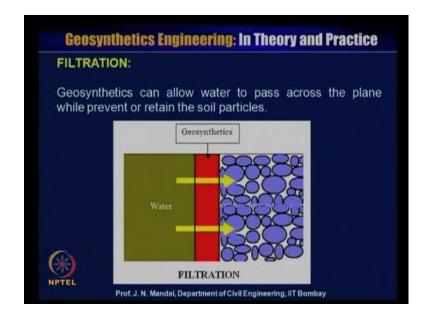
So, geosynthetics can allow water to pass across the plane while prevent or retain the soil particle. You can see here. This is the geosynthetics material and water or liquid which is rushing across the plane of this geosynthetics material. So, here geosynthetics material act as a filtration function.
