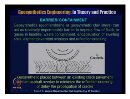
The geosynthetics or the geomembrane or geosynthetic clay liner can act as a relatively impermeable barrier to improve flow of fluid or gases in landfill waste containment encapsulated of swelling soil asphalt pavement overlays and reflection cracking. Here you can see that geosynthetics material placed between an existing crack pavement. This is the crack formation of crack in the pavement and asphalt overlay to minimize the reflection cracking or delay the propagation of the crack.
