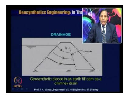
Now, here the geosynthetic material placed in a earth fill dam as a chimney drain, act as a chimney drain. So, this is the drainage. So, geosynthetics, this is the geosynthetics material. So, water can percolate along through this along the plane of the geosynthetics material. That is why it is the drainage. So, geosynthetics placed in a earth fill dam which is a chimney drain.
