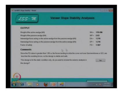
You can determine what will be the factor of safety, this factor of safety is come 1.507. So, since this factor of safety is greater than 1, then force tending the slide that cover soil over the geomembrane or geosynthetic clay liner are lesser than the resisting force. So, design is stable and safe.
