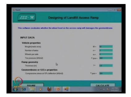
The input data vehicle property, that weight w is 50 metric tons, the number of axis is 2 and that is wheel per axle m is equal to the 4 and this is the this is the tire pressure. The sigma tire pressure is equal to 480 kilo Newton per meter square. Then ramp geometry
