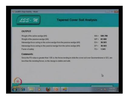
So if you substitute or input this data case A, so this is the output weight of the active wedge W A is equal to 508.706 kilo Newton, weight of the passive wedge W P is equal to 82.488 kilo Newton. Interwedge force acting on the active wedge from the passive wedge that is E A is equal to 36.503 kilonewton, interwedge force acting on the passive wedge from the active wedge that is E p is equal to 36.503.
