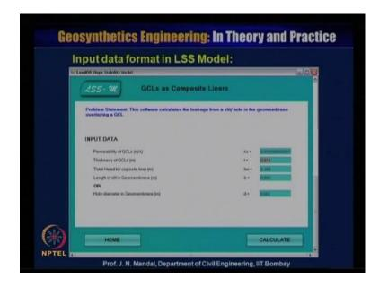
Now, we have put this input data formulation it over LSS model and this problem statement that this software calculate, what will be the leachate from any slit or hole in the geomembrane, and overlying by geosynthetics clay liner. Here, input data is permeability of the geosynthetics clay liner is equal to 7 into, note this data we have put 7 into 10 to the power minus 12 meter per second.
