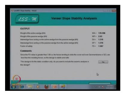
So, for the introduction of the reinforcement for slope stability, now we calculate and we find that output is weight of the active wedge W i is equal to 178.496 kilo Newton weight of the passive wedge w p is equal to 2.63 kilonewton. Interwedge force acting on the active wedge from the passive wedge EA is 1.216 kilo Newton, interwedge force acting on the passive wedge from the active wedge that is E P is 1.216 kilo Newton and the factor of safety value is F s is equal to 1.507.
