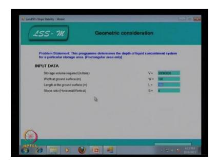
This is the input data what will be the storage volume required, let us say this is the v and this is in liter and you know the what will be the width of the ground surface that 100 meter length. So, the ground surface is 100 meter and the slope ratio that is horizontal to vertical s is equal to 4.
