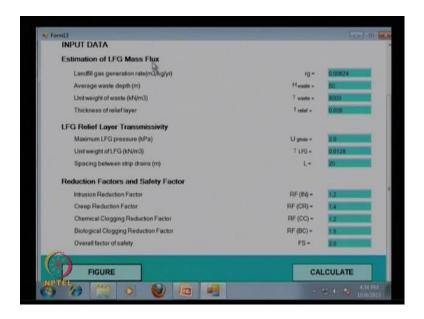
This is the estimated LFG mass flux, this is landfill gas generation that is 0.00024, that is the unit meter cube per k g per year. Average waste, that is h waste is equal to 50 meter, unit weight of the waste gamma is equal to 8 thousand that is kilonewton per meter cube.
