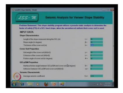
So, this is seismic analysis of veneer slope stability analysis, here the slope charateristic the length L 35, beta 15 degree, h is 0.35 meter. Cover soil property gamma is 18 degree, C is equal to 0, phi is equal to 32 and GCL geomembrane property delta is equal to 18 C a is equal to 0 and here the seismic characteristic the average seismic coefficient C a is 0.10.
