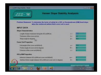
So, we are keeping almost this slope characteristics value A that is the length of the slope, the height of the thickness of the cover soil. This friction angle, also this is the soil cover property, that is gamma phi and C and the that is gamma is 17.5 phi is 30 degree,
