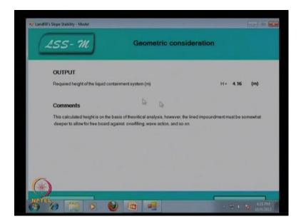
So, you can calculate and can determine that what will be the required height of the liquid containment system, that is H is equal to 4.16. So, you can calculate the height on
