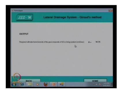
Then, you calculate and find the required ultimate transmittivity of geomembrane or the GCL lining system that is theta, 14.73 centimeter per second. So, then design of the landfill for access ramp, that is access ramp one and there is a access ramp like this.
