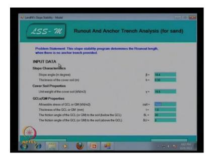
Then, this is the runout problem statement, the slope stability program determine the runout length when there is no anchor trench provided. So, input data soil characteristics slope angle beta 18.4 degree and thickness of the cover soil H is equal to 0.30 meter. Cover soil property unit weight of cover soil gamma that is 16.5 kilonewton per meter cube and GCL and geomembrane property.
