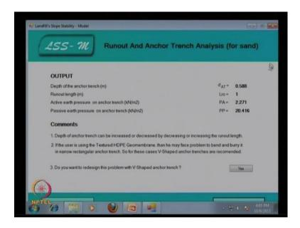
So, then you can obtain the output data what will be the design of the anchor trench, that is D a t which we are interested, that means D a t is equal to 0.588 and runout length L t 0 is equal to 1 meter. So, you can calculate P a and also the P p, so comment depth of the anchor trench can be increased or decreased by decreasing or increasing the runout length too.
