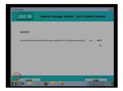
Then, you calculate and find that the required ultimate transmissivity of the geomembrane, geosynthetic clay liner lining system is theta is equal to 20.27 centimeter per second.
