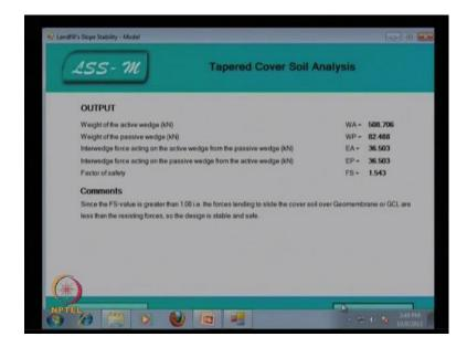
Now, this is for the tapered cover soil, so this is the output of the tapered cover soil analysis the output is weight of the active wedge W A is equal to 508.706 kilo Newton, weight of the passive wedge W P is equal to 82.488. Then interwedge force acting on the active wedge from the passive wedge E A 36.503 kilo Newton. Interwedge force acting on the passive wedge from the active wedge that is E P is equal to 36.503 kilo Newton.
