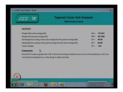
Then, you calculate, you can have the output the weight of the active wedge W a is 775.967 for passive W p, 207.999 and the E A is 66.88 kilo Newton and E P is 66.88 kilo Newton and factor of safety 1.64. So, you find the factor of safety value is greater than 1, so it is the safe and stable structure. So, we will discuss seismic analysis for veneer slope stability analysis without reinforcement, that is Qian 2001.
