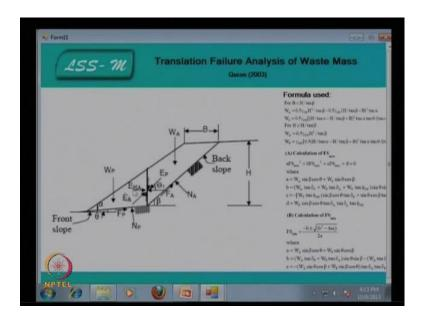
This is the waste mass, how it fail, so if the waste mass fail it is also necessary to properly design this. So, in this program also this problem statement this programme determine the factor of safety value for the landfill for translation waste mass failure analysis. The input data that is geometric data that has height of the slide slope H is equal to 30 meter and top width of the slope b is equal to 20 meter.
