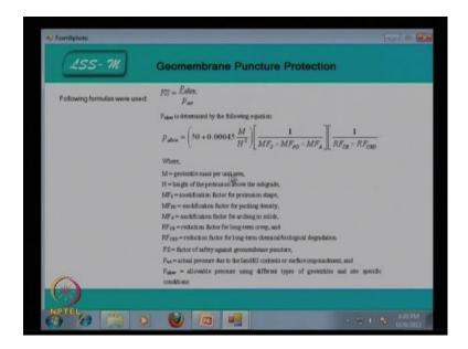
So, if there is a puncture geometric puncture protection, so this is equation has been used.
