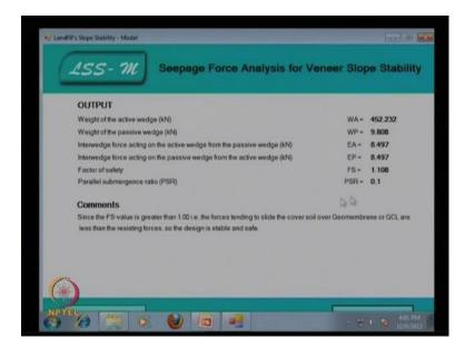
So, you can calculate and can determine what will be the factor of safety this factor of safety value is 1.108 and parallel to the submergence ratio, which is called PSR is 0.1. So, here we find the factor of safety value is greater than 1, so it is safe. So, now the runout and the anchor trench analysis of sand Koerner 1997, that is runout.
