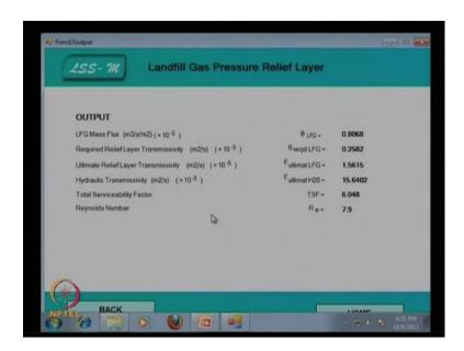
So, the landfill output gas pressure relief, you can have that mass flux phi U g is 0.8068, this is the theta required L f g is 0.82582 and this is the epsilon ultimate L f g is 1.5615 and epsilon ultimate is equal to 15.640. This is the total serviceability factor T s f is 6.068 and the reynold number is equal to 7.9 geocomposite gas pressure relief layer.
