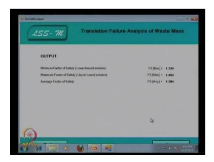
Now, if you calculate this, so you can have the output that is minimum factor of safety lower bottom solution F s minimum 1.334. The maximum factor of safety of the upper bottom solution F s maximum is 1.454 and average factor of safety that is F s average 1.394, so it is safety and the safe then it is ok. So, application of the GSL as a liquid containment liner.
