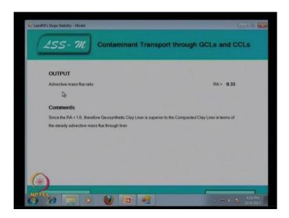
So, you can calculate what will be the advective mass flux ratio, that is R a is equal to 0.33. Since the R a value is less than 1, therefore geosynthetic clay liner is superior to the compacted clay liner in terms of the steady advective mass flux through the liner and if it is a steady diffusive mass flux.
