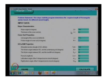
So, we can use this is a problem statement, the slope stability program determine the required depth of the rectangular anchor trench for the different. So, here slope charateristics beta is 18.4 and the thickness is 0.3, this is the cover soil property that gamma is is equal to 17.3, phi is equal to 35. This is geosynthetics and geomembrane property t allowable is equal to 19.8 kilo Newton per meter and the friction angle between GCL and the underlying soil delta C is equal to the 18.
