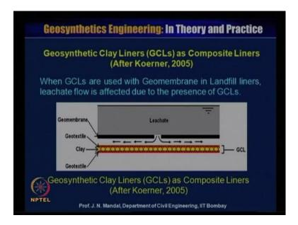
Now, I will address the geosynthetics clay liner GCL as a composite liner after Koerner 2005, when the geosynthetic clay liner is used with the geomembrane in landfill liner. Leachate flow is affected due to the presence of the geosynthetics clay liner, so what will happen? Sometimes, it has been observed that if there is no geomembrane or the geosynthetics clay liner, then leachate can percolate through the ground surface and polluted the ground.
