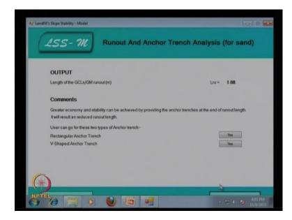
Now, you can calculate and you can find that what will be the length of the GCL or that is L is 0, that is 1.888. So, comment if it is a greater economy and stability achieved by providing the anchor trench at the end of the runout length. It will result to reduce the runout length, so user can go of these two types of the anchor trench either the rectangular anchor trench or v shaped anchor trench.
