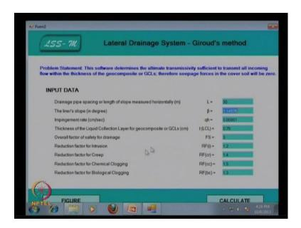
So, next lateral drainage system in the giroud method, so giroud method also this is the lateral drainage system for the Giroud's method. This is the equation has been used into this programme and this is the drainage pipe that spacing length of the measurement horizontally L is equal to 30 meter. The liner slope angle beta is equal to 1.345 that is degree and this is the impingnated rate that q h centimeter per second is 0.000001.
