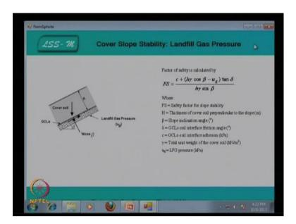
So, if there is a development of cover soil stability, where there is a development of gas if gas there is a leachate and gas pressure developed here. So, you have to calculate that what will be the factor of safety, so you can calculate and you find the factor of safety value 1.05. Now, for the lateral drainage system for unit gradient ratio for lateral drainage system for unit gradient ratio.
