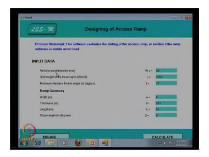
This is the vehicle weight that is W v is equal to, that is 55 metric ton and unit weight of the base layer gamma 2100 kilo Newton per meter cube and minimum interface friction angle delta is equal to 12 degree. The ramp geometry is width is equal to w, is equal to 6 meter thickness, t is equal to 0.61 meter and the length is equal to L 50 meter and slope angle degree is beta is 8.
