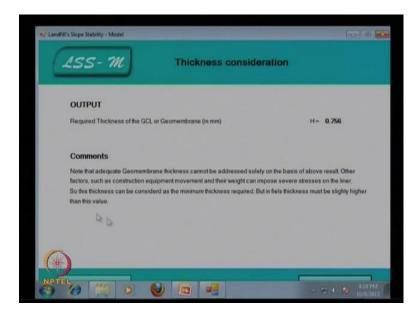
So, with this programme then ultimately you can have the required thickness of the geomembrane or geosynthetic, that is h is equal to 0.766 millimeter. Sometimes, though it is on the it is 0.776, it is preferable always you put in the higher thickness. Then you can give the 1 meter or you can 1.5 or 2 meter. So, because it is sometimes necessary that when you dump this any waste material and it is compacted, there is a possibility for the
