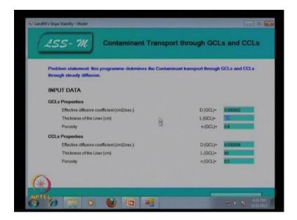
If it is a steady diffusive mass flux, this is the problem statement, the programme determine the contamination transport through GCL and the CCL through the steady diffusion. So, input data GCL property effective diffusive coefficient, that is d for the
