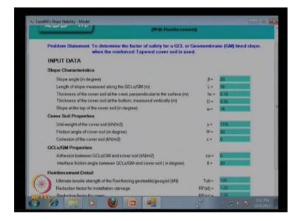
So, then you have to include what will be the slope characteristic, that is beta is equal to 20 degree. Then L the length of the slope is 35 meter and thickness of the cover soil h c 0.15 and thickness of the cover soil at the bottom measured vertically D is equal to 0.30 and slope at the top of the cover soil that is small, w is equal to 16 degree. Cover soil
