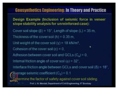
So, this is one design example inclusion of the seismic forces in a veneer slope stability analysis for unreinforced case cover soil slope. Beta is equal to 15 degree, length of the slope L is equal to 30 meter and thickness of the cover soil h is equal to 0.35 meter, unit weight of cover soil gamma is 18 kilo Newton per meter cube, cohesion of the cover soil c is equal to 0, adhesion between cover soil.
