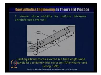
Next, 2 the veneer slope stability for uniform thickness unreinforced cover soil. So, there is no reinforcement and this is the slope and this is limit equilibrium forces involved in a finite length slope analysis for a uniformly thick cover soil, this after Koerner and Soong
