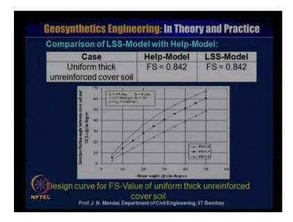
So, here some comparison of landfill slope stability model with the help model case uniform thick unreinforced cover soil that is with the help model factor of safety is equal to 0.842 and the landfill slope stability model factor of safety is 0.842. So, you can see that LSS model is satisfying with the help model that means it satisfy that criteria that means LSS model is now this is the design curve for the FS vale of uniform thick unreinforced cover soil.
