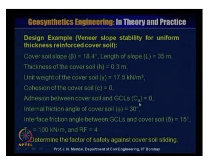
So, now I am giving one design example of veneer slope stability for uniform thickness reinforced cover soil. Let us say cover soil slope beta is 18.4 degree, length of the slope L is equal to 35 meter, thickness of the cover soil h is 0.3 meter, unit weight of cover soil gamma is equal to 17.5 kilo Newton per meter cube, cohesion of the cover soil c is equal to 0, adhesion between cover soil.
