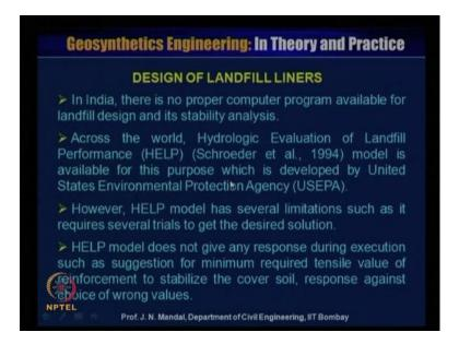
We are more interested here the design of the landfill liner. How can we design the most of the cases? We provide with something that thickness of the geomembrane or geosynthetics clay liner and they are introduced into the landfill in many project but one has to be very careful there are many, many issue which are need to be addressed for the design of the landfill liner.
