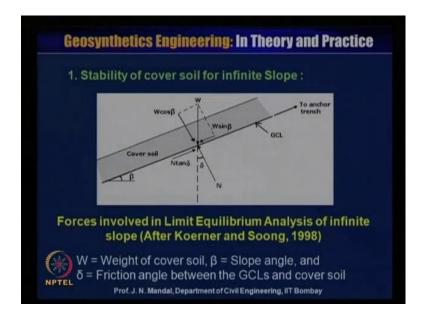
Here you can see that what are the forces involved in limit equilibrium analysis of infinite slope, This is after Koerner and Soong 1998. Here this w the weight of the cover soil and beta is the slope angle and this is the delta is the friction angle between the geosynthetics clay liner and the cover soil. So, this cover soil has a thickness and also this is the geosynthetic clay liner or geomembrane.
