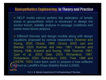
HELP model cannot perform the estimation of tensile stress in geosynthetics, which is necessary to design the anchor trench stability analysis in seepage condition and waste mass failure analysis. Sometime also in the landfill it has been observed the waste mass itself is failure.
