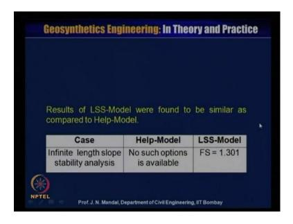
Here result for LSS model was found to be similar as compared to the HELP model. So, case with the infinite length slope stability analysis help model, no such option is available more or less that landfill slope stability model, which give factor of safety is equal to 1.301. So, it is a safe.
