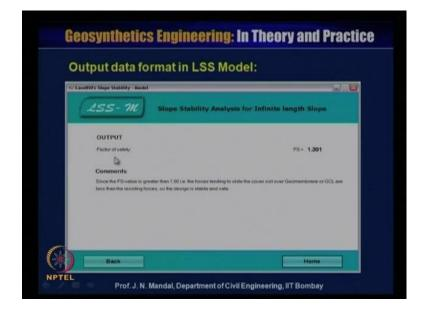
Now, you have to input this data into this model and then you calculate and then you can have the what will be the output, you can see the factor of safety is equal to FS 1.301. So, you can make a comment that since the factor of safety value is greater than 1.00 that is the force tending to slide the cover soil then over the geomembrane or geosynthetics clay liner are less than the resisting forces.
