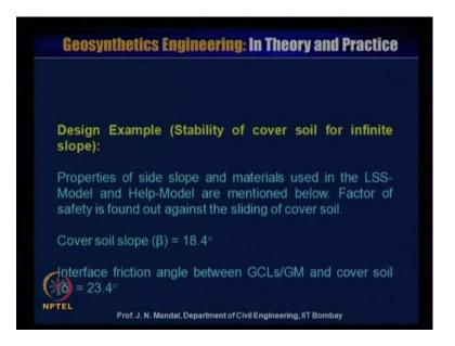
Now, property of the side slope and the material used in the LSS model that is landfill slope stability model and the help model are mentioned below. Factor of safety is found out against the sliding of cover soil and cover soil slope angle beta is equal to 18.4 degree. Interface friction angle between the geosynthetic clay liner or geomembrane and cover soil that is delta is equal to 23.4 degree.
