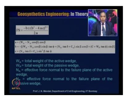
So, from this you can calculate what will be the factor of safety with this equation minus b plus minus b square minus four a c whole to the power 0.5 divided by two a, where a is equal to W A minus N A cos beta into cos beta. Hence b is equal to minus W A minus N A cos beta into tan phi plus N A tan delta plus C a into sin beta into cos beta plus C plus W P tan phi into sin beta. And c is equal to N A tan delta plus C a into sin square beta into tan phi.
