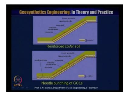
So, here also shown the reinforced cover soil apart from the geomembrane or geosynthetics clay liner. You can provide with the reinforcement to make a proper slope. You can make any steeper slope or the angle as you like it. So, you can provide sometimes the geosynthetic clay liner also the geomembrane also the geonet. This is all combination of the geosynthetics material.
