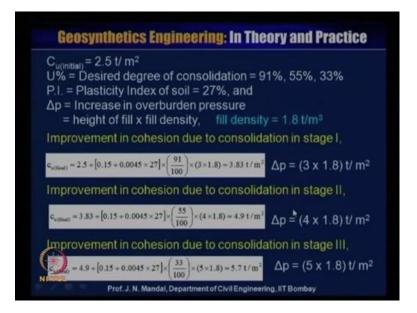
So, C u initial is given 2.5 ton per meter square where, U is desired degree of consolidation 91 percent, 55 percent and 33 percentage. PI is the plasticity index of the soil is 27 percent and delta p is the increase in overburden pressure, that means is equal to height of the fill into fill density. Fill density is given 18 ton per meter cube so improvement in cohesion due to consolidation in stage 1, that mean Cu final will be equal to 2.5.
