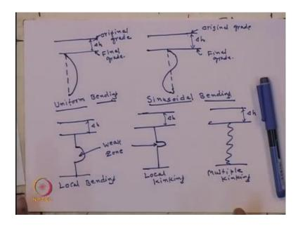
So, what may happen that in some cases, that if this is the drain and this is the original grade and this is let us say delta of h and here the relatively, the uniform soil mass and here is the final. So, this drain may be uniformly bending so there is a possibility for uniform bending or it may, if this is the drain so it may be like this, like this, that mean this is sinusoidal bending, this kind of the bending may occurs.
