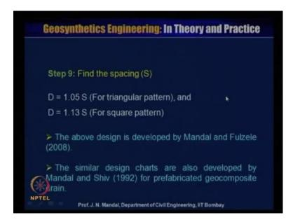
Step 9, now find the spacing that is S so you know that D is equal to 1.05 S for triangular pattern and D is equal to 1.13 S for square pattern. So, this above design chart is also developed by Mandal and Fulzele, 2008 and similar design chart are also developed by
