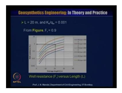
Now, you know the length is equal to 20 meter and Kh by qw is equal to 0, 0.001. So, from this figure you can calculate what is F of r so here is the design length, length is 20 meter and here is the Kh by qw that is 0.001 Kh by qw. So, this is 0.001 so if you know Kh by 0.001 then you move to the left and then you can calculate what is Fr. So, Fr is near about 0.9 so from this chart you calculate Fr.
