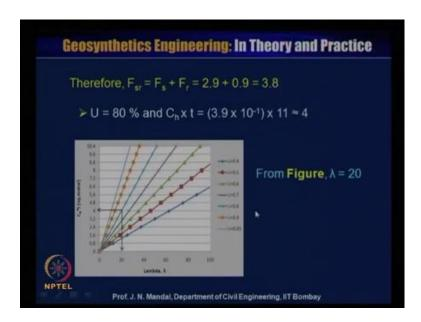
Now therefore, you know that Fsr is equal to Fs plus Fr, that means 2.9 plus 0.9 will be equal to 3.8. Now, U is equal to 80 percent given Ch into t also 3.9 into 10 to the power
