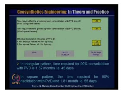
So, you can calculate so what will be the time required, for the given degree of consolidation with PVD in month 1.62. And time required for the given degree of consolidation, with PVD is 1.81 when, there is a square pattern and earlier one when, there is a triangular pattern. So, effective diameter of influence of PVD that is for triangular pattern is 1.05 into spacing, that is why it give 1.26 and for 2 for square pattern is equal to 1.13 into spacing that is 1.356.
