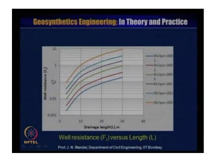
So, this is the chart well resistance versus the length, this is the length for different value of Kh by qw, Kh by qw 0.001, 2, 0.002, 0.005, 0.01, 0.02, 0.05. So, knowing the value of Kh by qw, Kh is coefficient of permeability in the horizontal direction and qw is the flow. So, if you know this ratio of this and what will be the drainage length so you know the drainage length, you know the Kh by qw then you can calculate, what will be the well resistance factor from this chart that is F of r.
