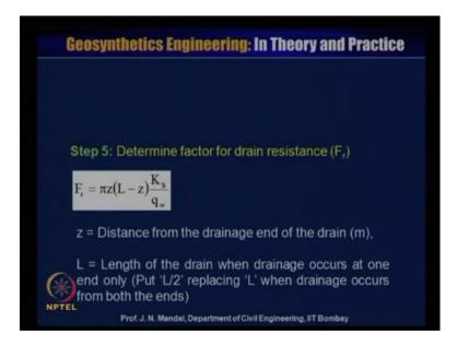
Now step five, determine factor for drain resistance that is Fr so use this equation drain resistance that is Fr is equal to pi z L minus z into Kh by qw. What z is equal to the distance, from the drainage end of the drain that is meter, L is equal to length of the drain when, drainage occur at one end only or put L by 2 replacing L when, drainage occurs from both the end.
