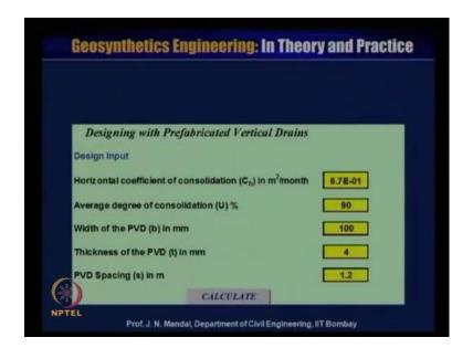
Now, design with prefabricated vertical drain you can put, the design input horizontal coefficient of consolidation Ch in meter square per month, 6.7 into 10 to the power minus 1. And average degree of consolidation U is, 90 percent width of the PVD in millimeter 100 millimeter, thickness of the PVD t in 4 millimeter so PVD spacing S in 1.2.
