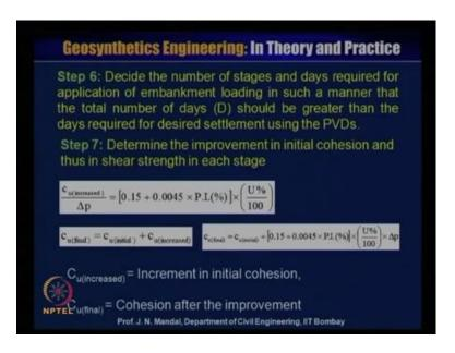
Step six, decide the number of the stages and days required for application of embankment loading. In such a manner that the total number of the days D, should be greater than the days required for the desired settlement, using the prefabricated vertical drain. Step seven, determine the improvement in initial cohesion and thus shear strength of in each stage. So, Cu increased divided by delta p is equal to 0.15 plus 0.0045 into PI in percentage, into U by 100 percentage.
