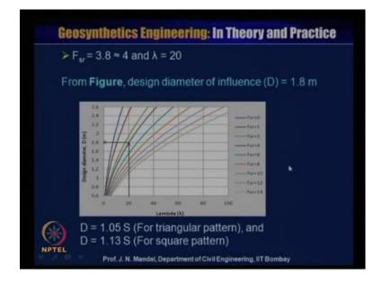
So, you know Fsr is about 3.8 or is equal to 4 and lambda is equal to 20. So, from this figure design diameter of influence, that is D you can calculate now, here that, what is the Fsr, that means Fsr is about 4. So, this is Fsr will be about 4, here Fsr 4 and you know the lambda is equal to 20 so lambda 20 then you move up, where Fsr is equal to about 44. And then you move horizontally here then you can obtain that what will be the design diameter D.
