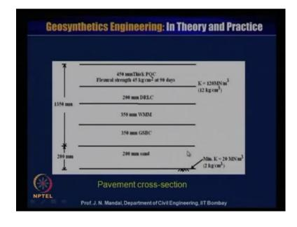
So, this is the pavement cross section so this is the 450 millimeter thick PQC, flexural strength is 45 kg per centimeter square at 90 days. And this k value is given 120 MN per meter cube, that means 12 kg per centimeter cube. And this is 200 millimeter DRLC, this is 350 millimeter that is WMM and 350 millimeter GSBC and 200 millimeter sand and here minimum k is 20 MN per meter cube or 2 kg per meter cube. This depth is about 200 millimeter from and here to here is about 1350 meter.
