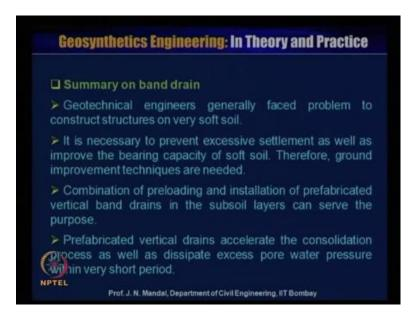
So, summary of the band drain, geotechnical engineer generally faced problem to the construction structure, on very soft soil. So, it is necessary to prevent the excessive settlement, as well as improve the bearing capacity of soft soil therefore, ground
