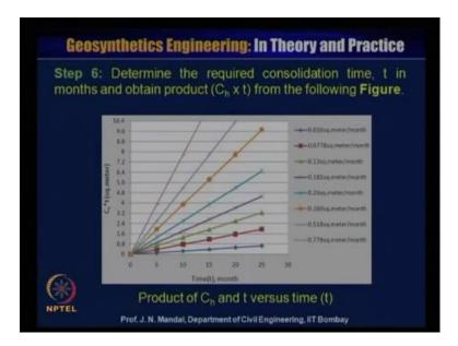
Step six, determine the required consolidation time t, in month and obtain product Ch
