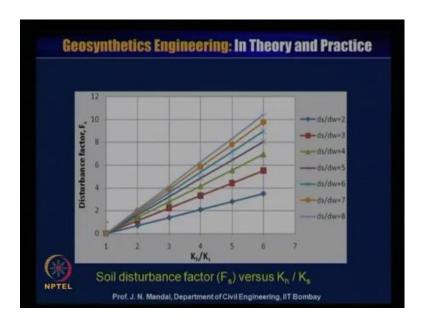
So, this is the figure, is shown that soil disturbance factor Fs versus Kh upon Ks. So, for the different value of ds by dw, so ds by dw may be 2, 3, 4, 5, 6, 7, 8 like this. So, for the
