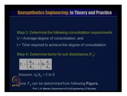
Step three, determine the following consolidation requirement that is, U is average degree of consolidation and t, time required to achieve the degree of consolidation. Step four, determine factor for soil disturbance, that is Fs so we will use this equation Fs is equal to Kh by Ks minus 1 into log ds by dw. Assume ds by d w is equal to 2 to 8 now, Fs can be determined from this following figure.
