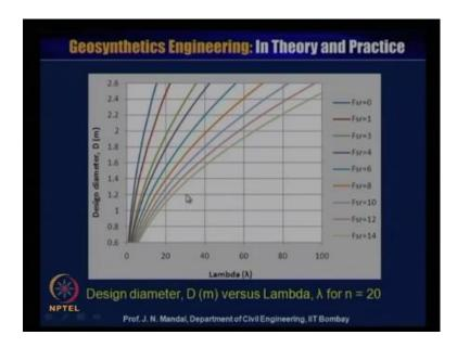
So, now this lambda here is the design diameter that is D in meter versus, the lambda for n is equal to 20. And here that Fsr is may be 1, 0, 3, 4, 6, 8, 10, 12 and 14 so different values. So, knowing also the lambda and Fsr so you can also calculate what will be the design diameter from this chart.
