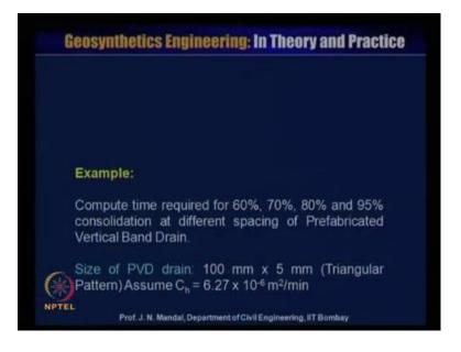
Compute time required for 60 percent, 70 percent, 80 percent and 95 percent consolidation, at different spacing of prefabricated band drain. Now, the size of the PVD drain is suppose given 100 millimeter into 5 millimeter and we are considering, this is a triangular pattern. And assume that Ch value is 6.27 into 10 to the power minus 6 meter square per minute.
