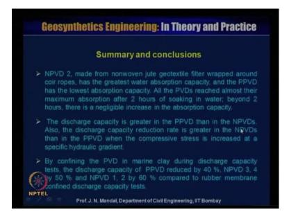
So, we come to some summary and conclusion that natural prefabricated vertical drain 2 made from nonwoven jute geotextile filter wrapped around coir rope has the greatest water absorption capacity. The polyester prefabricated vertical drain has the lowest absorption capacity you have observed that from the curve. All the prefabricated vertical drain reached almost their maximum absorption after 2 hours of soaking in water, beyond 2 hour, there is a negligible increase in the absorption capacity.
