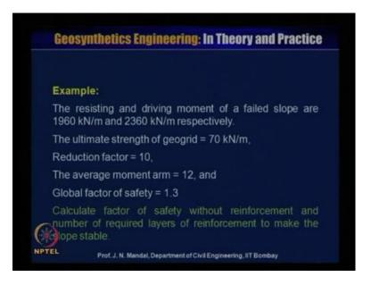
Now, I will present an example, the resisting and the driving moment of a fail slope are 1960 kilo Newton per meter and 2360 kilo Newton per meter respectively. Ultimate strength of the geogrid is 70 kilo Newton per meter, reduction factor 10 average moment arm 12, and global factor of safety 1.3. Calculate the factor of safety without reinforcement and number of required layer of reinforcement to make the slope stable.
