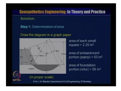
Now, the solution step a determination of the area. So, draw the diagram in a graph paper and you consider that in the graph paper the area of each small square is equal to 2.25 meter square. So, you have to check you have to check that what will be the area of this is the embankment. So, area of the embankment; that is p q S r p, so this area is equal to 63 meter square, because you know area of each small square is 2.25 meter square, so this embankment area will be equal to 63 meter square.
