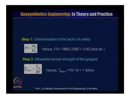
Step one, determination of factor of safety, so you know factor of safety is equal to resisting moment by driving moment. So, FS is equal to 1960 by 2360 is equal to 0.83,
