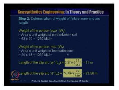
Now, step two determination weight of the failure zone and arc length, so weight of the portion of the p q is r; that is weight of the embankment W e. That is area into unit weight of the embankment soil. So area you have seen this is area is 63 meter square, so this 63 unit weight of embankment soil is given 20, so 63 into 21 260 kilo Newton per meter. Similarly, weight of the foundation that is r S T u that is W F; that means area into unit weight of foundation soil area is 59.
