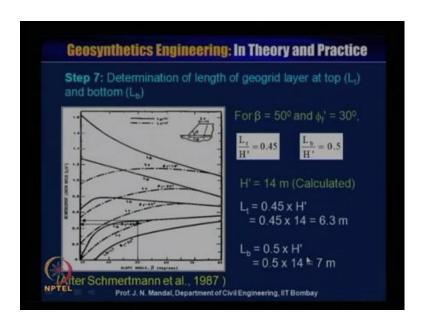
Now, step seven, determination of length of geogrid layer at the top is L t and at the bottom is L b. So, this is the design chart after Schmertmann et al 1987 and this is the L b bottom. This is the L t top and this angle is slope beta and this is firm line is L b by H dash and dotted line is L t by H dash [FL] length at that top and length at the bottom and H is equal to height of the slope. So, here you can see that when a one is the firm line another is another is the dotted line.
