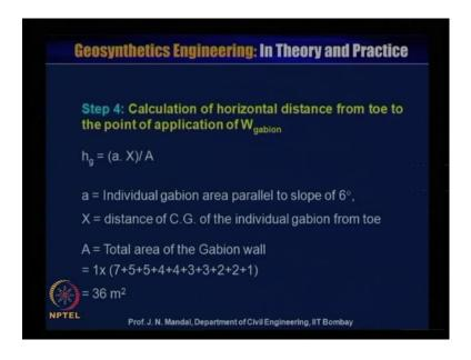
Now step 4, calculation of the horizontal distance from the toe, to the point of application W gabion also, we explained what is hg, a into X divided by capital A. A is equal to individual gabion area, parallel to the slope of 6 degree and X is equal to distance of the C G of the individual gabion from toe. So, here A total area means 1, into area I say initially 7 then, plus 5 plus 5 then, plus 4 plus 4, plus 3 plus 3, plus 2 plus 2 and plus 1. So, area will be equal to 36 meter square.
