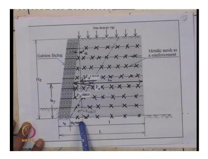
So, this will be the middle tg by 2 plus this is Hg tan alpha, that means Hg by 2 into tan alpha because tg is equal to wall thickness, Hg is equal to wall height and alpha is the wall inclination, with the vertical. So, you can calculate what is the Hg, Hg means this half of tg by 2 plus, half of Hg into tan alpha. Now step 5, calculation of weight of the surcharge.
