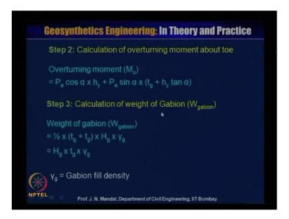
Now step 2, calculation of overturning moment about toe so overturning moment Mo again is equal to Pa cos alpha because horizontal force is acting Pa cos alpha, I show Pa.
