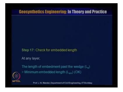
Step 17, check for embedment length, at any layer the length of the embedment past the wedge is Le. So, it should be minimum embedment length L em then it is okay. So, you have to check.
