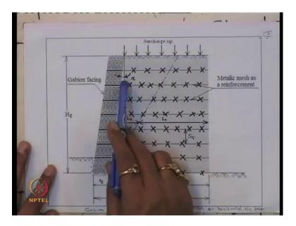
This is the gabion wall with welded wire anchor mesh, as a horizontal tie-back. So, this is fixed with the gabion, this is gabion as a facing and there is a surcharge and this is metallic mesh as a reinforcement. This is the failure line so we will design this structure and also, this is the failure surface which is making at an angle 45 degree plus phi s by 2.
