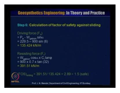
Step 6, calculation of the factor of safety against sliding. So, driving force Fd is equal to Pa minus W gabion into sin alpha so Pa we calculated 229.5, W gabion is 900 into alpha is equal to 6 so sine 6 degree. So, driving force Fd is equal to 135.424 kilo Newton per meter, resisting force Fr is equal to W gabion into cos alpha into Ci tan alpha, this is the resisting force, at the base.
