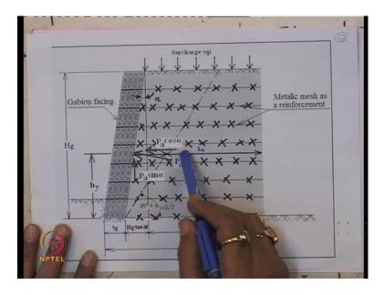
So, this is like, like this what I say that this is the P of a which is, this distance is hy and this is h of d and also Pa has the component of Pa cos alpha and also, the Pa sin alpha. So, we are interested to determine that the value of hy, so this value of hy can be calculated using this equation.
