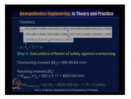
Now, with this equation so you have to calculate that h of g so this h of g you can see here for the 7, 1 this is for 5 and this is for 5, 2 then 4 and 4 this 2 then, after that 3 and 3 another 2 then, 2 and 2 another 2 and then, only 1. So, like this from the geometry of the gabion, you can calculate the hg and this hg value will be 5.17 meter. Step 5, calculation of factor of safety against overturning. So, you have calculated overturning moment Mo is 599.99 kilo Newton meter per meter.
