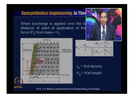
Now, when the surcharge is applied over the backfill, the vertical distance of the point of application of the resultant normal force that is, P of a. This, P of a from the base, this from the base is h of, h of y so here is the h of y, here hy. So, this h of y can be calculated with this equation, that is Hg by 3 into Hs plus 3 q by gamma s divided by Hg plus 2 q by gamma s, where gamma s is equal to soil density, Hg is equal to wall of height.
