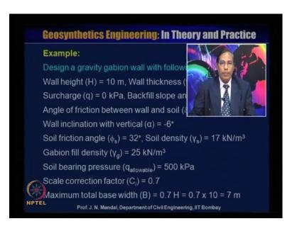
Now, I will present an example, design of gravity gabion wall with the following data. The wall height is about H is 10 meter, wall thickness tg is 1 meter, surcharge load q is 0 kilopascal, backfill slope angle i is 0, angle of friction between wall and soil delta is 0. Wall inclination with the vertical alpha is minus 6 degree, soil friction angle phi s is 32 degree, soil density gamma s is equal to 17 kilonewton per meter cube, gabion fill density gamma g is 25 kilonewton per meter cube.
