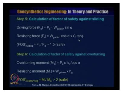
Step 5, at a calculation of factor of safety against sliding that means you have to calculate driving force Fd is equal to Pa minus W gabion into sin alpha. Resisting force Fr, is equal to W gabion into cos alpha into Ci tan phi. So, then you calculate what will be the factor of safety against sliding, is equal to Fr by Fd, it should be greater than 1.5 then, it is safe.
