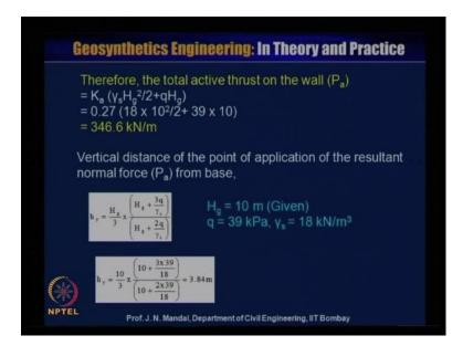
Therefore, total active thrust on the wall Pa will be equal to Ka gamma Hg square by 2 plus q into Hg, Ka you know 0.27, 0.27, gamma s value is given 18 and Hg is 10 square divided by 2 plus q is the surcharge load, is 39. And Hg is equal to 10 so you can calculate that, what will be the total active thrust on the wall Pa is 346.6 kilo Newton per meter.
