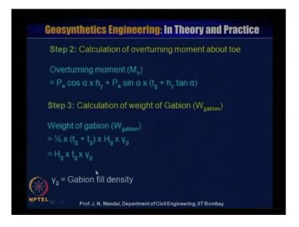
Where, this gamma g is the gabion fill density because this gabion is fill up with the stone. So, we know the, what is the gabion fill density, you can calculate the weight of the gabion.
