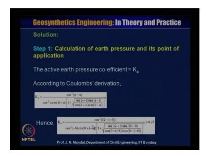
Now, for the solution so step 1, what we have already theory we have explained and step 1 here, calculation of earth pressure and its point of application. So, active earth pressure
