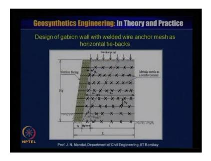
Now, design of gabion wall with welded wire anchor mesh as a horizontal tie-back now, here you can see that.
