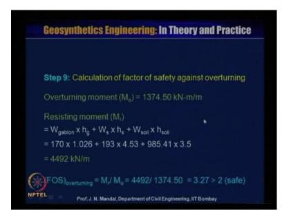
So step 9, calculation of factor of safety against overturning so overturning moment we calculated Mo is equal to 1374.50 kilo Newton meter per, meter resisting moment Mr is equal to W gabion into Hg plus Ws into hs plus W soil into h soil. That means we know that, W gabion 170 into Hg is 1, we calculated Hg is 1.026 plus Ws is 193 plus hs we calculated 4.53 and W soil is 985.4 one and h soil we calculated 3.5.
