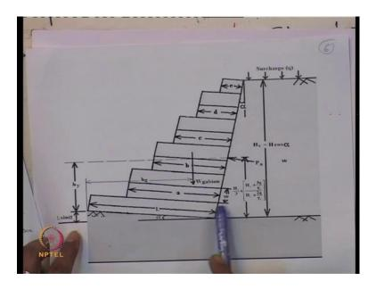
That, this is the A, that individual area of gabion parallel to the slope and then, you will be knowing, what will be the X distance, that means distance of the c t c g of the individual gabion, from the toe. And A is the total area of the gabion wall, you know this, you know this length, you know this width so you can calculate area. So, you can calculate what is the h of g that means, h g is equal to a into X divided by A.
