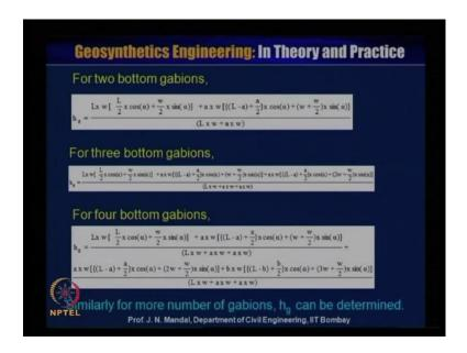
Now, you can also design for two bottom gabion or for three bottom gabion or four bottom gabion. This is from the geometry, you can solve this h of g for the two bottom gabion, this you know L, this is width. So, you know what is L 2 cos alpha into w by 2 into sin alpha plus a into w into L minus a plus a by 2 into cos alpha plus w plus, w by 2 into x sin alpha divided by L into w plus, a into w.
