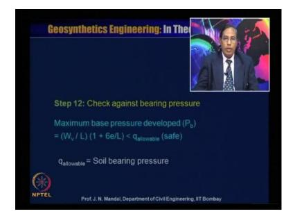
Step 12, you have to check against the bearing pressure so maximum base pressure developed Pb will be equal to Wv divided by L into 1 plus 6 e by L, that should be less than q allowable then, it is safe. So, q allowable where you can say soil bearing pressure.
