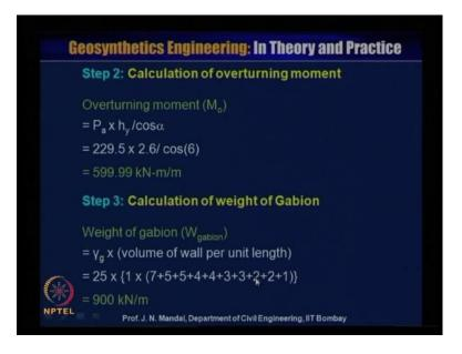
So then step 2, calculation of overturning moment, overturning moment Mo is equal to Pa into hy divided by cos alpha. So, Pa you know 229.5 into hy is 2.6, you calculated divided by cos alpha is 6 so you can have overturning moment Mo is equal to 599.99 kilonewton meter per meter. Step 3, calculation of the weight of the gabion so weight of the gabion that means, gamma g into volume of wall per unit length. So, we are considering unit length and gamma g is given 25, gamma g is given 25.
