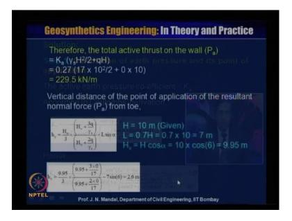
Therefore, the total active thrust on the wall Pa will be equal to Ka into gamma s into H square by 2 plus q H, that is due to surcharge. So, Ka you know that 0.27, gamma s is 17, H is equal to 10 meter height of the wall, that 10 square divided by 2 plus, this no surcharge we have considered so q is equal to 0 and H is equal to 10. So, you can calculate what will be the total active thrust on the wall Pa is 229.5 kilo Newton per meter.
