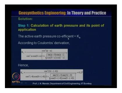
So, solution step 1, calculation of earth pressure and its point of application so active earth pressure coefficient is equal to Ka according to the coulombs' derivation. So, you can calculate Ka using this equation, so you know that phi is equal to 32 degree given, alpha is minus 6, that is why minus 6 and then cos square alpha, cos square alpha is minus 6 into cos delta value is 0 and alpha value is minus 6.
