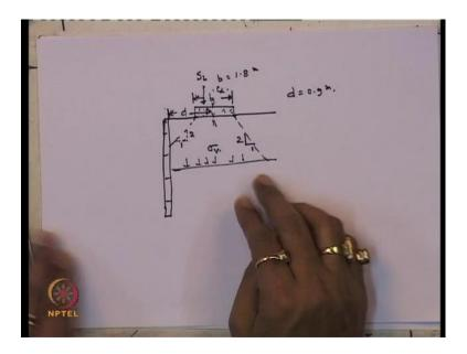
I am showing you that so it is like this and this is b and this b is 1.8 meter and this is the wall let us consider, this is the wall and this is dispersed with the slope horizontal to vertical is 1 is to 2 and similarly, this is also 2 vertical 1 horizontal. So, any strip 1 is the vertical stresses acting, this is sigma of V and this the center line and where, the strip load S L is acting. And from this center line to here, this distance is equal to that is d and this d is equal to 0.9 meter.
