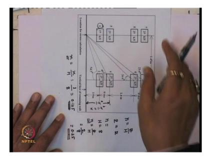
We are calculating location for the stress calculation at this point and this is the wheel 4 so this wheel is the 4, which is making at an angle of 45 degree. Let us say, this is theta is equal to 45 degree and you want to measure the, what will be the stress or which we call the sigma H dash. So, sigma H dash for the wheel load 4, what it will be.
