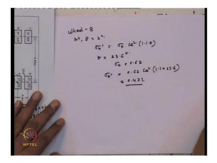
So, let us say, I am just showing you for the wheel load 8 only, wheel 8 at depth z is equal to 2 meter and you know, what will be the sigma H dash. This is equal to sigma of H into cos square 1.1 theta and theta is given 23.6 degree and sigma H at a depth of 2 meter is 0.62. So, you can calculate sigma of H dash is 0.62 into cos square 1.1 and theta is 23.6. So, you can have at a depth of 2 for the wheel load 8 will be equal to 0.472 so this you can obtain 0.472.
