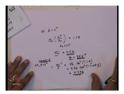
So, we know that equation to calculate the stress that is, sigma of H dash for the wheel 6 and let us say, at a depth of 2 meter so sigma H dash will be equal to sigma H in cos square 1.1 into theta. Now, theta value is known, 26.2 and sigma H value is known so
