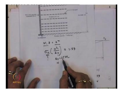
Now, I am showing you here that, we know that sigma of H, H square by Q of p is equal to, you calculate at a depth at z is equal to 2 meter, you calculate this value is 1.59. So, when at a depth of 2 meter, sigma H by H square Q is 1.59, you substitute value n and you find it is, 1.59. Now, you have to calculate sigma of H, this is unknown, H is 8 and Q p is point load that is, 25 that means, this will have a 25, this point we are, this is 25 so Q p is 25.
