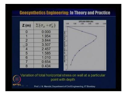
So here, you can see that, variation of the stresses here and this is the depth, at any depth you calculate what will be the total stress. So, you know what is sigma H, you know what is sigma H of dash so you know that, what is the wheel from this table, wheel 7 and any depth, wheel 7 and wheel 8. So, you can calculate, what is sigma H and sigma H
