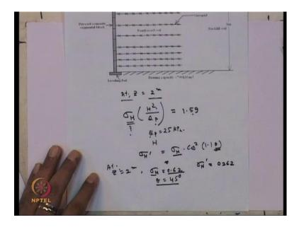
Also here, you want to calculate sigma H dash is equal to sigma H into cos square 1.1 theta. Now, you know at depth let us say, z is equal to 2 meter. So, sigma of H value is known, sigma of H value is equal to 0.62 and theta you know, this is making at an angle 45 degree. So, you substitute the value of sigma H and theta here so then you can calculate sigma of H dash and that will give at a depth of 2 meter about 262.
