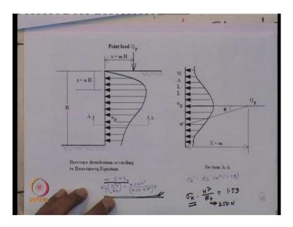
Now, we know that earlier, from this Boussinesq pressure distribution that, if the m value is less than equal to 0.4 sigma H, H square by Q p is equal to 0.28 n square divided by 0.16 plus n square whole to the power cube. If m value less than equal to 0.5, if it is that m value greater than equal to 0.5 then equation is different, which I have explain also earlier.
