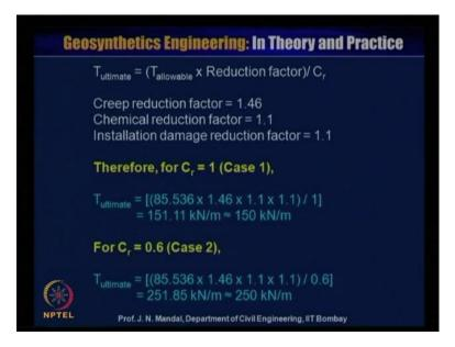
Now, what will be the T ultimate value, that will be T allowable into reduction factor divided by C of r. Now, this reduction factor that we can consider, that creep reduction factor is 1.46, chemical reduction factor is equal to 1.1 and installation damage reduction factor is equal to 1.1. So, all these reduction factor you have to take into consideration and then you have to calculate what will be the ultimate tensile strength of the geotextile geosynthetics material.
