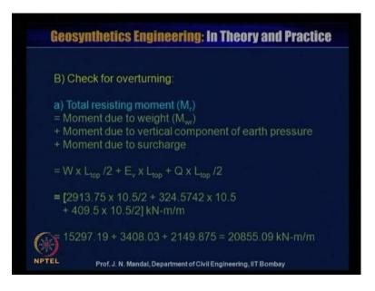
Next, we have check for the overturning so total resisting moment M r is equal to moment due to the weight M w r plus moment due to the vertical component of the earth pressure plus moment due to the surcharge. So that means, you know what is weight, weight into L top divided by 2 E v that mean, moment due to the vertical component of the earth pressure that is, E v into the L top and plus due to the surcharge that is, Q into L top by 2.
