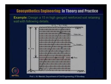
Now, I will present a example, design a 15 meter high geogrid reinforced soil retaining wall, whose following is given details. This is height of the wall, this is 15 meter and this is the failure surface, which is making at an angle of 45 degree plus pi by 2. And there is a live load and dead load, so total load is about 39 kiloPascal.
