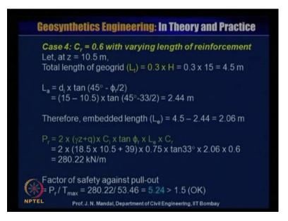
Now, case 4 that, when the coverage ratio is 0.6 with varying length of the reinforcement. So, let at depth z is equal to 10.5 meter so total length of the geogrid L t will be 0.38 that means, 0.3 into 15 that is, 4.5 meter. L a will be equal to d i into tan 45 degree minus phi r by 2 that means, 15 minus 10.5 into tan 45 degree minus 33 by 2 by 2 is equal to 2.44 meter. Therefore, embedment length L e will be equal to 4.5 minus 2.44 is equal to 2.06 meter.
