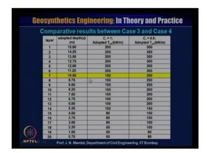
And now, if you compare the result between the case 3 and case 4 so all are 20 layer and this is the adopted that, depth this is the 15 meter height of the wall and we have shown only calculation for at a depth of 10.50. In this example, you see that, when the coverage ratio 1 so adopted ultimate tensile strength value 150 kiloNewton per meter. But, when you are considering C r value is equal to 0.6 or coverage ratio 0.6, adopted ultimate tensile strength value 250 kiloNewton per meter.
