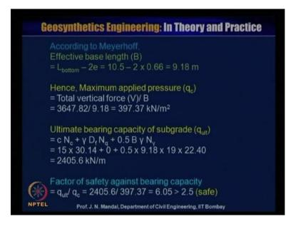
So now, adding M to the Meyerhoff distribution, what will be the effective base width B so effective base width is important, that is equal to L of bottom minus 2 e, L bottom also 10.5 minus 2 e, you calculated 0.66. So, 10.5 minus 2 into 0.66 is 9.18 hence, maximum applied pressure q c is equal to total vertical force V divided by B. So, that is 3647.82 divided by, this is the acting length 9.18 so this is the 9.18 so this is 397.37 kiloNewton per meter.
