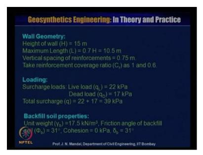
The problem is like this wall geometry, I say height of the wall is 15 meter, maximum length is 0.7 times the height of the wall, that mean 10.5. Vertical spacing of reinforcement is 0.75 meter, take the reinforcement coverage ratio C r as 1 and 0.6. So,
