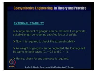
Now, external stability, a large amount of geogrid can be reduced if we provide the suitable length, considering satisfy the factor of safety. Now, it is required to check the external stability, as weight of the geogrid can be neglected, the loading will be the same
