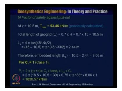
Next, b that, you have to check factor of safety against pullout at depth z is equal to 10.5 so we know that, T maximum is equal to 53.46 kiloNewton per meter. We have already previously calculated now, what will be the total length of the geogrid. We know total length of the geogrid is equal to 0.7 into H, H is the height of the geogrid wall. So, 0.7 into 15 is equal to 10.5 meter, now we have to calculate the L of a.
