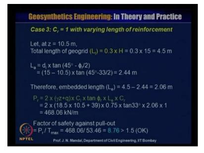
So now, this case 3 we are this varying length, we are considering case 3 that, when coverage ratio is equal to 1 that means, whose varying length of the reinforcement. So, we have shown you that, at a depth of 10.5 meter let us say that, total length of the geogrid L t is equal to 0.3 times H that means, 0.3 into 15, 4.5meter. And at that point, you have to calculate what will be the L of a that means, L a is equal to d i into tan 45 degree minus phi r by 2.
