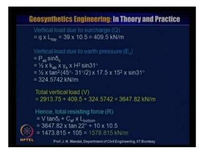
So, we are showing here that, vertical load is equal to P a b into sin delta b and again P a b you know, half into k a b into gamma b into H square into sin delta b, delta b is 31 degree. So, you know half tan square 45 minus 31 by 2 into H, that is gamma b is 17.5 into H is equal to 15 square into sin 31 degree. So, if you calculate, you can have the vertical load due to the earth pressure, E b is 324.572 kiloNewton per meter. What will be the total vertical load then V.
