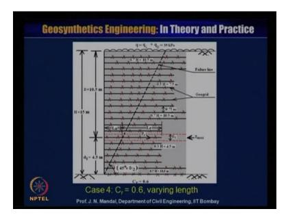
Now, case 4 that, when the coverage ratio is 0.6 and varying the length, it has been shown, it is the layout of the reinforcement. You can see that tough layer, we are providing the three layer here, it is a three layer so it was like this.
