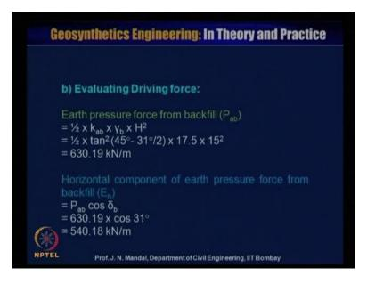
So, this is earth pressure from the backfill that is, P a b. So, you can see here that (Refer Slide Time: 56:27) earth pressure due to the P a b. So, earth pressure force from the backfill is P a b, you can calculate that half into k b into gamma b into H square so this will give you this value.
