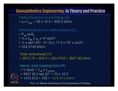
Now, this vertical load due to the surcharge so that is q into L of top, length of the top reinforcement and you know that, q is equal to 39 that is, dead load plus live load and length of the top layer is 10.5. So, this will be equal to 409.5 kiloNewton per meter, what is vertical load due to the earth pressure E v.
