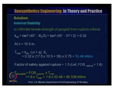
So, to determine the ultimate tensile strength, you have to check what will be the k of a b that means, coefficient of active earth pressure at the backfill soil, that is equal to tan square 45 degree minus phi b by 2. Phi b value is given 31 degree so tan square 45 degree minus 31 degree by 2 is equal to 0.32. So, you know k b is equal to 0.32 now, we are considering that, at a depth z is equal to 10.5.
