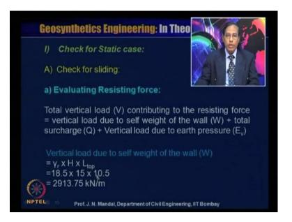
That V will be equal to 2913.75, we have to calculate here 2913.75 that is, vertical load due to the self weight.
