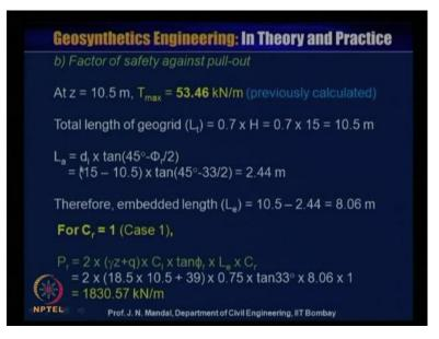
So here, we are just showing that L a, how you have calculated so this is d i means, that is 15 minus 10.5 into tan 45 degree minus phi r value is 33 divided by 2, this is 2.44 meter and embedded length L e, that is total. We know L t, we know that 10.5 so this minus this L of e so this is 2.44. So, this L e will be 8.06 now, for C r is equal to 1, case 1 we are considering and we have to calculate, what will be the P of r that means, what will be the pullout force.
