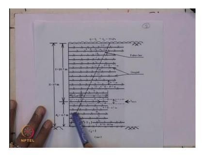
So, what we are doing here that, you can see this in this problem, when the coverage ratio is 1 and this is the case 3 that we are assuming, assuming that in this problem, that we are keeping here. That mean, total length that means, 0.7 times of H that is from the bottom two layer, one and two layer we are giving 0.7 of H, height is 15 meter. So, 0.78 is equal to 10.5 meter so total length L t that is, 10.5 meter from the bottom two layer.
