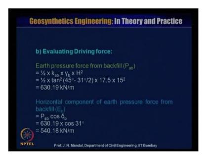
You can see here that, this half into tan square 45 minus 31 by 2 into 17.5 into 15 square so this is 630.19 kiloNewton per meter, that is the driving forces earth pressure from the backfill. Now, horizontal component of the earth pressure force from the backfill that is, E h that will be equal to P a b into cos delta b, that is 630.19 into cos 31 that means, 540.18 kiloNewton per meter.
