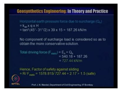
So, if you calculate this then you have to calculate what will be the horizontal earth pressure force due to the surcharge Q h that is, k a b into q into H that is, tan square 45 minus 31 by 2 into 39 q into H is equal to 15 then 187.26 kiloNewton per meter. So, no component of surcharge load is considered so as to, obtain the more conservative solution. So, total driving force F static will be equal to what is, E h plus Q h. So, we have calculated earlier, what is H, that is 540.18 plus 187.26.
