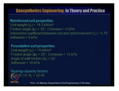
Now, reinforced soil properties unit weight gamma r 18.5 kiloNewton per meter cube, friction angle pi r 33 degree, cohesion 0 kiloPascal, interaction coefficient between soil and the reinforcement that is, C i is equal to 0.75 and adhesion is 0 kiloPascal. So, do not confuse with the interaction coefficient between soil and reinforcement C i and C of r. C r is the coverage ratio that is, the width of the geogrid strip divided by center to center horizontal spacing.
