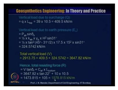
So, we are showing here that, how you have calculated hence, the total resisting force R V tan delta f C a f into L of the bottom. So, this will be 3647.82, this value plus into tan of 22 degree plus 10 into that is, C a f 10 and this into L bottom, 10.5. So, this will give you the total resisting force R is equal to 1578.815 kiloNewton per meter. So, you know that, what should be the total resisting force now, you have to check, what should be the driving force.
