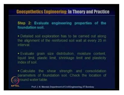
Step 2, evaluate the engineering properties of the foundation soil, detailed soil exploration has to be carried out along the alignment of the reinforced soil wall at every 25 interval. It is necessary to carry out the test, sometimes you can obtain some result without any soil exploration it will be danger. So, it is very important that one should carry out the test along the element of the reinforced soil wall and every 25 meter interval.
