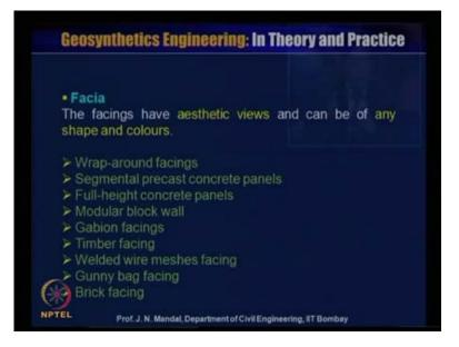
Now, geo textile it may be woven and nonwoven are also used wrap around faced mechanically stabilized earth wall. So, you do not need that any facing element, like the geo grid what you wanted to use this kind of the panel or kind of the block instead, of that in case of the geo textile, where whether it is a woven and nonwoven geo textile you can simply the wrap the face element, so you can construct this wall.
