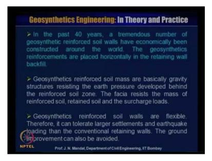
So, in the past 40 years a tremendous number of the geo synthetics, reinforced soil wall have economically been constructed around the wall, the geo synthetics reinforcement are placed horizontally in the retaining wall backfill. Geo synthetics reinforced soil mass are basically gravity structure resisting the earth pressure develop behind the reinforced soil zone, the facia resists the mass of the reinforced soil retained soil and surcharge load.
