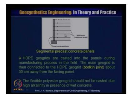
You can see this is a segmental precast concrete block and this is the number of layer of the geo grid material, it may be the high density polyethylene geo grid or non polyester geo grid also. So, here is the segmental precast concrete block this is the block, so high density polyethylene geo grid are casted into the panel during the manufacturing process in the field.
