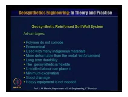
Geo synthetics reinforced soil wall system, it has a advantage because polymer do not corrode, it is economical used with many indigenous materials, more deformable than the metal reinforcement long term durability. The geo synthetics is flexible we can move any direction as you like it. And unskilled labor can place, it you do not need any skilled labor for this and you require minimum excavation, it gives good drainage and heavy equipment is not needed.
