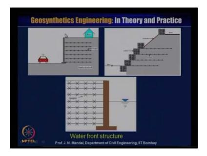
This is the some of the useful use of the reinforced soil retaining wall and when you want to construct a vertical wall, you can provide with the reinforced soil wall and you can construct the building here. So, there will be no problem and the bottom one that there will be a road, the car can pass through this area also when there is a slope you can use this gabion and also the parallel layer of the geo grid reinforced soil retaining wall.
