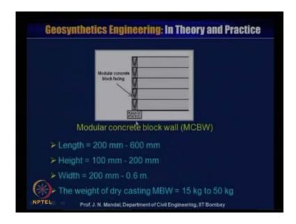
Now, this modular concrete block wall, so this is the modular concrete wall facing and this is the number of the layer of the reinforcement material. And this block has a length about 200 millimeter to 600 millimeter and height is about 100 millimeter to 200 millimeter width is 200 millimeter to 0.6 millimeter and the weight of the dry casting modular block wall is 15 k g to 50 k g.
