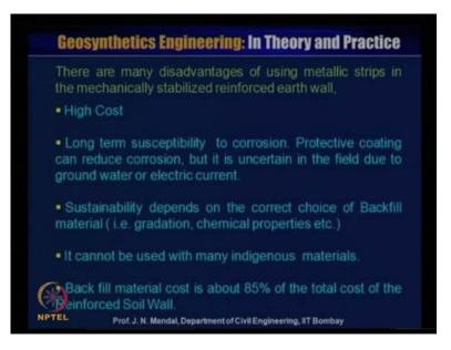
There are many disadvantage of using the metallic strips in mechanically stabilized reinforced earth wall it is high cost, long term susceptibility to corrosion protective coating can reduce the corrosion, but it is uncertain in the field due to the ground water or electric current. Sustainability depend on the correct choice of the backfill material gradation chemical properties.
