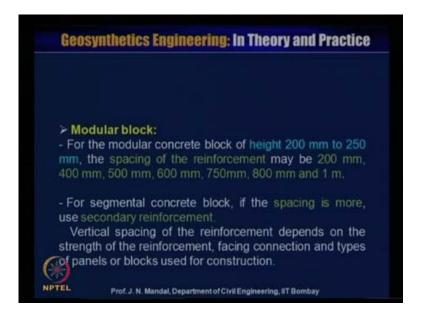
Now, modular block for the modular concrete block of height 200 millimeter to 250 millimeter, the spacing of the reinforcement may be 200 millimeter, 400 millimeter, 500 millimeter, 600 millimeter, 750 millimeter, 800 millimeter and even then 1 millimeter 1 meter. Now, for segmental concrete block, if the spacing is more then you use the secondary reinforcement.
