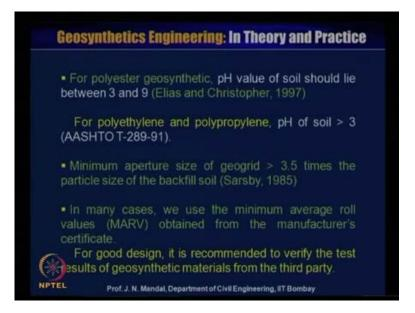
For polyester geo synthetics p h value of soil should lie between 3 and 9, that is Elias and Christopher 1997, for polyethylene or polypropylene p h of soil greater than 3 AASHTO T 2 8 9 9 1. Minimum aperture size of the geo grid should be greater than 3 point 5 times, the particle size of the backfill soil as given by Sarsby 1985, in many cases we use the minimum average roll value m a r v obtained from the manufacturer's certificate.
