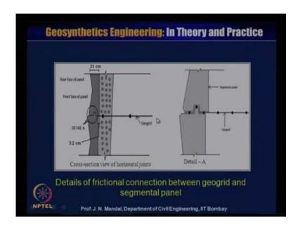
So, more about this you can see here, that cross sectional view of the horizontal joint this is about detail about, And you can see here 3 point 2 centimeter and this is the front face of the panel this is the rear face of the panel and this is 21 centimeter, it is like this you can see detail of the here and this is the geo grid material and this is the segmental panel. So, this is the detail of frictional connection between the geo grid and the segmental panel.
