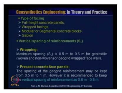
Now, what is the type of facing it may be full height concrete panel, then wrapped facing or modular or segmental concrete block or gabion facing. And you should know the what will be the vertical spacing of the reinforcement s v, if there is a wrapping system, so maximum spacing s v is 0 point 5 meter to 0 point 6 meter for geo textile, it may be the woven geo textile or it may be nonwoven geo textile.
