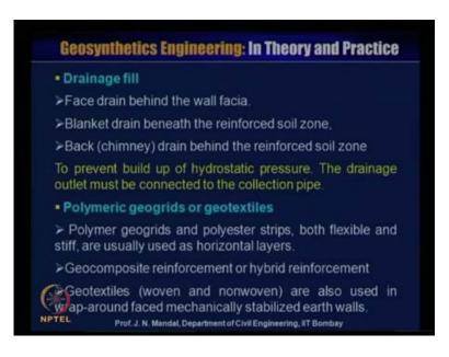
So, you should know that what exactly that kind of the geo grid it is, so that soil this criteria you should satisfy that this what would be the value of c e g, it should be less than 30 meter mol per k g and also at the same time, what will be their molecular weight that greater than 25,000 gram per mol. So, this you can satisfy the criteria that for the
