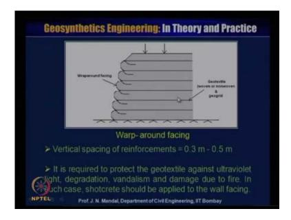
So, vertical facing of the reinforcement generally point 3 to point 5 meter and it is required to protect, the geo textile against the ultraviolet light or degradation vandalism and damage due to the fire. In such case that shotcrete should be applied to the wall facing, here the shotcrete should be applied to the wall facing, this may be the geo textile woven and nonwoven geo textile material, this is wrap around facing.
