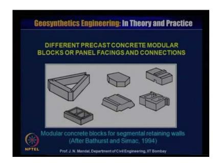
Now, there are different precast concrete modular block or panel facing and connection, you can see this is a some of the modular concrete block for segmental retaining wall after Bathurst and Simac 1994, you can say this is a kind of the block. And you can see that, there is a hole here this is a act as a facing element and this hole is filled up with the aggregate which will act as a drainage.
