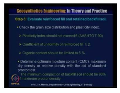
Step 3, evaluate the reinforced fill and retained backfill soil, check the grain size distribution and the plasticity index, plasticity index should not exceed 6 as per AASHTO T 90. Coefficient of uniformity of the reinforced fill should be greater than equal to 2, organic content should be limited to 5 percent and determine the optimum moisture content o m c, maximum dry density or relative density with the aid of standard proctor test.
