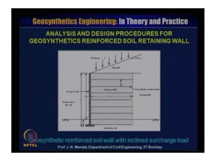
So, now you require further analysis and design reinforced is for geo synthetics reinforced soil retaining wall, these are geo synthetics reinforced soil wall with inclined surcharged load. Sometimes it may be the inclined, sometimes it is not inclined if there is a inclined, then you have to be consider, what will be the surcharge load here you can see key with the surcharge load, which is making at an angle of beta and this is the slope field.
