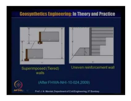
Also superimposed or tiered wall, you can construct one wall and then make a slope and make the another wall, it is superimposed or it is called the tiered slope and this also uneven unreinforced soil wall. You can see that the length of the reinforcement is less, then gradually increasing like this little bit trapezoidal inset and this is the depth of the embankment and this is after f h w a n h I 1 0 0 2 4 2009, so different types of the systems of reinforced soil wall can be constructed.
