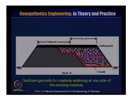
also the geo foam or geo cell for roadway widening on one side if you want this is the existing road and if you want it to widening on the other side of the road. So, this is the new road by you can include the geo cell or the geo foam material.
