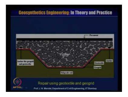
You can excavate and you can provide with the geo grid or the geo textile material and you can anchor, the geo grid and geo textile and then you filled up with the stone and then you can provide with the pavement on the top.
