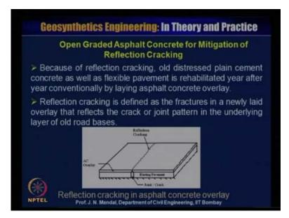
Now, I will address open Graded Asphalt Concrete for Mitigation of Reflection Cracking you know, because of reflection cracking the old distressed plain cement concrete as well as flexible pavement is rehabilitated year after year conventionally by laying asphalt concrete overlay. Reflection cracking is defined as the fracture in a newly laid overlay that reflect the crack or the joint pattern in the underlying soil of old road bases.
