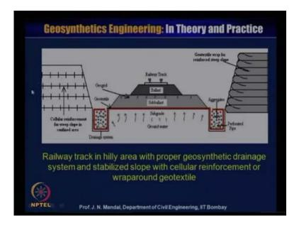
This is another this railway track in the hilly area with proper geo synthetics drainage system and stabilized slope with cellular reinforcement, one side you can go for the cellular reinforcement, you can also provide with the wrap around geo textile. So, we will discuss later how we will design the wrap around geo synthetics material here, so this is another system where you can use the different system.
