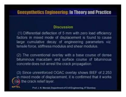
So, this factor also important, so from this what we can discuss, the differential deflection of 5 millimeter with 0, load efficiency factor in mixed mode of displacement is found to cause large cumulative decay of engineering parameters, that is tensile force stiffness modulus and shear modulus. Second, the conventional overlay with the base course or dense bituminous macadam and surface course of bituminous concrete does not arrest the crack propagation.
