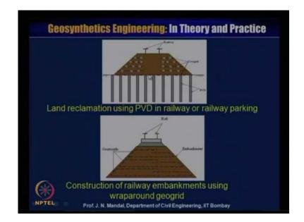
This is land reclamation using the p v d in railway, so where this is the p v d has been installed and then on the top of the then embankment has been constructed and railway can be pass through, this kind of the embankment. This construction for the railway embankment using the wrap around geo grid, you can wrap around the geo grid and construct the slope and the railway line can be passed through this.
