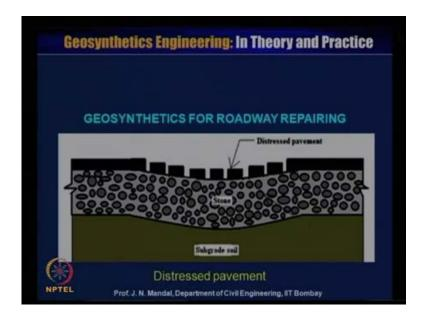
So, here this geo synthetics for the roadway repairing, you can see this is a distressed pavement this is the stone, this is the distressed pavement and how you can rectify this distressed pavement.
