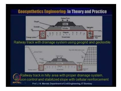
You can see some railway track in the hilly area, here is the hilly area with the proper drainage system and you can see one side, that it is a hill you can provide with the kind of the cellular reinforcement. And if the space is a shortage, so you can length can also be reduced or if there is any mountain and space is not enough, so we can provide with the cellular reinforcement.
