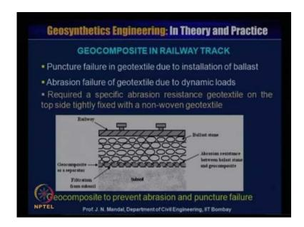
Now, geo composite in railway track, puncture failure in geo textile due to installation of the ballast, abrasion failure of geo textile due to dynamic load. Require a specific abrasion resistance geo textile on the top side of the tightly fixed with the nonwoven geo textile material. So, this is I mentioned that how also the geo composite material also can be prevent the abrasion and the puncture failure.
