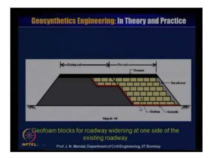
And geo foam block roadway widening at one side of the existing road, if the situation is like this where you can place the geo foam, it is very easy to place the geo foam and you can widening and then you fill up with the soil and the grass can grow. So, you can make a new road.
