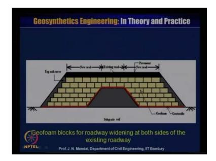
Also geo foam block on the roadway widening at both the side of the existing with existing road, then you can road the new road you can provide with this here like this, so you can use it.
