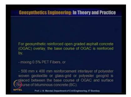
Now, for geo synthetics reinforced open graded asphalt concrete which we designated here OGAC overlay, the base course of the open graded asphalt concrete is reinforced by mixing. The point 5 percent pet fiber or 500 millimeter into 400 millimeter reinforce interlayer of polyester woven geo textile or glass grid or polyester geo grid is placed between the base course of the open graded asphalt concrete and surface course of bituminous concrete or which we call b c.
