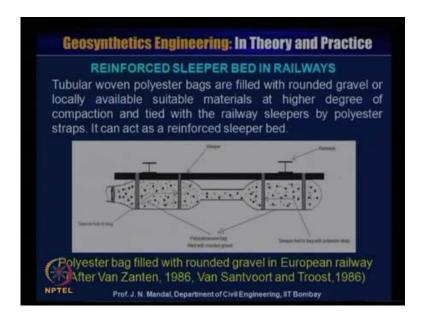
Here that reinforcement sleeper bed in the railway tubular this is the polyester bag filled with the rounded gravel in European railway, after van zanten 1986 van santvoort and troost 1986, this is tubular woven polyester bag are filled with the rounded gravel or locally available suitable material at a higher degree of compaction and tied with the railway sleeper by polyester strap.
