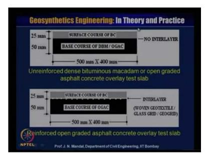
So, here you can see that unreinforced dense bitumen macadam or open graded asphalt concrete overlay test slab, this is about 500 millimeter to 400 millimeter and no interlayer, this is the base course of d b m and o g a c and this is the surface course of b c. And this thickness about 50 millimeter base course and surface course is 25 millimeter, so here unreinforced dense bitumen macadam or the open graded asphalt concrete overlay test slab.
