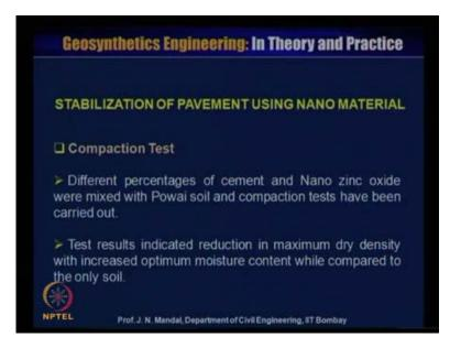
Now, stabilization of pavement using NANO material, this is a you have done the number of the compaction test and different percentage of the cement and the NANO zinc oxide were mixed with the powai soil. And compaction test have been carried out test result indicated, the reduction in maximum dry density with increase of the optimum water content while compare the only soil.
