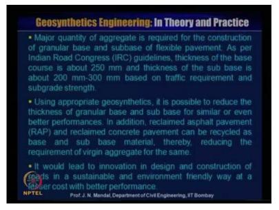
More quantity of aggregate is required for the construction of granular base sub base flexible pavement as per the Indian road congress guideline, the thickness of the base course is about 250 millimeter. And thickness of the sub base is about 200 millimeter to 300 millimeter based on traffic requirement and sub grade strength, using the appropriate geo synthetics, it is possible to reduce the thickness of the granular base and sub base for similar or even better performance.
