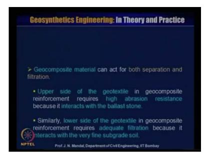
Now, geo composite material can act both separation and the filtration, upper side of the geo textile in a composite reinforcement require high abrasion resistance. Because, it interact with the ballast stone on the other hand, similarly lower side of the geo textile in a geo composite reinforcement require adequate filtration, because it interact with the very fine sub grade soil you can see here.
