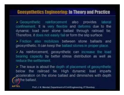
Which can provide you the confinement effect lateral confinement effect and it is very flexible and deform due to the dynamic load, over the stone ballast through rail road tie therefore, it does not easily fail to or from the slip surface, filtration also mobilize
