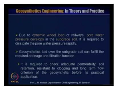
Now, due to the dynamic wheel load of the railway pore water pressure developed in the sub grade soil, it is required to dissipate the pore water pressure rapidly the pore water pressure may be moved upward or due to the dynamic wheel load of the railway then there will also a development of the pore water pressure on the sub grade. So, it is very much essential that how you can dissipate the pore water pressure rapidly.
