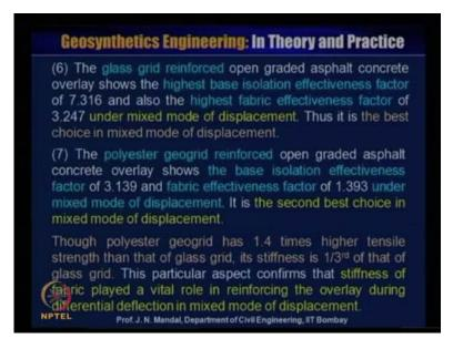
Six, the glass grid reinforced open graded asphalt concrete overlay show the highest base isolation effectiveness factor of 7 point 3 1 6 and also be the highest fabric effectiveness factor of 3 point 2 4 7 under mixed mode of displacement. Thus it is the best choice in the mixed mode of displacement, you can see that how the glass grid will be the more effective, because this isolation effectiveness factor is more compare to the other material.
