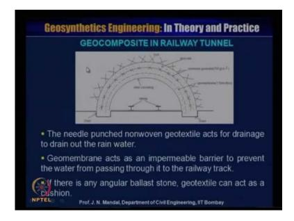
This geo composite also in the railway track, this is a kind of the tunnel where inside the tunnel these this is a railway line, so needle punched nonwoven geo textile here act as a drainage to drain it out, the water and geo membrane you are placing here, where geo membrane will act as a impermeable barrier to prevent, the water from passing through it to the railway track. So, it is therefore, that any angular ballast stone with geo textile can act as a cushion.
