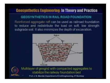
Now, geo synthetics railroad foundation you can see that this is a multi layer of the geo textile with compacted aggregate to stabilize the railway foundation, where reinforcement aggregate raft can be used as a railway foundation to reduce. And the redistribute, the load on the soft low strength sub grade soil, you go for the mat which is very expensive, alternative to that you can provide with the multilayer of geo grid with compacted that aggregate to stabilize the railway foundation bed.
