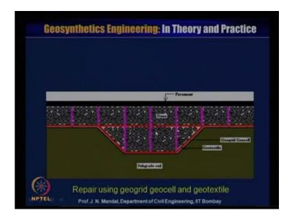
Also you can repair using the geo grid, geo cell this is the geo grid geo cell and this is made of the geo grid or it may be the geo cell all combination, you can see this is the geo cell and this filled up with the stone. And there will be there will be no lateral also the deformation, it very give very good confinement effect or you can repair this kind of the problem using the geo grid, geo cell or geo textile.
