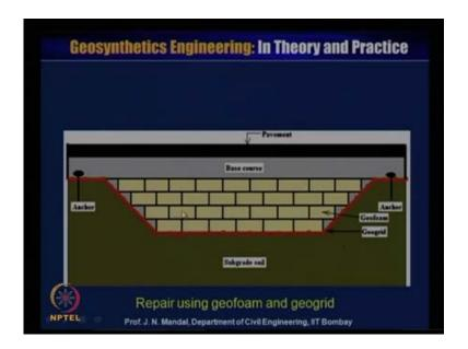
You can also use the geo textile, which can be anchored and then you can place this geo foam material on the top of this is as a base course drain and then the pavement.
