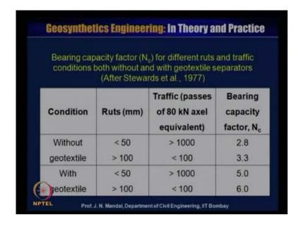
So, this table gives that condition rut and the traffic, and what will be the bearing capacity factor, we will calculate the bearing capacity factor using this table, depending upon the rut traffic and number of the passage. So, bearing capacity factor N c for
