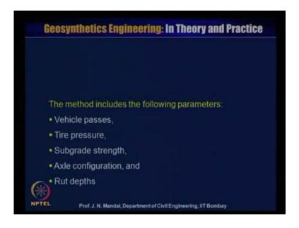
This method includes the following parameter, vehicle passage, what will be the tire pressure, what will be the sub-grade strength, what will be the axle configuration and rut depth.
