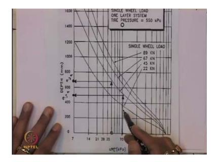
So, here is the design chart for the calculation, for the thickness of the aggregate, this is single wheel load one layer system tire pressure 550 kilopascal, and this is under the various load 22 kilo Newton, 45 kilo Newton, 67 kilo Newton and 89 kilo Newton this is single wheel load. In our problem we have considered it only single wheel load is 40 kilo Newton that means, we will consider in between these two load 22 kilo Newton and the 45 kilo Newton.
