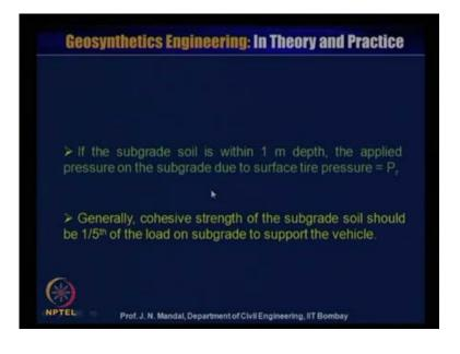
So, if the sub-grade soil is within 1 metre depth. the applied pressure on the sub-grade due to the surface tire pressure P r, generally cohesive strength of the sub-grade soil should be 1 5th of the load on sub-grade to support the vehicle.
