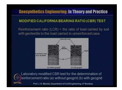
Now, this is modified California bearing ratio test, this we call that reinforcement ratio or LCR, is the ratio of load carried by the soil with geotextile to the load carried in unreinforced case. Here, laboratory modified CBR test for determination of reinforcement ratio without geogrid and with geotextile are shown, this is without geogrid and this is the soil, and this is at a particular moisture content, and the in situ density.
