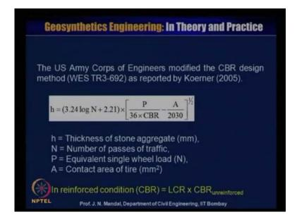
So, this is given by u s army corps of engineer modified the CBR design method, WES TR3-692 as reported by Koerner, 2005, so this is the equation. So, h is equal to 3.24 log N plus 2.21 into P divided by 36 into CBR minus A divided by 2030 whole to the power half, where h is the thickness of the stone aggregate in millimetre. N is the number of the passage of traffic and P is the equivalent single wheel load that is Newton, and A is the contact area of the tire.
