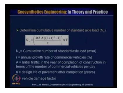
Now, determine the cumulative number of standard axle load N s, so you have to what will be the standard axle load with this equation, N s is equal to 365 A into 1 plus r to the power n minus 1 divided by r into F, where N s is the cumulative number of standard axle load, that is msa. And that A is equal to initial traffic in the year of completion of the construction, in terms of the commercial vehicle per day.
