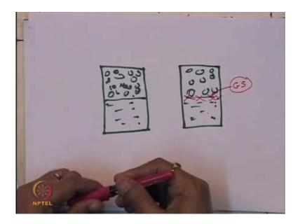
So, let us say this is the mould and the lower part is the soil, and upper part is the aggregate layer, and in case of the reinforcement lower part is the soil and upper part is the aggregate layer. And in between here we are placing this geosynthetics material, now you the soil is at the bottom, aggregate is at the top, so when you apply the load and you measure the what should be the deflection.
