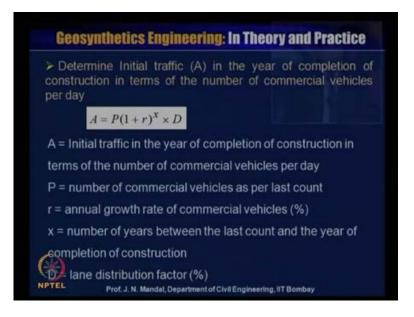
Next determine the initial traffic that means, A in the year of completion of the construction in terms of the number of commercial vehicle per day. So, this is the equation given by the code A is equal to P into 1 plus r whole to the power x into D, A is the initial traffic in the year of completion of construction, in terms of the number of the commercial vehicle per day.
