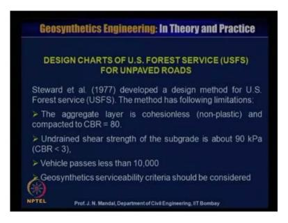
Now, I will address the design chart of US forest service, USFS for unpaved roads, Steward et al, 1977 developed a design method for US forest service, this method has the following limitation. The aggregate layer is cohesionless non plastic and compacted to CBR is equal to 80, undrained shear strength of the sub-grade is about 90 kilopascal or CBR less than 3, vehicle passage less than 10000, geosynthetics serviceability criteria should be considered.
