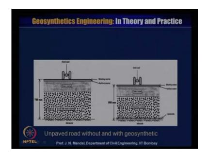
Here, just shows this diagram for the unpaved road without and with geosynthetics road, when the with without geosynthetics this thickness of the pavement is 700 millimetre,
