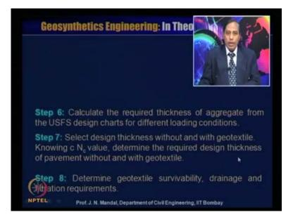
Step 6, calculate the required thickness of aggregate from the USFS design chart of different loading condition. Step 7 select the design thickness without and with geotextile, knowing the value of C into N c value, determine the required thickness of pavement without and with geotextile. Step 8 determine geotextile survivability drainage and the filtration requirement.
