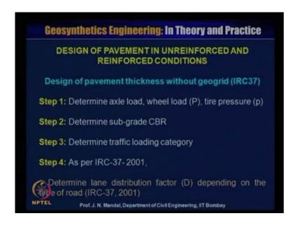
Design of pavement thickness without geogrid as per IRC 37, step 1 determine the axle load wheel P and tire pressure P, step 2 determine the sub-grade CBR value, step 3 determine traffic loading category. And step 4 as per IRC-37-2001, determine the lane distribution factor D depending upon the type of the road as per IRC 37 to 001
