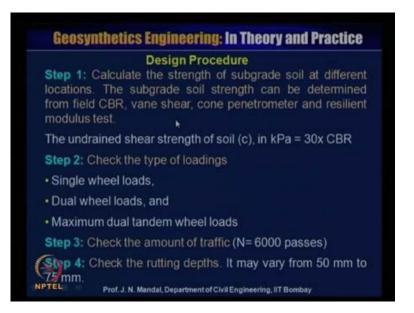
So, this is the procedure step 1, that calculate the strength of the sub-grade soil at different location, this sub-grade soil strength can be determined from the field CBR, vane shear, cone penetrometer and resilient modulus test. So, when you can calculate the what should be the CBR value, then you can calculate also undrained shear strength of the soil C is equal to 30 into CBR, that is in terms of kilopascal.
