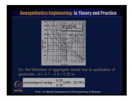
So, thickness of the aggregate saved due to application of geotextile, that is delta h will be equal to 700 millimetre minus 500 millimetre or 0.7 minus 0.5 is equal to 0.20 metre. So, that means, percentage of saving is about 0.2 by 0.7 into 100 that 28.58 percentage, so you are saving about 28, 29 percentage is saving. So, very good amount of aggregate you are saving, when you are using this geosynthetics material as a separation.
