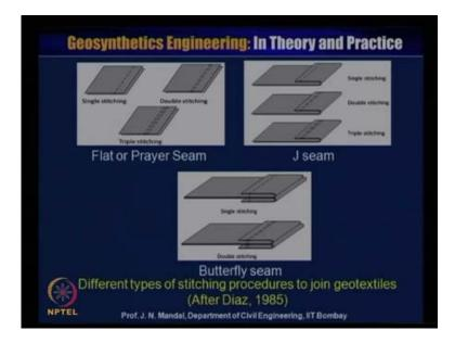
And here, the different types of the stitching procedure to join the geotextile material, after Diaz, 1985 you can say flat or prayer seam this is a single stitching, double stitching, triple stitching. Or J seam with a single stitching, double stitching and triple stitching and to also butterfly seam, it is a single stitching and the double stitching.
