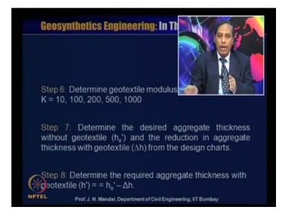
Step 6 they determine the geotextile modulus, I say modulus value may be 10, 100, 500 and 1000 kilo Newton per meter, step 7 determine the desire aggregate thickness without geotextile h 0 dash, and reduction in aggregate thickness with geotextile delta h from the design chart. Step 8 determine the required aggregate thickness with geotextile that is h dash will be equal to h 0 dash minus delta h, and h 0 dash is equal to aggregate thickness with geotextile.
