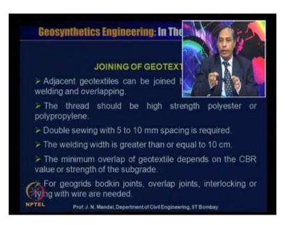
Now, adjacent geotextile can be joined by stitching, sewing, welding and overlapping, the thread should be high strength polyester or polypropylene, double sewing with 5 to 10 millimeter spacing is required. The welding width is greater than or equal to 10 centimeter, minimum overlap geotextile depend on the CBR value or strength of the subgrade soil, for geogrids bodkin joint, overlap joint, interlocking or tying with the wire are needed.
