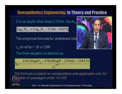
So, for rut depth other than 0.075 the N s is modified by log 10 N s tends to log 10 N s minus 2.34 r minus 0.075, the empirical formula of undrained cohesion C u in kilo Pascal is equal to 30 into CBR. So, you can obtain the final equation derived at h 0 dash is equal to 119.24 into log N p plus 470.98 log P minus 279.01 r minus 2283.34 divided by C u to the power 0.63. So, this formula is based on extrapolation and applicable only for the number of the passage under 10000.
