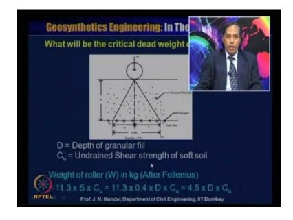
Now, what will be the critical dead weight of vibro-roller, so here this is the weight of the roller W in K g, this is after Fellenius and this is a depth of the granular fill, so this is a granular fill and this is the geosynthetics material. And this is 0.8 times of the D and this is distance S, this distance is S and D is the depth of the granular fill, and C u is the undrained shear strength of the soil.
