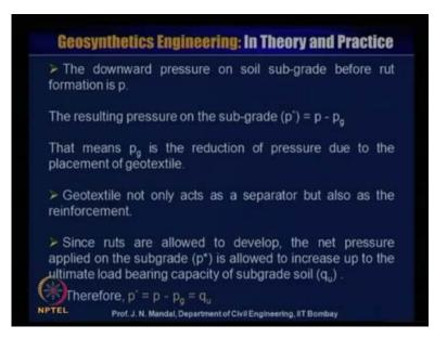
Now, downward pressure on soil sub-grade before rut formation is p, the resulting pressure on the sub-grade p star will be equal to p minus p of g.
