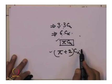
Now, Barenberg and also van den has given that rut begin at 3.3 C or what you call C of u without geosynthetics material, and with the geosynthetics material this value is 6 into C u. So, Barenberg and van den have performed number of the filters with and without geosynthetics material, and this is much more realistic value that without geotextile material rut begin at 3.3 into C u and with geotextile material rut begins at 6 of C u.
