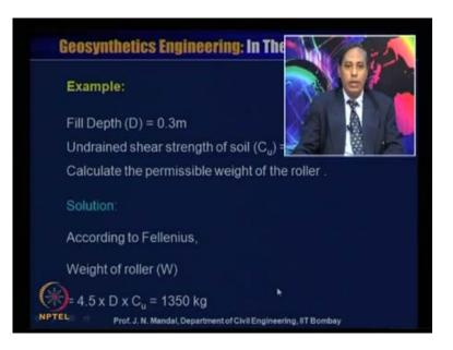
Giving one example that full depth D is equal to 0.3 meter, undrained shear strength of the soil C u is equal to 1000 K g per meter square, so calculate that what will be the permissible weight of the roller. So, here is the solution according to the Fellenius equation, the weight of the roller W is equal to 4.5 D into C u, so you substitute value of D 0.3, C value is 1000 K g per meter square, so this will give you that 1350 K g; so weight of the roller will be the 1350 K g.
