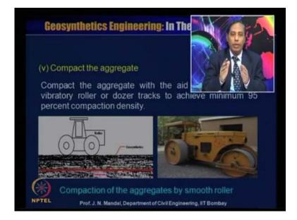
And then, compact the aggregate, compact the aggregate with the aid of smooth drum vibratory roller or dozer tracks to achieve the minimum 95 percent is compaction density. You can see this is the roller which we can use for the compaction, this is the compaction
