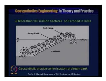
You can see here geosynthetics erosion control system at a stream blanket, where this geosynthetics material has been placed, this is the sand bed geosynthetics material has been placed. And this is the rap, and this is the rock riprap material placed on the top of the geosynthetics material, and more than hundred million hectare of soil eroded in India, you think about that quantity of the soil is eroded in India.
