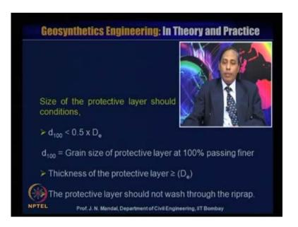
So, this will act as a protective layer for riprap installation, it is also important the size of the protective layer, should satisfy the following condition that is d 100 should be less than 0.5 into D e. D 100 is the grain size protective layer at 100 percent passing finer, and thickness of the protective layer should be greater than equal to D e, so protective layer should not wash through the riprap.
