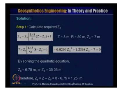
Now, solution step one calculate required z 0, so we have to use this equation z d is equal to z 0 to 1.48 by r z minus z 0 plus 1, we know z is equal to 8 metre r is equal to 50 metre z d is equal to 7 metre. So, you substitute this value that is z d which we calculated earlier that is 7 metre is equal to z 0 1.48 by r, r is 50 metre into z, z is equal to 80 metre minus z 0 plus 1.
