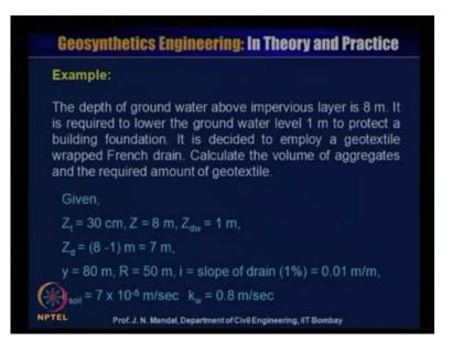
Next, I will explain the one example, the depth of the ground water above the impervious layer is 8 metre, it is required to lower the ground water level, 1 metre to protect a building foundation. It is decided to employ a geotextile wrapped French drain, calculate the volume of the aggregate and the required amount of geotextile.
