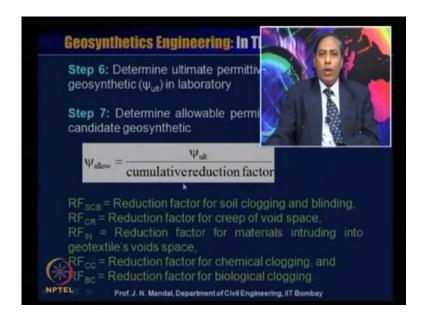
Step 6 determine the ultimate permittivity of the candidate geosynthetics, psi ultimate in laboratory, step 7 determine the allowable permittivity of the candidate geosynthetics, so psi allowable will be equal to psi ultimate by cumulative reduction factor. So, this cumulative reduction factor, it may be due to reduction factor for SCB; that means, reduction factor for soil clogging and blinding.
