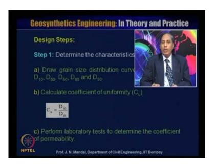
So, you can make a grain, so some design step, step 1 determine the characteristics of the field soil a draw the grain size distribution curve, and calculate all this D 10, D 50, D 60, D 85, D 90. Calculate coefficient of uniformity, that is C u is equal to D 60 by D 10 c perform laboratory test to determine the coefficient of permeability.
