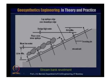
Here, also stream bank revetment you can see this is geotextile you should place the stone upslope, and also you can join with the some securing pin. So, you can place it this is the high water level, and how you can protect the stream bank revetment by using this geosynthetics material.
