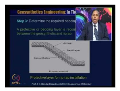
Step 3 determine the required bedding, so if this is the subgrade this is the erosion control let it problem, we are placing this geosynthetics material here, so you need a protective layer between the geosynthetics and the riprap. Otherwise, the geosynthetics material if you place directly, the stone armour stone on the geosynthetic material then geosynthetics material may tear up or damage.
