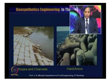
You can see some places slope or channel, where it has been used that prefabricated block, but you can see how it fell, you can use also the hard armour near to the sea shore to protect the sea from the erosion. And at the base of these armour stone we should provide proper kind of the geosynthetics material, because there is a development of the excess pore water pressure, and that was the major reason that this kind of the structure fell.
