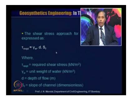
Now, there is a development of shear stress approach for channel, can be also expressed as t required is equal to this is gamma w into d into S f, where T required is equal to required shear stress that is kilo Newton per metre square. Gamma w is unit weight of water kilo Newton per metre cube, and d is the depth of flow in metre, S f is slope of channel is dimensionless, so you can calculate what will be the required shear stress using this equation.
