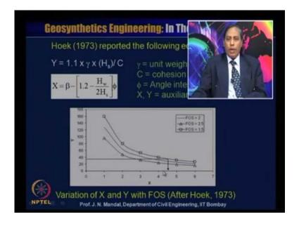
So, you have to calculate what will be the slope angle, now Hoek 1973 reported the following equation, that is y is equal to 1.1 into gamma into H s by C, gamma is equal to unit weight of soil, C is equal to cohesion of the soil, phi is equal to angle of internal friction of the soil. And X is equal to beta minus 1.2 minus H w by 2 H s into phi, for this
