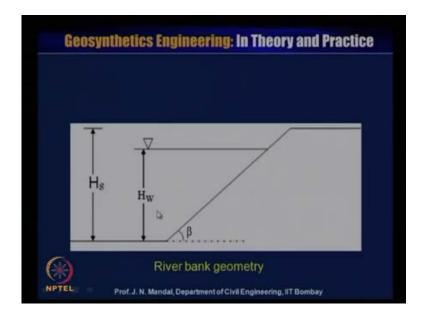
Now, we can see here river bank geometry, this is height of the slope H s, this is angle beta this is the water level height is H w and this is the solution.
