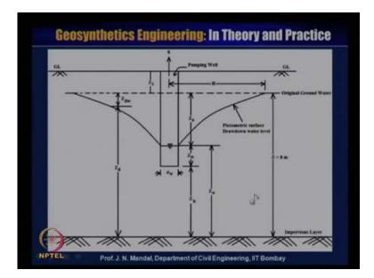
Here it is given z of t is 30 centimetre, and z this is 8 metre and z of w, so this d of z is 8 metre, and z of d w is 1 metre, so z of d here to here z of d will be equal to z 8 metre by z d w is 1 metre. So, z of d will be z 8 metre by z d w 1 metre, so z d will be equal to 8
