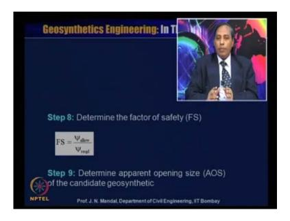
Step 8 determine the factor of safety, so factor of safety will be equal to psi allowable by psi required, step 9 determine apparent opening size that mean AOS of the candidate geosynthetics. So, this we require for the design, so when you will design you should follow up all the step, you have take care about the flow related problem, you have to take consideration of the apparent opening size of the geosynthetics material or the equivalent opening size of the geotextile material.
