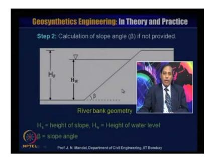
Then step 2 calculation of slope angle this is beta you have not provided, so this is a 1 river bank geometry, and this is the height of the slope, and this is the height of the water level and this angle is beta.
