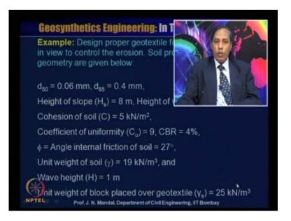
This one example design proper geotextile for placing at a river bank in view to control the erosion, soil properties and the river bank geometry are given, and these are the data is given D 50 is 0.06, millimetre, D 85 0.4 millimetre. This we can have grain size distribution curve of the soil, height of the slope let us say H s is equal to 8 metre, height of the water level H w is equal to 5 metre.
