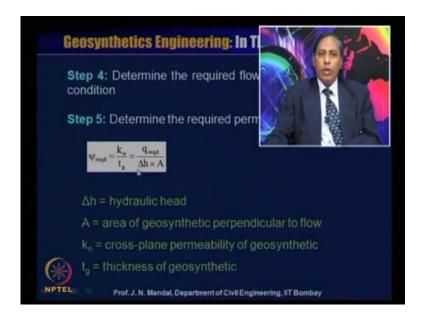
Step 4 determine required flow rate, q require in the field condition, step 5 determine the required permittivity psi required, so psi required you know the equation that is k n by t g
