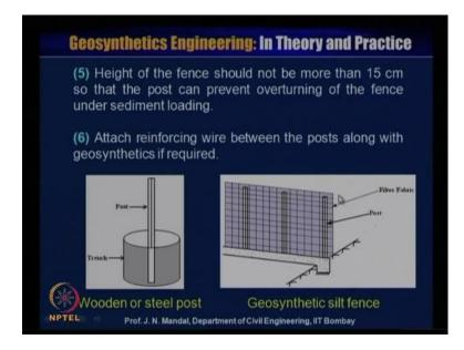
So, this backfill material provided and this you necessary for the anchoring. Next height of the fence should not be more than 15 centimeter. So, that post can prevent overturning
