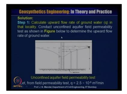
Now, the same I say the capillary migration break using geo textile under roadway and first of all that step 1, you have to calculate the upward flow water of ground water in the
