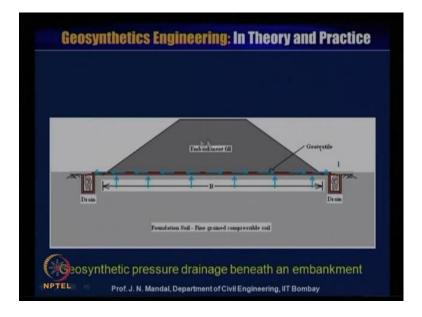
This is the embankment and geo synthetic is placed, here and this is the B and this is the foundation soil fine grained, compressible soil. So, there is a development of the pressure on the geo synthetic material and this is the drain, you can see that how the water is passing along the plane of the geo synthetic material through the drainage.
