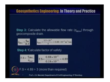
So, this is q required is 0.18 into 10 to the power minus 4. So, this will give you the factor of safety 4.89. So, factor of safety is equal to 4.89 it is greater than 3. So, it is more than required. So, it satisfy the criteria. So, here you see that how that that geo composite material have been used and it is the design is based on the flow related. So, you remember, when it is a not in the laminar flow condition, then you have to design
