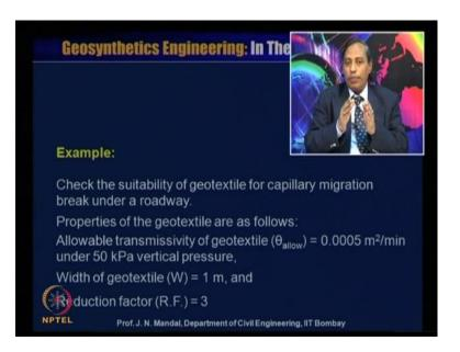
Here, I am giving one simple example, check the suitability of the geo textile for capillary migration break under a roadway. So, properties of the geo textile is given, let us say allowable transmissivity of the geo textile theta allowable is equal to 0.0005 meter square per minute, are under a 50 kilopascal vertical pressure, width of the geo textile W is equal to 1 meter and reduction factor is equal to 3.
