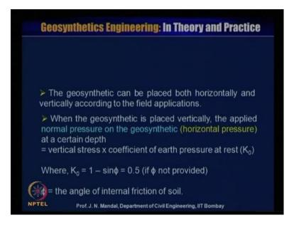
The geo synthetic can be placed both horizontally and vertically according to the field
