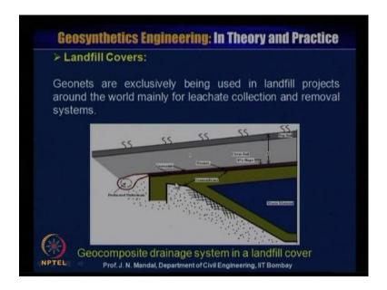
And landfill cover, this is geo net are exclusively being used in the land fill project around the world mainly for leach ate collection and removal system. So, here geo composite drainage system is shown in a landfill cover on the top, this is the landfill and this is the all waste material and on the top of that you have to provide with the geo composite material, that is geo net and then laminated with geo textile material, it is top and bottom is geo textile and this is geo net material.
