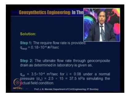
So, now the solution now step 1, we require flow rate is provided; that means, q required is 0.18 into 10 to the power minus 4 meter cube per second. Step 2, you ultimate flow rate through the geo composite drain as determine in the laboratory is given that q ultimate is equal to that is 3.5 10 to the power minus 4 meter cube per second for i is equal to 0.8 under a normal pressure sigma n is equal to 37.5 kilopascal, simulating the actual field condition.
