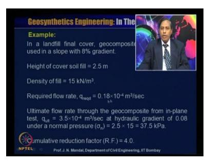
So, this also we have calculated earlier this is q required is 0.18 into 10 to the power minus 4 meter cube per second.
