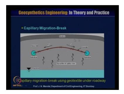
Next, the capillary migration break, we can see that most of the time in the roadway, you can see it is a clay soil and this water level is here and there is a upward flow of capillary water, sometime water can move beyond the roadway and water is stagnant that is due to the upward flow of the capillary water. So, what we do in general, we provide with the drainage somewhere here.
