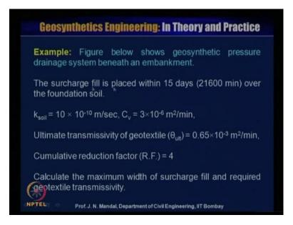
So, in this problem the surcharge fill is placed within 15 days; that means, 21600 minute over the foundation soil and coefficient of permeability soil is given, 10 into 10 to the power of minus 10 minute per second. And coefficient of consolidation C v is given equal to 3 into 10 to the power minus 6 meter square per minute, ultimate transmissivity of the geo textile is given theta ultimate is equal to 0.65 10 to the power minus 3 meter square per minute.
