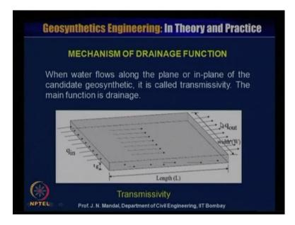
Next, mechanism of drainage function you know that, when the water flow along the plane or in-plane of the candidate geo synthetics, is called transmissivity. The main function is the drainage or which we call the transmissivity.
