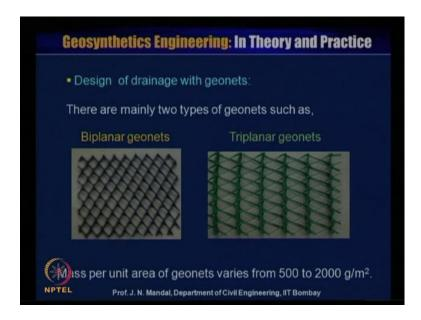
Next design of drainage with the geonets. So, let us discuss that design of drainage with geo net, there are mainly two type of the geo net, that is one is the bi planar geo net and another is the tri planar geo net. So, you can see this is a kind of the bi planar geo net material, you can see this is rhombus in shape and if there is any flow quantity is more then you can use the bi planar geo net material or if the quantity of more and more then you can use tri planar geo net.
