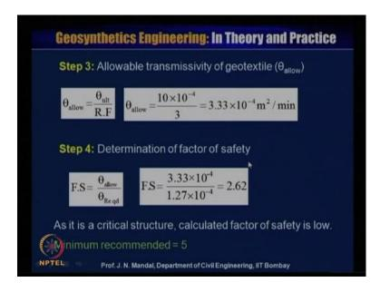
Now, step 3 allowable transmissivity of geo textile that is theta allowable. So, theta allowable will be theta ultimate by reduction factor. So, theta allowable you know that theta ultimate value 10 into 10 to the power minus 4 and reduction factor is given 3. So, theta allowable will be equal to 3.3 into 10 to the power minus 4 meter square per minute.
