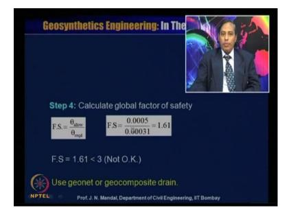
Step 4, calculate the global factor of safety, that mean factor of safety is equal to theta allowable by theta required. So, factor of safety you know what is theta allowable 0.0005 and this divided by theta require 0.00031 which we know earlier, what is theta require. So, you can calculate the factor of safety this is 1.61. So, factor of safety is equal to 1.61 on the lower side, it is less than three. So, it is not ok.
