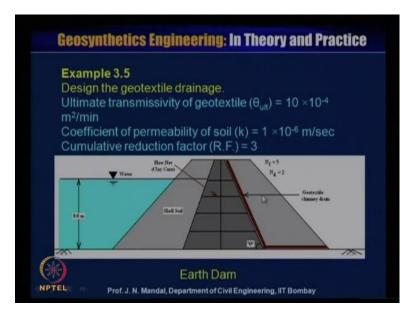
So, this is a earth dam and ultimate transmissivity of this geo synthetics material given 10 into 10 to the power minus 4 meter square per minute and coefficient of permeability of the soil k is 1 into 10 to the minus 6 meter per second and cumulative reduction factor is 3. So, in the core, this is a clay core. So, you can draw a flow net diagram and this angle is 70 degree and this height is about 8 meter.
