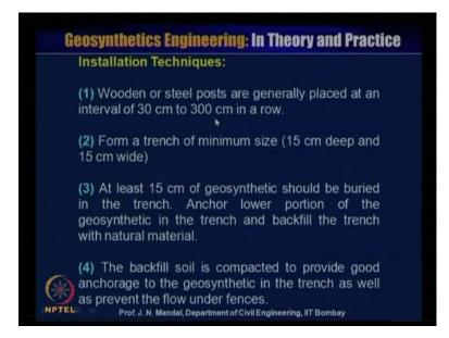
Next at least 15 centimeter geo synthetics should be buried in the trench. Anchor lower portion of the geo synthetics in the trench and backfill the trench with natural material. Here, to be buried it geo synthetics material, the backfill soil is compacted to provide good anchorage to the geo synthetics in the trench as well as prevent the flow under fences.
