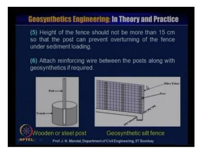
These is the wooden or the steel post can be placed at a interval of 30 to 300 centimeter
