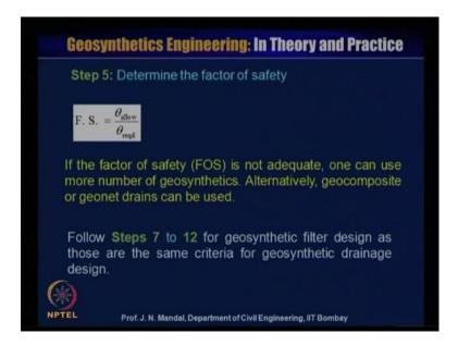
Step 5, determine the factor of safety. So, factor of safety will be equal to theta allowable by theta require, if the factor of safety is not adequate, one can use more number of the geo synthetic material, alternatively geo composite or geo net drain can be used. So, in our permittivity problem, filtration problem you can follow the step 7 to 12 geo synthetic filter design, as those are the same criteria for geo synthetic drainage design.
