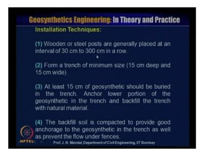
Now, how to install this system. Now, I will explains installation technique of silt fences, the wooden steel posts are generally placed at an interval of 30 centimeter to 300 centimeter in a row.
