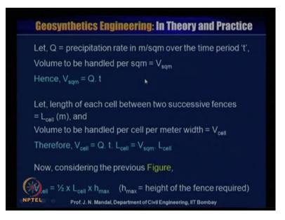
That means, this will be equal to this; that means, this will be equal to this, this is the volume to be handled per cell meter; that means, V square meter into L cell this will be equal to that what should be the V cell here half into L cell into h maximum. So, that was the area and h is the height of the fence required.
