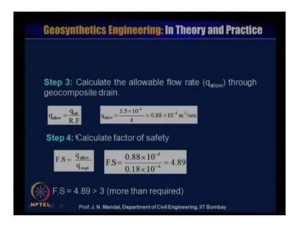
Step 3, calculate the allowable flow rate q allowable through the geo composite drain. So, q allowable will be q ultimate by reduction factor, q ultimate is 3.5 into 10 to the power minus 4. So, q ultimate 3.5 into 10 to the power minus 4 this reduction factor is 4. So, q allowable will be 0.88 into 10 to the power minus 4 meter cube per second. Step 4, calculate the factor of safety.
