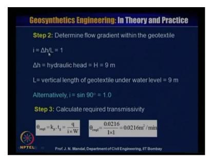
Now, step 2 determine the flow gradient within the geo textile here, i is equal to delta h by L; that means, it will be 1 and delta h is equal to hydraulic head H is equal to 9 meter, L is equal to vertical length of the geo textile under water level is equal to 9 meter. Now, alternatively we can also write i is equal to sin 90 degree is equal to 1.0.
