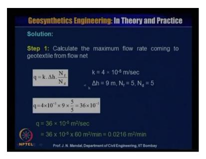
Now, the solution step 1, calculate the maximum flow rate coming to the geo textile from
