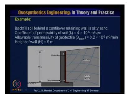
Now, this is another example, this is the backfill soil behind a cantilever retaining wall is silty sand and coefficient of permeability of the soil is 4 into 10 to the power minus 5 meter per second, allowable transmissivity of geo textile theta allowable is given 0.2 into 10 to the power minus 3 meter square per minute, height of the wall is 9 meter. So, here you can see that again you can draw the flow net diagram you find out what is N f and N d that is equal to the 5.
