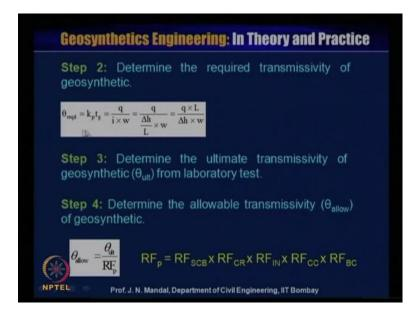
Step 2, you can determine the record transmissivity of geo synthetic. So, earlier we discussed with the permittivity now, it is transmissivity of the geo synthetics this equation also known theta require into k p into t g is equal to q L by delta h into w. Step
