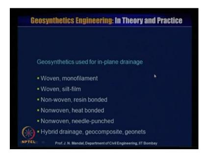
Now, geo synthetics used for in-plane drainage. So, different types of the material can be used it may be woven monofilament, woven silt film, nonwoven resin bonded, nonwoven heat bonded, nonwoven needle punched and hybrid drainage, geo composite and geo nets.
