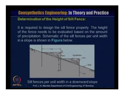
Now, we want to determine the height of the silt fence, it is required to design the silt fence properly. The height of the silt fence need to be evaluated based on the amount of the precipitation. So, this is a schematic of the silt fences, per unit width in a slope as shown. So, this is h of maximum this is L of cell and this is depth and this is the peg and this is the slope and this is the face and this is all precipitation. So, this is the silt fence
