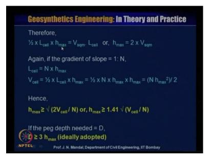
Therefore half into L cell into h maximum is equal to V square meter into L cell.
