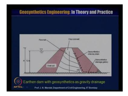
You can see this is an earth dam geo synthetics as a gravity drain, here the geo synthetics as a chimney drain, here geo synthetic drain as a gallery and this is the clay core and you in the clay core you can draw the flow net and you can determine what should be the number of the flow lines and equipotential line and this angle also is known to you suppose, here is 75 degree, this height of the dam is h and this water level is about 12 meter, this is as showing one of the example like that.
