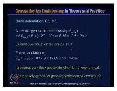
So, we do some back calculation assuming factor of safety is equal to 5, allowable geo textile transmissivity theta allowable will be equal to 5 into theta required; that means, 5 into theta required you know 1.27 into 10 to the power minus 4 that is equal to 6.35 into 10 to the power minus 4 meter square per minute. Now, considering cumulative reduction factor that is 3.
