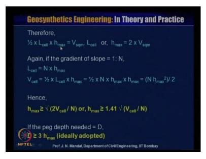
So, from that we can write half into L cell into h maximum is equal to V square meter into L cell or h maximum will be equal to 2 into V square meter. Again if the gradient slope is 1 is to N, for this is gradient slope is 1 is to N for example, if gradients of 1 is there. So, L cell will be N into h maximum. So, V cell will be equal to half into L cell into h maximum then half into N into h maximum into h maximum; that means, N into h maximum square divided by 2.
