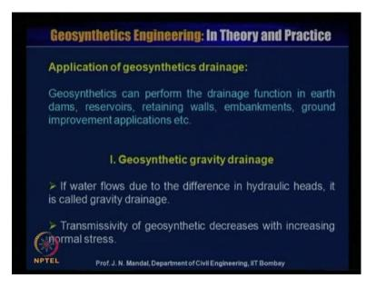
So, application of geo synthetic drainage. Geo synthetic can perform the drainage function in earth dam, reservoir, retaining wall, embankment, ground improvement application etcetera. Now, first I am expressing the geo synthetics gravity drainage. If the water flows due to the difference in the hydraulic head, it is called the gravity drainage. Transmissivity of geo synthetic decreases with increasing the normal stresses, you know this we have already discussed earlier.
