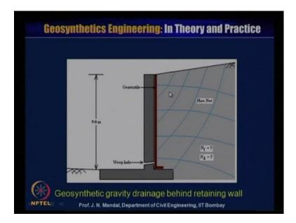
Similarly, geo synthetic gravity drainage behind the retaining wall, what you can use, you can see this is the retaining wall there is a weep hole and geo textile material is placed, just behind the retaining wall. So, whatever water will flow this will go vertically downwards and then passes through the weep hole.
