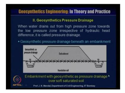
Now, we discuss geo synthetics pressure drainage, when water drains out from high pressure zone towards the low pressure zone irrespective of hydraulic head difference, it
