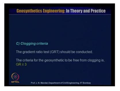
Also you should satisfy the c clogging criteria; that means, gradient ratio test have to be
