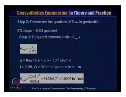
Now step 2, determine the gradient of flow in the geo textile, here it is given the 8 percent slope that is equal to 0.08 gradient. Step 3, required transmissivity that is theta required, theta required will be q by i W and q is equal to flow rate which we calculated here q 2.5 into 10 to the power minus 5 meter cube per minute.
