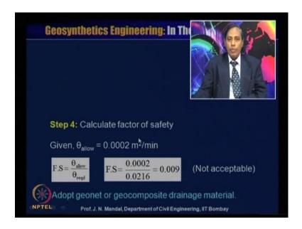
Now, step 4 calculate the factor of the safety, it is given theta allowable 0.0002 meter square per minute. So, factor of safety will be theta allowable by theta required, that mean factor of safety will be equal to 0.0002 divided by 0.0216 is equal to 0.009. So, we can see factor of safety is very, very less, so not acceptable. So, in that case we can adopt the geo net or geo composite drainage material.
