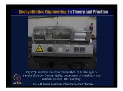
So, this you can see, this is the injection mould for the preparation of ASTM type V sample and this is also central facility for department of metallurgy and material science IIT, Bombay.
