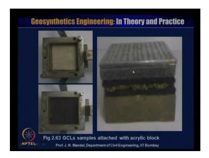
This you can see that figure, this is the geosynthetics clay liner sample, it is attached with the acrylic block and this is the direct shear test machine.
