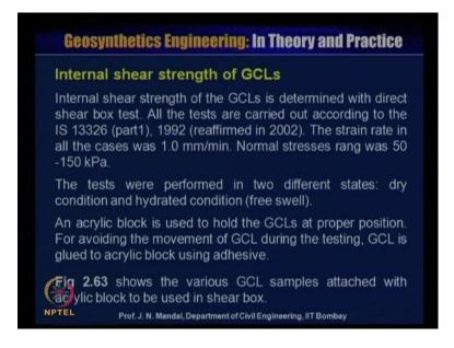
Now, internal shear strength of the GCL is determined with direct shear box test, all the test are carried out according to the IS 13326 part 1 1992 reaffiliated in 2002. The strain rate in all cases was 1 millimetre per minute, normal stresses range from 50 to 150 kilo Pascal. The test was performed in two different state, dry condition and hydrated condition, that is free swell.
