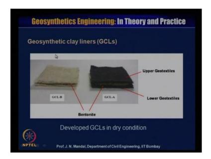
So here, we have developed two kind of the geosynthetics clay liner, one geosynthetic clay liner A, another geosynthetic clay liner B and you can see, this is the geosynthetic
