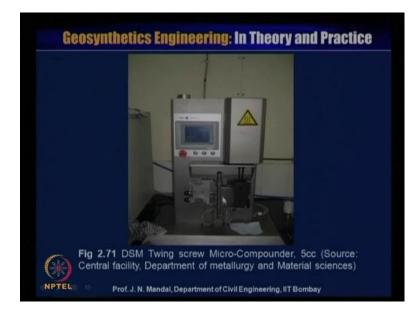
So, this is the DSM Twing screw micro compounder, this is the source from the central facility of the department of metallurgy and material science.
