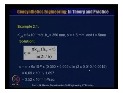
Now, I am giving one typical example where, k of gcl is equal to 6 into 10 to the power minus 11 meter per second, h W is 350 millimetre, b is 1.5 millimetre and t is 5 millimetre. Now, this is the equation q you know now, if you substitute this value then q will be equal to pi into this is k gcl is 6 into 10 to the power minus 11 into h W, h W is 0.350 in meter and then this is the t, t is 5 meter that mean, plus 005, this divided by ln into 2 into t, 2 into that is the t, that is 0.010.
