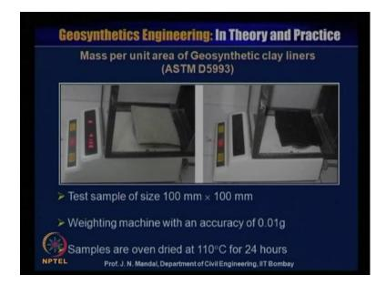
So, initially, we have to calculate what would be the mass per unit area of geosynthetics clay liner as per ASTM D5993. So, this is very simple way to determine that, mass per unit area of geosynthetics clay liner you can see, this is the sample, this is the white colour and this is the black colour, this is the test sample of size 100 millimetre by 100 millimetre. And you are putting in a weight machine with an accuracy of 0.01 g and sample are oven dried at 110 degree centigrade for 24 hour.
