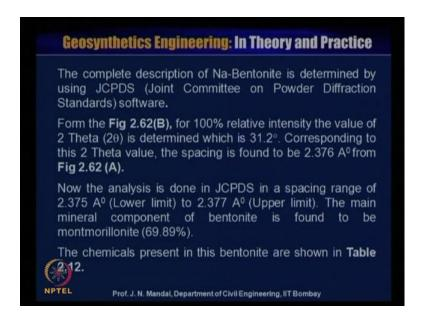
So, from this, the complete description of sodium bentonite is determined by using JCPDS, what called Joint Committee on Powder Diffraction Standards software. From this from this figure from this figure this is suppose B and also the C. So, for 100 percent relative intensity, the value of 2 theta is determined which is 31.2 degree.
