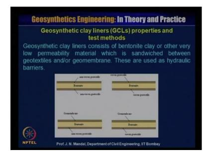
Now, we will discuss the geosynthetics clay liner that is, GCL properties and test method. Geosynthetics clay liner consists of bentonite clay or other very low permeability material, which is sandwiched between geotextile and or geomembrane, these are used as a hydraulic barrier. So, this material may be, this bentonite and sandwiched between the non-woven geotextile, non-woven geotextile, bentonite it may be bottom is woven geotextile and top is woven geotextile.
