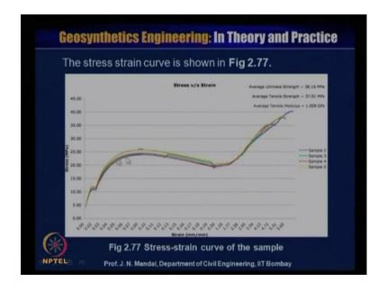
So, this is the figure so the stress strain curve of the sample you can see that, how the stress is increasing with the strain. And then it is increasing then almost constant and then decreasing then again also it is increasing.
