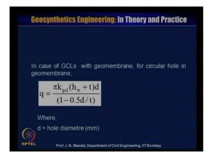
And in case of GCL with geomembrane, for circular hole in the geomembrane, if it is a circular hole so then q will be equal to pi into k gct then h W plus t into d divided by 1 minus 0.5 d by t where, d is the hole diameter so this is a circular hole. But in this case, this is the width of the slit, d and if it is a circular then this is the difference between the circular and width of the hole of the geomembrane.
