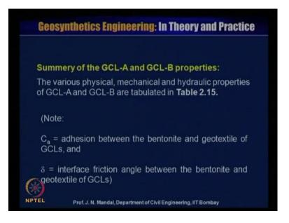
So, what summary of the GCL A and GCL B property can we conclude, the various physical, mechanical and the hydraulic property of GCL A and GCL B are shown. And where C a is the adhesion between the bentonite and the geotextile of GCL and delta is the interface friction angle between the bentonite and the geosynthetics clay liner.
