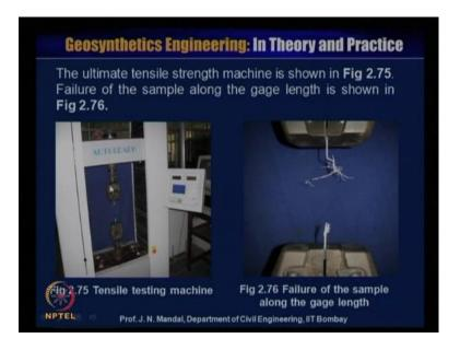
So, this is the universal testing machine and this test has been conducted and you can see that, how the failure of the sample along the gauge length. The ultimate tensile strength machine is shown, the failure of sample also along the gage length is shown.
