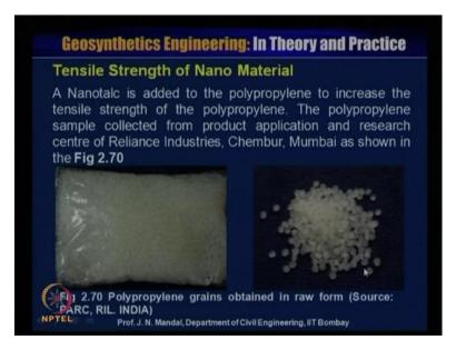
Now, this is some tensile strength of nano material, a nanotaic is added to the polypropylene to increase the tensile strength of polypropylene. The polypropylene sample collected from the product application and research centre of reliance industry, Chembur, Mumbai. This you can see, this is the sample is been collected, this is the polypropylene grain and this is obtained in raw form and this is the source for PARC, RIL, India you can see, this is the bits.
