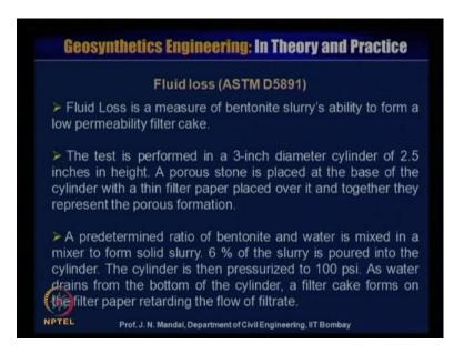
Next, fluid loss test as per ASTM D5891, fluid loss is a measure of bentonite slurry's ability to form a low permeability filter cake. The test is performed in a 3 inch diameter cylinder of 2.5 inches in height, a porous stone is placed at the base of the cylinder with a thin filter paper placed over it and together they represent the porous formation. A predetermined ratio of bentonite and water is mixed in a mixer to form solid slurry, 6 percent of the slurry is poured into the cylinder.
