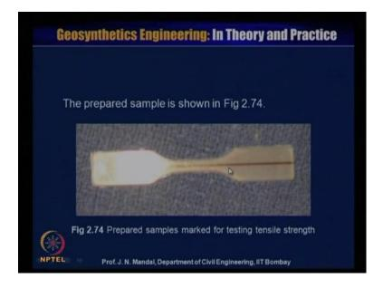
So, this is the sample and this prepares the sample is shown in this figure so this is the prepared sample for marked for testing for the tensile strength.
