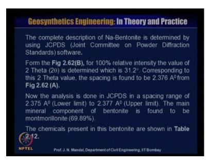
And now, the analysis is done in JCPDS in a spacing range of 2.375 Angstroms that is lower limit to 2.377 Angstrom for the upper limit. The main mineral component of bentonite is found to be montmorillonite that is about 69.89 percentage, the chemical present in this bentonite are shown.
