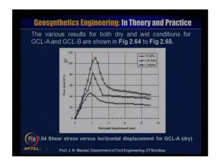
So, you have performed the shear stress versus this horizontal displacement, the various result for both the dry and the wet condition for the geosynthetic clay liner A. And geosynthetic clay liner B has been performed under the pressure of 50 kilo Pascal, 100 kilo Pascal and 150 kilo Pascal. You can see here, how the shear stress is increasing with the increasing of the hydraulic displacement.
