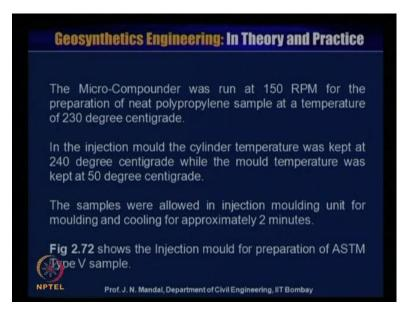
These microcomputer was run at 150 rpm for the preparation of neat polypropylene sample at a temperature of 230 degree Centigrade. In the injection mould, cylindrical temperature was kept at 240 degree Centigrade, while the mould temperature was kept at 50 degree Centigrade. The samples were allowed in injection moulding unit for moulding and cooling for approximately 2 minutes.
