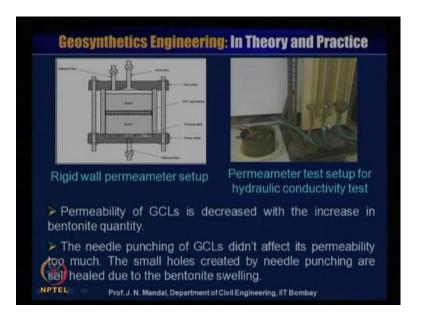
So here, the rigid wall permeameter setup here, the permeameter test setup for hydraulic conductivity test. So, permeability of the geosynthetics clay liner is decreased with the increase in the bentonite quantity, the needle punching of GCL did not affect it is permeability too much. This small holes created by the needle punching are self-healed due to the bentonite swelling.
