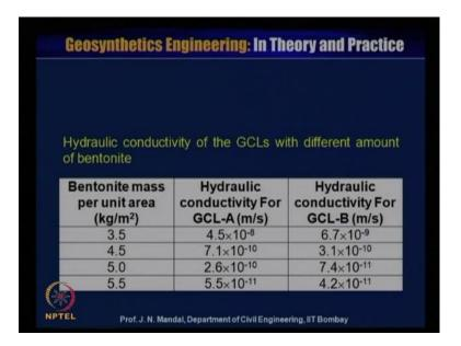
So here, showing in the table that, hydraulic conductivity of GCL with different amount of bentonite. So, bentonite mass per unit area you can see, kg per metre square that is, you have been given 3.5, 4.5, 5, 5.5 and thus, hydraulic conductivity for GCL A that is metre per second when the mass is 3.5 kg, this hydraulic conductivity 4.5 into 10 to the
