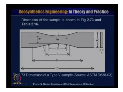
And from this, we can prepare this kind of the sample and you can perform the test, this is the dimension of the sample as various ASTM D638 so you know all these dimension or this sample.
