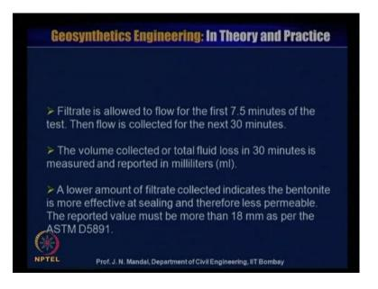
And then flow is collected for the next 30 minutes, the volume collected or the total fluid loss in 30 minutes is measured and reported in millilitre or ml. A lower amount of filter collected indicate the bentonite is more effective at sealing and therefore, less permeable. The reported value must be more than 18 millimetre as per the ASTM D5891.
