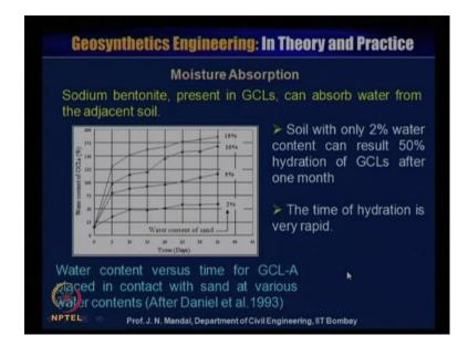
Now, some test also had performed for moisture absorptions tests now, sodium bentonite present in the geosynthetic clay liner can absorb water from the adjacent soil. Here, you can see that, water content versus the time for a geosynthetics clay liner A placed in contact with the sand at various water content. So, soil with 2 percent water content can result that, 50 percentage of hydration of the GCL after 1 month.
