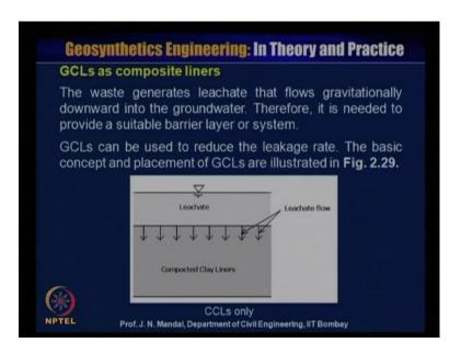
The geosynthetics clay liner as a composite liner, the waste generates a leachate that flow gravitationally downward into the groundwater. Therefore, it is needed to provide a suitable barrier layer or the system. GCL can be used to reduce the leakage rate, the basic concept and the placement of the GCL are shown in this figure. You can see, if this is the
