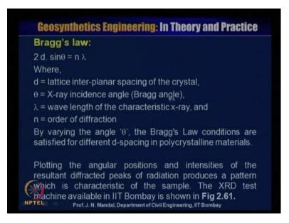
So, what is Bragg's law is 2 d sin theta is equal to n lambda where, d is lattice inner planar spacing of the crystal, theta is equal to x ray incidence angle is Bragg's angle and lambda is wavelength of the characteristics x ray and n order of diffraction. By varying the angle theta, the Bragg's law conditions are satisfied for different d spacing in polycrystalline material.
