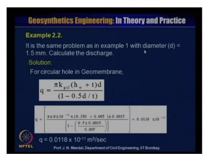
Now, in example 2, in the same problem as in the example 1 we discussed, where the diameter d is 1.5 millimetre then you calculate the distance. So, it is a circular hole in the geomembrane then equation is changing, this is the equation. So, in the same formula, if you calculate what is q, this everything is same, only that it is the d value will change so d will be the 1.5 millimetre. So, you substitute this value that is, 0.0015 and also this will be the 0.0015, other remain constant.
