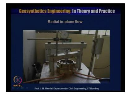
Now, this is another test for transmissivity this is call the radial in-plane flow, so you can see this equipment and this geotextile is placed somewhere here, and this there is a hole I will show you then water can just pass through radically through this; that means, along the plane of the geosynthetics material. And one side this water is in another side is water is out at a particular hydraulic gradient and this is the loading arrangement, so you have to apply the load.
