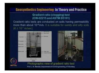
Now, gradient ratio or clogging test is U S army corps of engineers gradient ratio that is C W 02215 and A S T M D 5101, gradient ratio test are conducted on soil having permeability more than about 10 to the power minus 5 meter per second. It is suitable for sandy and silty soil for coefficient of permeability less than equal to 10 to the power minus 7 meter per second.
