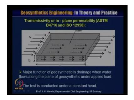
That means, this area will be this area; that means, this is the w g w g and this is the thickness t g, so this area will be w g into t g.
