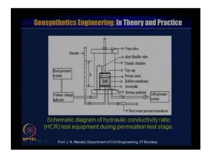
Now, here you can see that schematic diagram of hydraulic conductivity ratio test equipment during permeable test stage, here you can measure this is the soil sample this geotextile material is here this is the bottom pedestal. And this is the rubber membrane and porous stone is on the top, and then the top is the top cap, you can also from that back pressure system, so you can volume change indicator.
