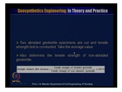
After this you take two abraded geotextile specimen are cut and tensile strength test is conducted take the average value and also you determine the tensile strength of the nonabraded geotextile material. So, strength retained after abrasion will be equal to the ratio of tensile strength of abraded geotextile and the tensile strength of non-abraded geotextile into hundred into percentage, so this way you can calculate what will be the strength retained after abrasion.
