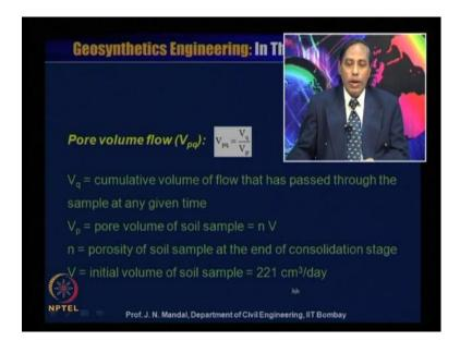
Now, pore volume flow or V p q, V p q is defined as the ratio of V q by V p, V q cumulative volume of flow that has passed through the sample at any given time and V p is the pore volume of soil sample is equal to n into V. So, n is equal to the porosity of the soil sample at the end of consolidation test and V is initial volume of the soil sample that is 221 centimeter cube per day.
