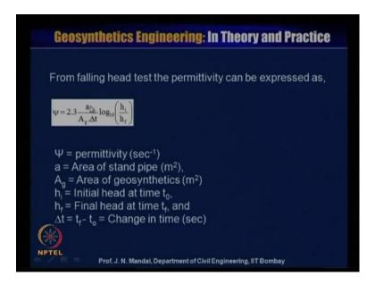
So, you know that falling head test, so this falling head permittivity test also you can determine, from the falling head test permittivity can be expressed psi is equal to 2.3 small a by A g into delta t log of h 1 by h f. And this psi which we call permittivity this
