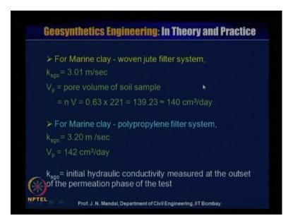
Let us say for the marine clay and woven jute geotextile filter system, so you can calculate k s g o 3.1 meter per second V p pore volume of soil sample that is n into V, and n we have calculated earlier that is n is equal to 0.63. This n is equal to 0.63 and this V is 221, this is V initial volume of the soil sample 221 centimeter cube, so V p will be equal to 0.63 into 221; that means, 139.23 this is approximately one 40 centimeter cube per day.
