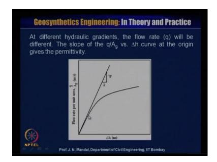
Now, you can also draw a correlation between the flow rate per unit time that is q by A g to the delta h; that means, this is q by A g to delta h, so if you can draw the relationship between the flow rate per unit area to the delta h and you can draw this tangent and this slope which will give you the value of permittivity. So, at different hydraulic gradient the flow rate q will be different, the slope of q by A g versus the delta h curve at the origin give the permittivity.
