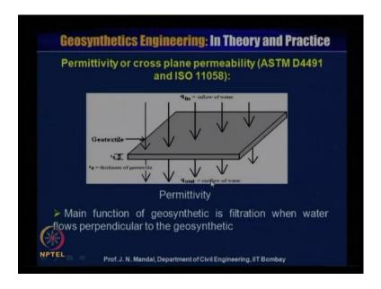
So, next we will address the permittivity or cross plain permeability as per ASTM D4491 and ISO 11058, this test is very important in hydraulic related structure. So, here you can see that this is the geosynthetics material and water flow into the geotextile material and water out from the geotextile material, so this is the flow q in and this is the flow q out and this is the thickness of the geotextile material is t g.
