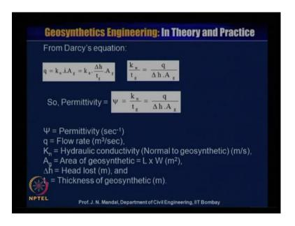
Now, that what are the theory from the Darcy's equation, we know q is equal to k into n into i into A g k n and i is delta h by t g, t g is the thickness of the geosynthetic material and delta h is equal to head lost and A g is equal to area of geosynthetics and area of geosynthetics is length into width.
