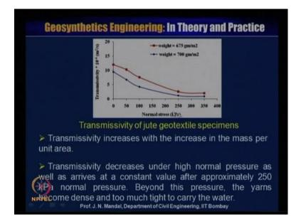
Now, as I mentioned that transmissivity of geosynthetics material are to be conducted under different normal stresses, you can see here we have performed some test under different weight and also under different normal stresses. So, this y axis is the transmissivity into 10 to the power minus 6 meter square per second, and this is all under the normal stress that is begin in the beginning, then you start with the 50 kilopascal.
