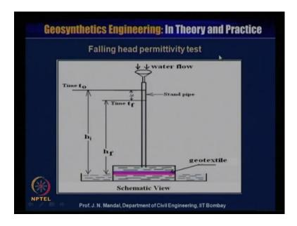
Similarly, falling head permittivity test, you can see this is the initial time t 0 and for a initial height h i this is the final time t f, and this is the final height h f and this is the stand pipe water is flowing to the stand pipe and geosynthetics material is here this red color geosynthetics material is here.
