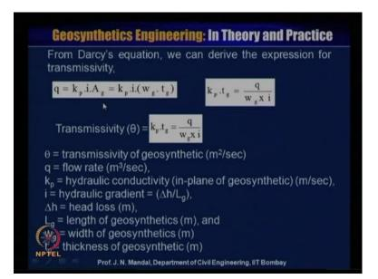
So, now again from the Darcy's equation we can derive the expression for transmissivity; that means, q is equal to k p into i into A g or k p into i into A g is the area,
