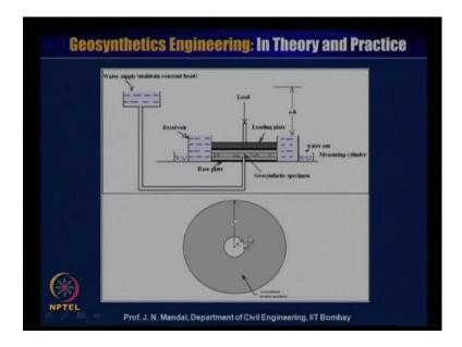
So, you can see here some schematic view, so here the geosynthetics material is placed this is the base plate, and there you can see this is the one diameter inner and this is the outer.
