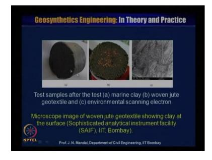
So, this is the some microscopic image of the woven jute geotextile showing clay at the interface, this is has done in sophisticated analytical instrumental facility SAIF in IIT, Bombay. And test sample after the test a is the marine clay and B is the woven jute geotextile material, and see you can see how environmental scanning electrons, so what is happening just to see their structure and their behavior.
