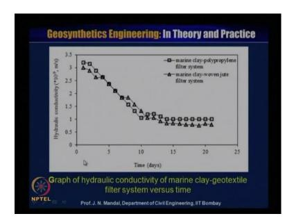
I am showing in a larger scale here, this is the graph of hydraulic conductivity here this is 100 can tend to the minus 9 meter per second and this is time days, so this is for the marine clay geotextile filter system value. There are two marine clay polypropylene filter system marine clay woven jute filter system, you can see that what will be the nature of the curve; that means, how what is happening the hydraulic conductivity with respect to the time.
