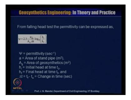
So, you can calculate this what should be the permittivity of the geosynthetics material by falling head permittivity test, so this test is very important permittivity test, similarly there is another term is very important that is transmissivity or in-plane permeability is as for A S T M D 4716 and I S O 12958.
