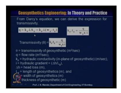
So, then k p into t g will be equal to q by w g into i, so transmissivity, which can be expressed as theta is equal to k p into t g is equal to q by w g into i, this theta is
