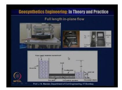
This is geosynthetics material and this is applied load I will tell you later on we are applying the load and this is geosynthetics material.
