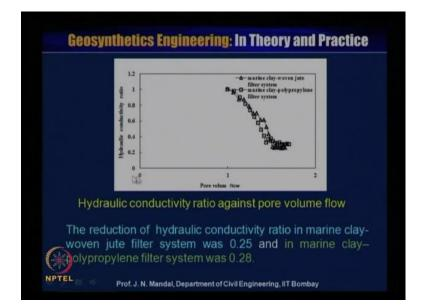
So, it depend upon that what will be the type of the material you are using, what type of the soil and after how many days it is stabilized, this figure show the relationship between the hydraulic conductivity ratio that is H C R and pore volume flow that is V p q from 0 to 2 and the hydraulic conductivity ratio from 0 to 1.2. This is hydraulic conductivity ratio against pore volume flow, so hydraulic conductivity ratio pore volume
