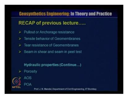
Recap of the previous lecture, we have completed pullout or anchorage resistance, tensile behavior of geomembrane, tear resistance of geomembrane, seam in shear and seam in peel test, and then we are continuing hydraulic properties that is porosity A O S Apparent Opening Size and P O A Percentage Opening.
