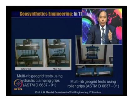
So, roller grip generally used, so you can see this is multi-rib geogrid tensile testing machine with the hydraulic clamping you can see type of the failure after test and this is the multi-rib geogrid tensile testing. This is the roller grip, this is the roller, this is the roller grip if we to perform with the very strength of the geogrid. So, we could use this roller grip.
