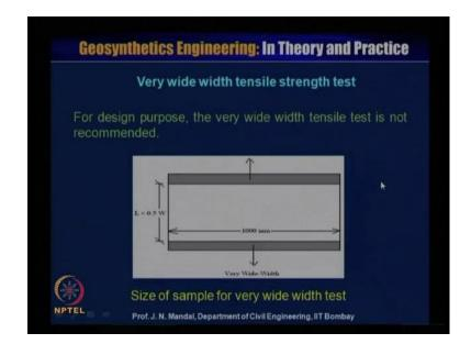
There are also other very wide width tensile strength, test for design purpose very wide width tensile test is not recommended. You can see this is the width of the sample about that  $1\ 0\ 0\ 0$  millimeter and this is about 0.5 times of W. So, this test is not recommended.
