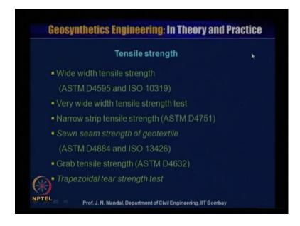
Tensile strength, there are various type of the tensile strength, that is wide width tensile strength, that is ASTM D4595 and ISO10319, very wide width tensile strength test, narrow strip tensile strength ASTM D4751, sewn seam strength of geotextile ASTM D4884 and ISO 13426, grab tensile strength ASTM D4632, trapezoidal tear strength test.
