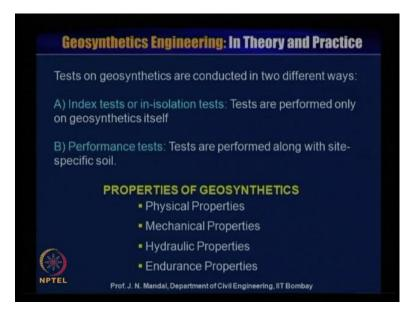
Test on geosynthetics are conducted in two different ways: a) index test or in-isolation test, test are performed only on geosynthetics material itself and b) performance test. Tests are performed along with site specific soil. Now, we will discuss the properties of geosynthetics, their physical properties, mechanical properties, hydraulics property and endurance property.
