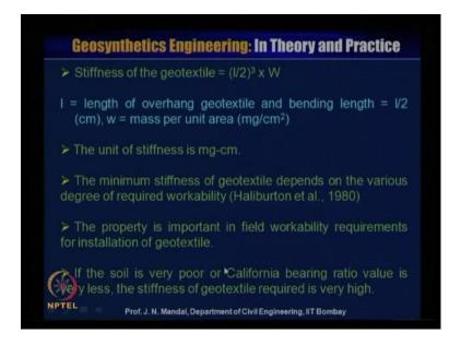
Then you can measure what will be the stiffness of the geotextile. Stiffness of the geotextile l by 2 whole to the cube into w, where this l is equal to length of over hang geotextile and the bending length is l by 2 and this expressed is centimeter and w is the
