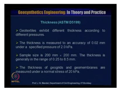
Next property is thickness ASTM D5199: Geotextile exhibit different thickness according to the different pressure. The thickness is measured to an accuracy of 0.02 millimeter under a specified pressure of 2 kilopascal and sample size is 200 millimeter into 200 millimeter. The thickness is generally in the range of 0.25 to 8.5millimeter. The thickness of geogrid and geomembranes are measured under a normal stress of 20 kilopascal.
