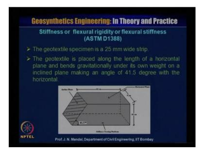
Now, the stiffness of flexural rigidity or flexural stiffness as per ASTMD 1388. So, geotextile specimen is 25 millimeter wide strip, geotextile is placed along the length, along the length of a horizontal plane and bends gravitationally under its own weigh ton a inclined plane making at an angle of 41.5 degree with the horizontal.
