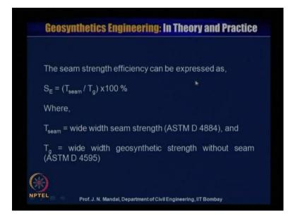
So, seam strength efficiency can be expressed as SE is equal to T of seam divided by T g into 100 percentage, where T of seam in wide width seam strength as far ASTM D4884.
