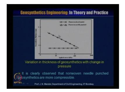
You can see this figure, that is related between the geotextile thickness in millimeter and this is the applied pressure in kilopascal. You can see, there are the two types of the geosynthetics material, how the variation in thickness of geosynthetics with change in the pressure this is its nonwoven heat bonded material and this is nonwoven needle punched material. You can see, this is non woven needle punched material and this is nonwoven heat bonded material.
