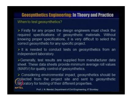
Without knowing proper specification, it is very difficult to select the correct geosynthetics for any specific project. It is needed to conduct test on geosynthetic from an independent laboratory. Generally, test result is supplied from manufacturer data sheet. These data sheet provide minimum average roll values that is MARV for quality
