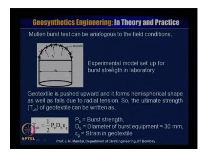
Now, Mullen burst test can be analog to the field condition, so this is the experimental model set up for burst strength in the laboratory and this is the D b, which call the diameter of the burst equipment and this equal to about 30 millimeter and this is the gravitational material clamp and there is a upward force, that is P v, this is, this is what we call the burst strength.
