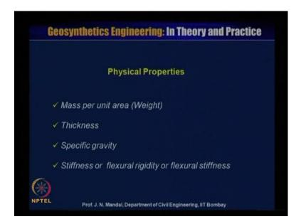
So, we will discuss the different properties of the geosynthetics material. It may be woven geosynthetics material, non woven geosynthetics material, it may be geogrid, it may be geomembrane, it may be geosynthetic clay liner, it may be geo cell and we will teach you about their different properties.
