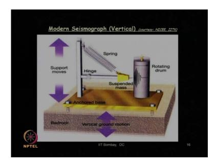
So, let us look at this picture. This shows modern seismograph in the vertical direction, that is, again we have a bedrock slab, on top of this we have an anchored base plate and a support system connected like this. Through a spring there is a suspended mass, you can see over here, and on tip of this mass there is a pen or pencil and this drum, again, is surrounded by white papers and this drum can, of course, rotate.
