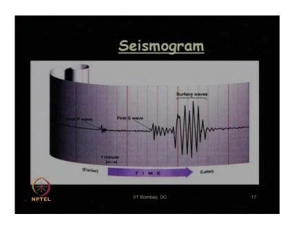
Now, as we have mentioned, instrument is called seismograph and the recorded data, we call it as seismogram. So, let us see how the seismogram will look like. So, this is the typical output of the seismogram, that is, what is getting recorded on that piece of paper through that rotating drum. We get, finally, that paper out from the drum and when we take a note of these excitations, which are getting recorded due to a particular earthquake; it will be something like this.
