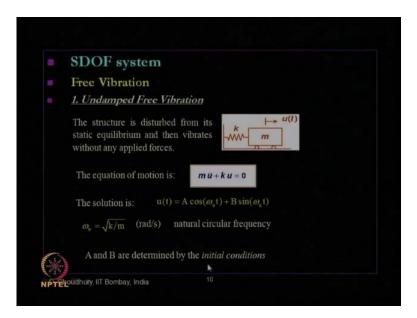
Then, we have seen the solution for simplest case of free vibration with undamped condition. That means the equation of motion boils down to m u double dot plus k u equals to 0. We should know the initial condition that is at time t equals to 0. What is the displacement? What is the velocity for this free vibration to get the complete solution? The solution of this equation will be of this form, where these constants, a and b need to
