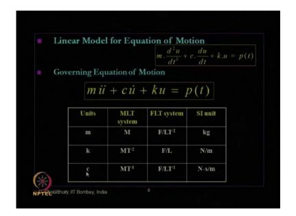
So, using that if we consider a linear model for the equation of motion, we have seen that mass times acceleration is the inertial force damping. Constant times velocity is the damper force and spring constant time displacement is the spring force which will be equal to this externally applied dynamic load p of t. This is why for linear model because the assumption is masses not changing with time
