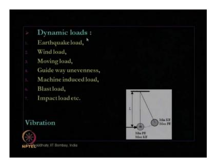
So, what we learned in the previous lecture in this module 2 that various types of dynamic loads what is called dynamic loads, it has to be time variant load as well as it should create a vibration that is the exchange of kinetic energy to potential energy and vice versa. So, these are various types of dynamic loads and of course, our earthquake load for which we are studying this course is one of the major forms of dynamic load.
