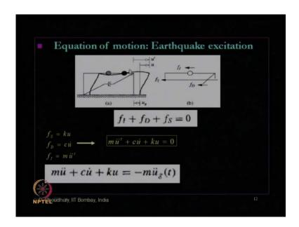
So, this is the basic model where inertial force damper force and spring force equals to 0 where inertial force act's on the total displacement, because the acceleration acts on this mass for the total displacement, but damper and spring force acts further relative displacement compare to this ground and total displacement difference between that will give us the relative displacement.
