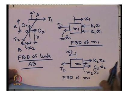
So, the link which is shown over here that AB link, AB we are drawing the free body diagram. So, this is moving by x 2, this is moving by x 1. So, this distance is x 2, this distance is x 1 and corresponding forces are let us say, this is T 1, let us say this is T 2.
