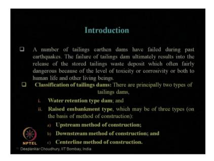
Now, let us come to another sub topic, which is seismic stability of tailing dam. Now what is tailing dam or earthen dam, let us first introduce. A number of tailings earthen dam have failed during the past earthquake. The failure of tailing dam, ultimately results
