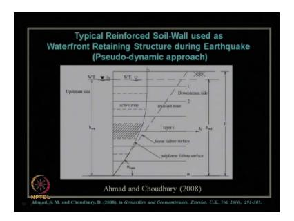
We studied the seismic design of waterfront reinforced soil wall; that the analysis of reinforce soil wall in the water front, by using Pseudo-dynamic approach, both in terms of internal stability as well as external stability. The internal stability this is the paper, by Ahmad and Choudhury, appeared in journal Geo-textile and Geo-membranes Elsevier publication 2008.
