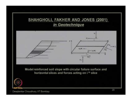
Then Shahgholi Fakher and Jones in 2001, they also use the horizontal slice method for slope stability analysis for a reinforced soil slope. So, for reinforced soil slope, this paper is available again in the journal Geo-technique, published by IC London. This is the basic force diagram on an infinite simal soil mass, which contains only one
