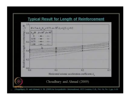
We found out how much reinforcement length is required, in terms of overturning mode of failure, in terms of sliding mode of failure. And then among these three length; that is one is pullout of the reinforcement, another is sliding, another is over turning. Based on all these three, you have to provide the maximum length of the reinforcement, for stability of such reinforce soil wall in the waterfront. Then in our previous lecture, we also discussed about seismic design of shallow footings.
