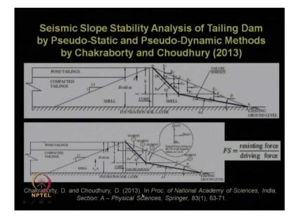
This is the downstream side failure surface are considered, based on the frenetic line etcetera, and factor of safety can been calculated like this as we know. In this case, the upper figure shows the all the forces, including the seismic inertia force in vertical and, in horizontal and vertical directions, considering pseudo-static approach. And this one shows the same problem, but these inertia forces are considered or calculated using Pseudo-dynamic approach.
