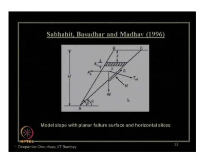
Other researchers like, Sabhahit, Basudhar and Madhav in 1996 proposed this horizontal slice method, for slope stability analysis. And this is the additional horizontal force of p h, which is acting along with other static forces.
