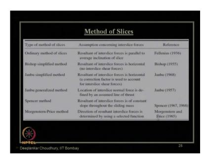
Like method of slices, we know these are the various methods of slices which are used in static case of slope stability analysis, and their references also are given over here.
