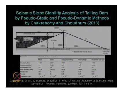
Now, next one comes, the seismic slope stability analysis, using pseudo-static and pseudo-dynamic method, because initially we have done using FLAC method and TALREN method software. Now we are using the analytical method, to check whether
