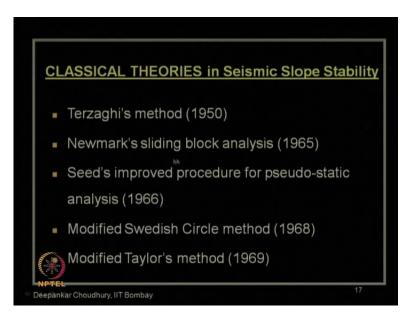
We discussed first about the classical theories in seismic soil slope stability analysis, using conventional pseudo-static approach, which was started with Tarzagi's approach in 1950, then followed by Newmark's sliding block method 1965 and so on.
