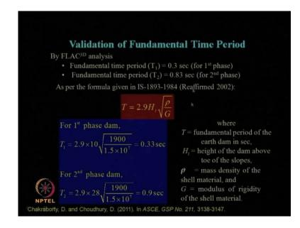
Next, we need to calculate, or validate the fundamental time period of the entire structure, how we do that. In the FLAC 3D analysis, we automatically get the
