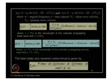
What we can see? The similar approach has been adopted. In this case, it is the active state. So, the seismic inertia force in both horizontal and vertical direction is obtained in the similar manner. But, when you are doing the equilibrium and finding out the P a e, you have to do the proper analysis of all the forces involved and their corresponding directions, etcetera to get the design value of this. And, once you get the expression for P a e, next step is to do the optimization once again.
