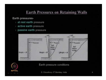
We have mentioned that, what are the various states of earth pressures acting on the retaining wall based on the movement of the wall.
