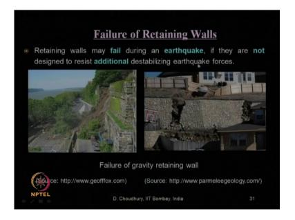
Now, failure of retaining wall; there are several cases worldwide that during the earthquake, retaining walls fail due to the additional destabilizing earthquake forces. So in what way, this earthquake forces induce the additional forces on this retaining wall, for which probably it was not designed or analyzed; that is why there were several damages as you can see from some of these pictures.
