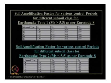
Also, if we look at what are the recommendations for the soil amplification factor for various control periods for different sub soil class; what are the different sub soil class? Already we have mentioned like A, B, C, D, and E. These five are major sub class and then S 1 and S 2 are other two different sub class.
