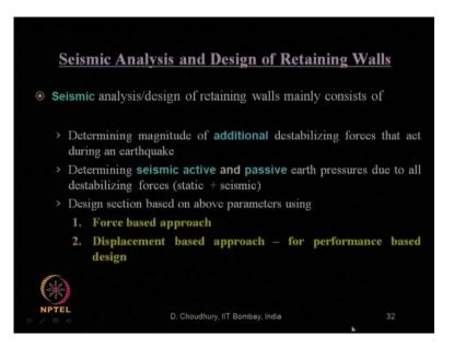
So, when we are talking about seismic analysis and design of this retaining walls, it mainly consist of determining the magnitude of that additional destabilizing force; that
