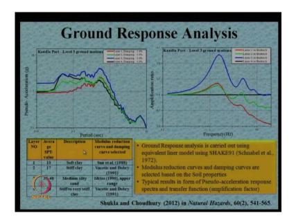
And, the ground response analysis was carried out to obtain the pseudo acceleration versus period, considering different modulus reduction curve and the damping curve as proposed by various researchers for different types of soil using shake software.
