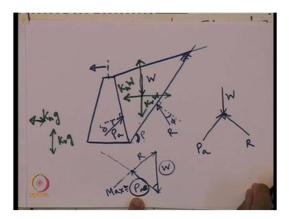
So if I show here, how the couloumbic earth pressure; let us say for active state of earth pressure, this is the rigid retaining wall. And, we are mentioning that this wall is moving towards this side. So, this is an active state of earth pressure. As coulomb's theory says,
