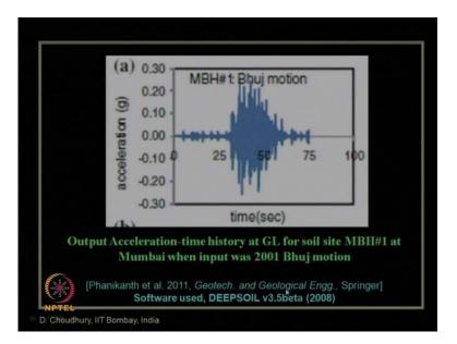
With those input motion after carrying out the equivalent-linear ground response analysis, the output what was obtained is for each borehole location. For a particular input earthquake motion, we can get the output at different levels of soil layer. So, this is at ground level or ground surface. This is the output that is, how the acceleration time response will be when a Bhuj motion is given as input bed rock motion.
