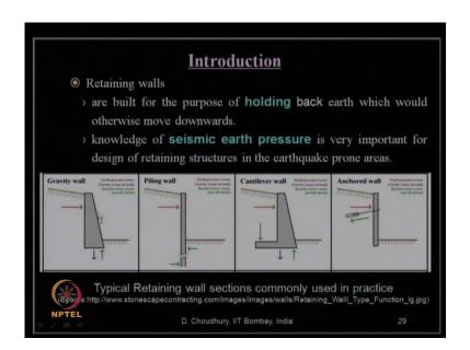
When we talk about seismic design of retaining wall, first let me introduce. As we all know, there are different type of retaining wall like gravity type, piling wall, cantilever type of wall, anchor sheet pile wall. These are different types of retaining wall.
