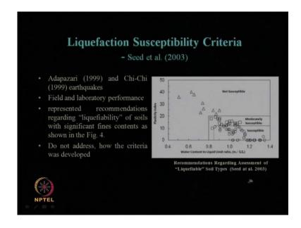
Seed et all in 2003, they proposed the recommendations for fine grained soil. That is, plasticity index versus water content to liquid limit ratio in the x-axis. They have divided into different three zones, that is susceptible to liquefaction, moderately susceptible and non susceptible. So, accordingly if somebody wants to put their soil in this region and try to find out whether it is coming in susceptible range or non-susceptible range, this recommendation may be used.
