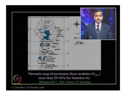
This GIS based map shows the value of maximum shear modulus, G max value, where it is more than 20 MPa for Mumbai city. How it is obtained? From the values of V s, the G max value can be easily computed by knowing the density of the soil. So through that, the G max of more than 20 MPa, those locations are marked over here. That means, these are relatively stiffer soil zone.
