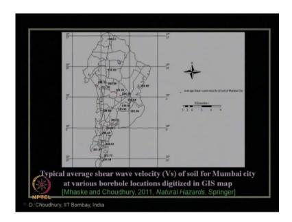
So now, let us look here that when we want to develop some particular relationship of that SPT N value versus the shear wave velocity V s for Mumbai region from the collected borehole data, you can see that these are the typical average shear wave values all around Mumbai city at various borehole locations, which are digitized in the GIS map. These details are available in this paper.
