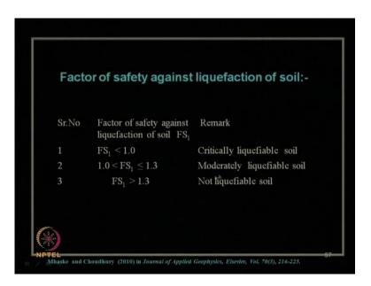
So, CRR by CSR will give the factor of safety with respect liquefaction. Using this concept, this paper of Mhaske and Choudhury in journal of Applied Geophysics, Elsevier, classified the 3 ranges of factor of safety with respect to liquefaction. That is, their value to identify or remark their soil as critically liquefiable, moderately liquefiable, and non-liquefiable soil.
