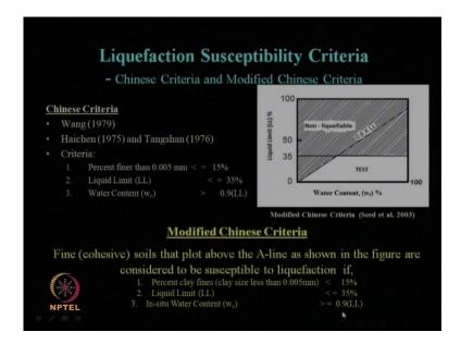
Now, let us see Chinese Criteria and Modified Chinese Criteria. Chinese Criteria was developed by Wang in 1979 based on the study by Haichen and Tangshan in 1975 and 1976. The criteria says that, the percent finer than 0.005 mm should be less than 15 percent, liquid limit should be less than equal to 35 percent and water content should be greater than 0.9 times of liquid limit for that fine grained soil. This criterion is basically for fine grained soil.
