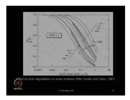
The variation of this G by G max with respect to cyclic shear strain for different values of plasticity index was reported by Vucetic and Dobryin in 1991, which shows like this type of variation and also with respect to the number of cycles. That is, if number of cycle increases, then there will be a change in the G by G max value. Obviously, it is going to decrease as it can be seen from here.
