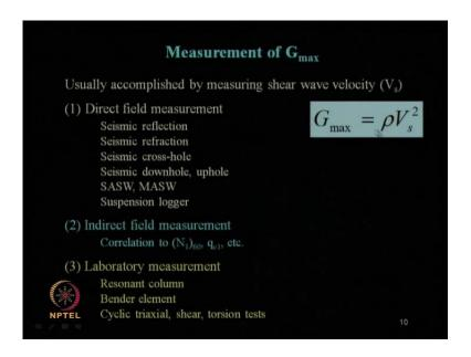
Now, how to find out this G max value or maximum value of shear modulus? The measurement involves basically three major methods. One is direct field measurement by using these techniques or indirect field measurement by using this technique or laboratory measurement using these techniques. Also from the shear wave velocity value, that is V s value, we can calculate the value of G max using this relationship, using this density of the material or density of the soil as rho.
