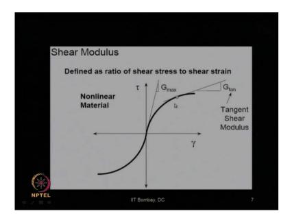
If we draw a tangent at that curvilinear portion of that material behavior, the slope of that line will give us the tangent shear modulus.
