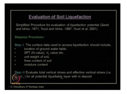
How is the evaluation of soil liquefaction carried out? From the entire set of borehole data collected for the entire Mumbai region as the dynamic soil properties, the V s value has been estimated and reported just few slides back. We have discussed here. Then for each borehole location, the soil liquefaction susceptibilities are estimated using the simplified procedure for evaluation of liquefaction potential.
