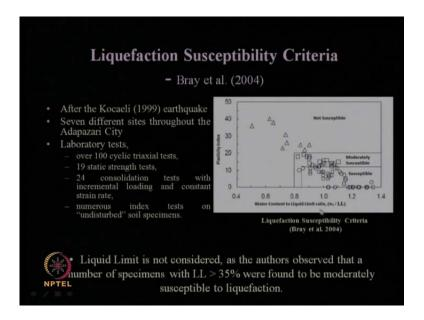
Further, Bray et al in 2004 proposed another methodology using the similar concept of plasticity index versus water content to liquid limit ratio like this. It is mentioned that liquid limit is not considered as the authors observed that a number of specimens with liquid limit greater than 35 percent were found to be moderately susceptible to liquefaction.
