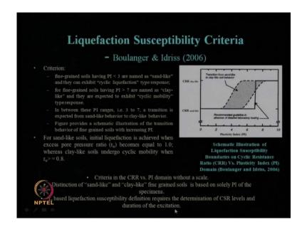
Another criteria is mentioned by Boulanger and Idriss in 2006, where CRR of clay like material and CRR of sand like material has been considered as two boundaries with respect to the x axis plot of plasticity index PI. So, different values of plasticity index, the typical range from transition of sand like to clay like soil behavior is mentioned by these researchers, which is showing the exhibit of cyclic liquefaction.
