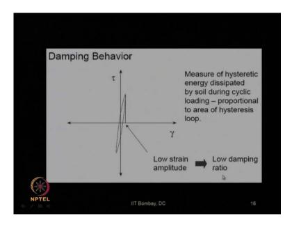
Another important parameter damping behavior, which we have discussed in our previous lecture like, at low strain, we will expect low damping ratio, whereas at high strain, we will get high damping ratio value.
