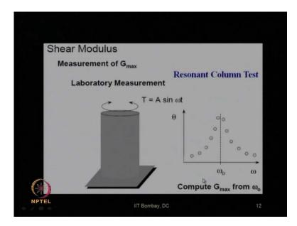
Also in the laboratory, one can find out using resonant column test like this. That is, what is the value of G max at the resonant frequency from this plot of the distortion at different frequency on the resonant column with the torque applied on it. Also from cyclic triaxial test, one can find out the G max value.
