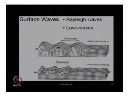
For Surface wave like Rayleigh wave and Love wave, we have seen that these are the behavior. Picture a is for Rayleigh wave and picture b is for love wave. This type of rotary motion that you can see over here for this surface wave, this is the undisturbed media and this is the disturbed media when waves are passing through. So, this also creates particle movement and particle movement is in this fashion compared to the direction of the propagation of the wave.
