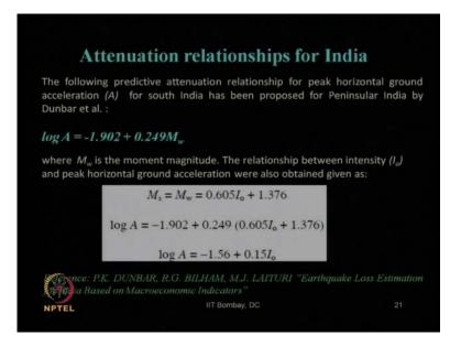
Now, let us come to another attenuation relationship of India which was proposed by Dunbar et al. Dunbar et al this earthquake loss estimation for India based on macroeconomic indicators, they proposed this equation of attenuation relationship for peak horizontal ground acceleration A for the south India.
