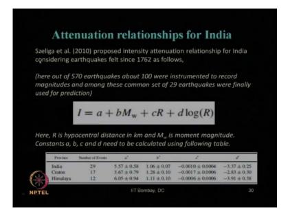
Other equation like Szeliga et al had proposed the in two thousand ten this is the intensity based equation. Once again consider the earthquake felt attenuation relationship since seventeen sixty two, seventeen hundred and sixty two to two thousand nine they have taken, but as I said the older earthquake only the intensity scale will be available.
