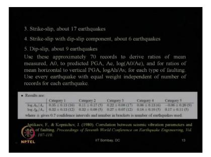
So, these are the relationship proposed for five different categories of faulting like strike slip, strike slip with dip slip, dip slip fault, etcetera, etcetera. All are detailed here, total 70 records they had used and these are the values of log of a naught by A e and log of A
