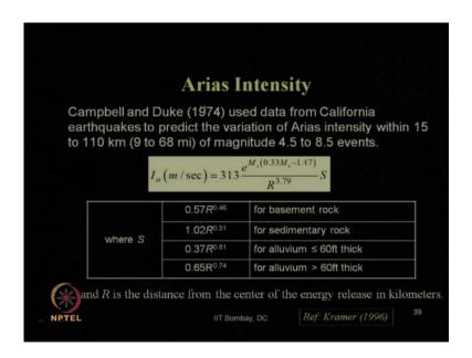
Further to estimate the arias intensity empirically Campbell and Duke in 1974 using the Californian earth quake data between the distance of 15 to 110 kilometer and between the magnitude range of 4.5 to 8.5 scale, they proposed using those historical data points. This is the empirical relation to estimate the arias intensity I a in the unit of meter per second, using this relation 3 1 3 e to the power M s times 0.33 M s minus 1.47 divided by R to the power 3.99 times S.
