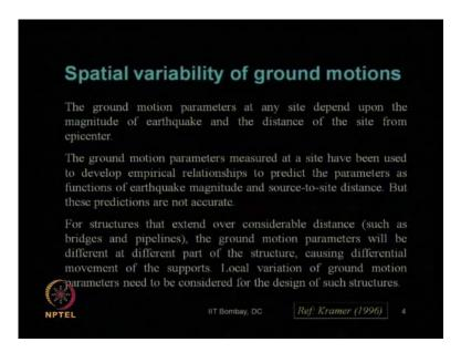
We have discussed about the spatial variability of ground motions, that is how this ground motion vary from the hypo center point of earthquake or the epicentral location to a particular distance or a site, where we are planning any new construction or any new structure to be constructed. So, the ground motion parameters they vary in terms of magnitude, and in terms of distance for a site from the epicentral location.
