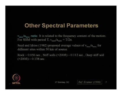
Then we had also mentioned about the others under the umbrella of other spectral parameters, the importancy of parameter like v max by a max ratio. So, that v max by a max ratio we have also related it through the derivation in the previous lecture, that how this for a simple harmonic motion, if it is applied to a single degree of freedom system with period T.
