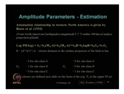
So, let us see now the equation or a attenuation relationship, which is proposed by that Boore et al 1993 for the California region earthquake. So, let us look at here in the slide, attenuation relationship in Western North America, which is given by Boore et al 1993. So, this was mentioned as latest as for as this book of Kramer is concerned which was published first in 1996.
