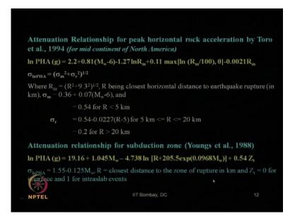
Now, let us come to the next attenuation relationship for peak horizontal rock acceleration, which was proposed by this attenuation relationship for peak horizontal rock acceleration by Toro et al in 1994, that is after Boore et al. So, this Toro et al they proposed for mid content of North America, mid content of North America means
